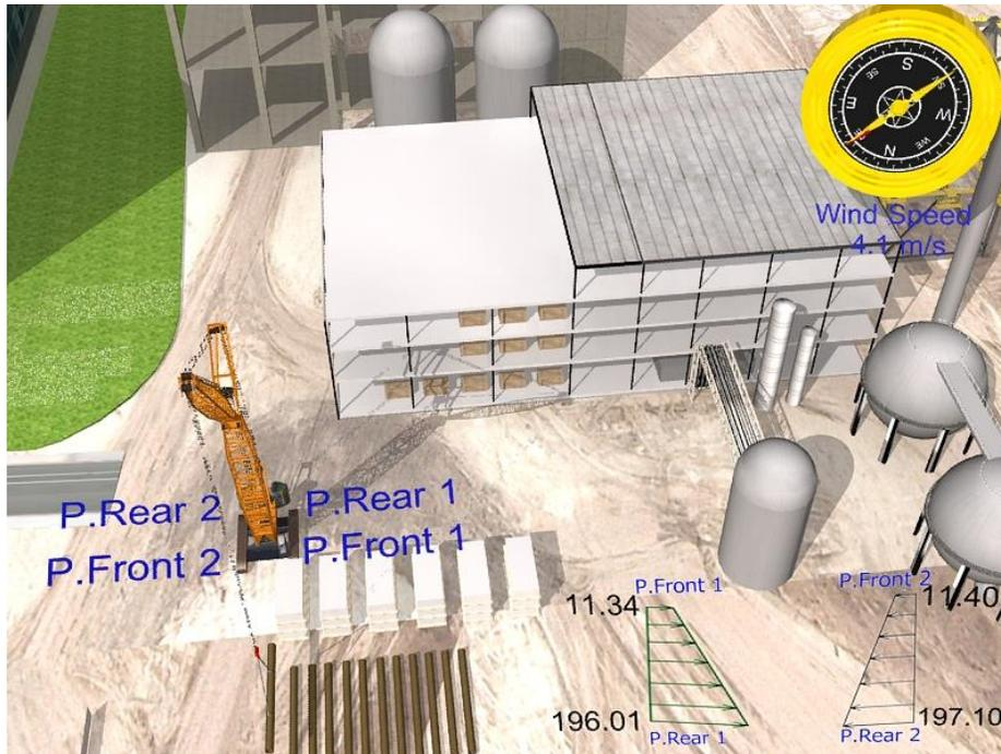
Figure 3.61: BIM-supported visualization model for crawler crane operations
