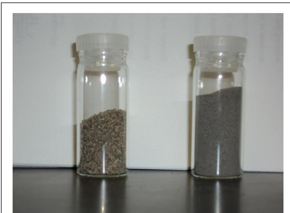
**Figure 3.4** Catalyst samples; Pt-Pd and Pt catalyst(left to right)
