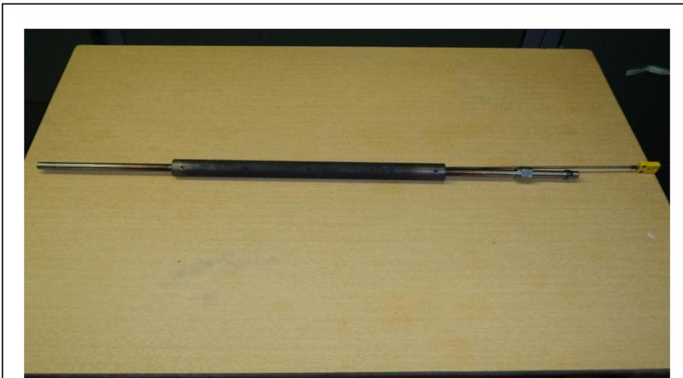
**Figure 3.3** Photo of micro-reactor
