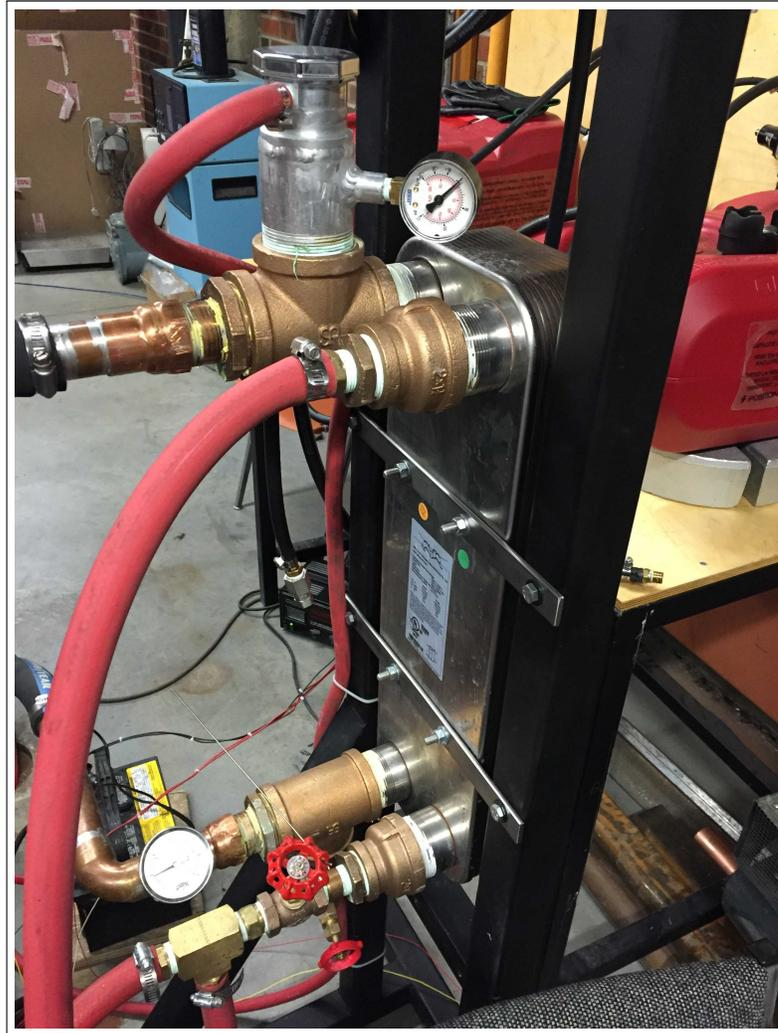
Figure 3.9: Flat Plate Heat Exchanger and Pressure Relief Valve.
