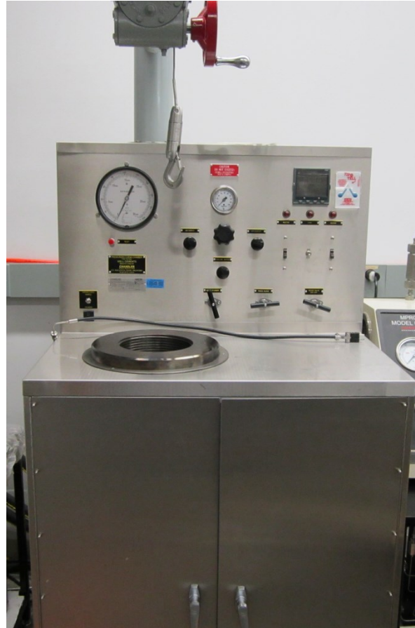
Figure A3. Pressurized curing chamber
