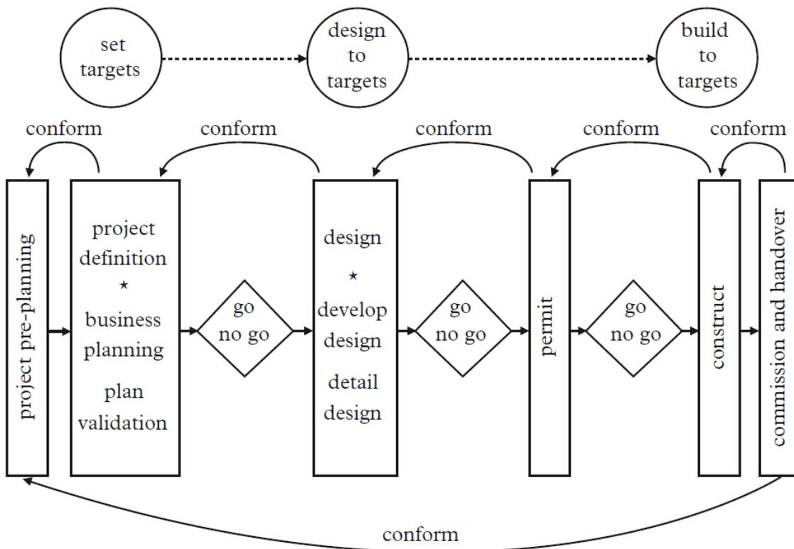
Figure 2.6: Target value design process (Daria Zimina et al., 2012)
