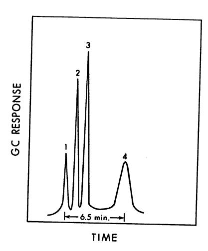
Figure A-3. Standard curve for ethylene estimation. The gas was analysed by gas chromatography and was resolved by a activated alumina column (with 2-1/2% silicone 550). The column temperature was room temperature and the detector temperature was 125°.
