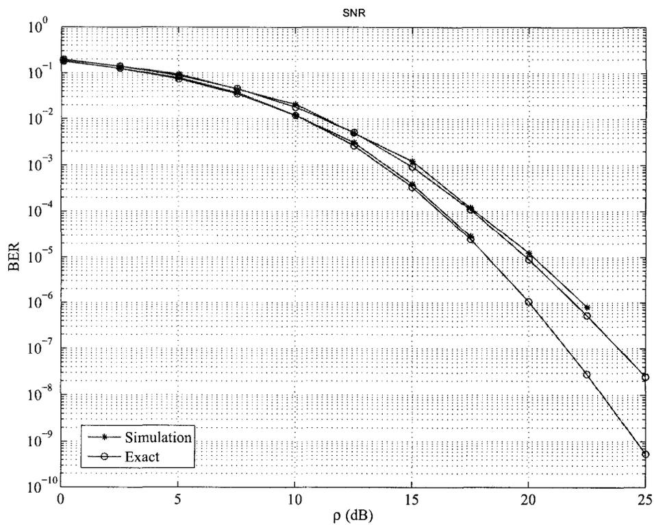
Figure 5.2: Comparison between the exact expression, approximation and simulation for  $N = 2$  transmit antenna selection out of  $L_t = 3, 4$  with  $L_r = 2$  correlated receive antennas, 16-QAM.
