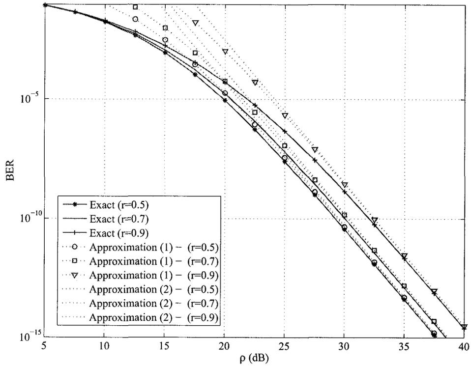
Figure 5.4: Comparison between different correlation parameter  $r$  for  $N = 2$  transmit antenna selection out of  $L_t = 3$  with  $L_r = 2$  correlated receive antennas and two approximation of performance, using 16-QAM constellations
