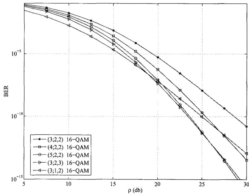
Figure 4.5: Exact BER derived in (5.45) for  $(L_t; N, L_r)$  transmit antenna selection systems, using 16-QAM
