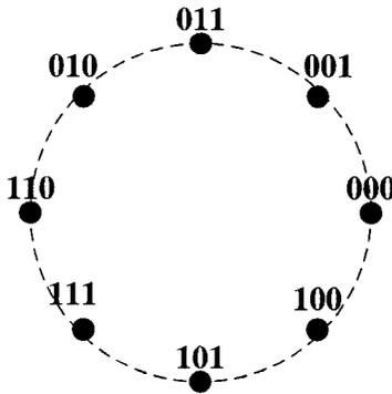
Figure 2.5: 8-PSK signal constellation with Gray Mapping.
