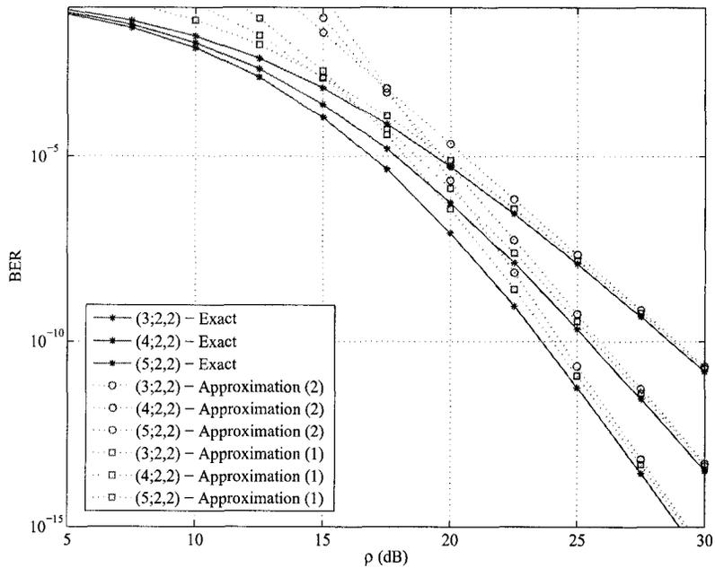
Figure 4.4: Comparison between exact BER for  $(L_t, N; L_r)$  systems, selecting optimal  $N$  transmit antennas out of  $L_t$  with  $L_r$  antennas in receiver, using 16-QAM and approximations derived in (4.32) and (4.35) and diversity and coding gain approximated BER in (4.35).
