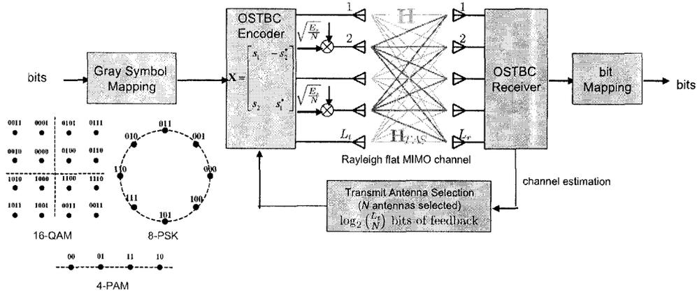
Figure 4.1: MIMO OSTBC with transmit antenna selection.
