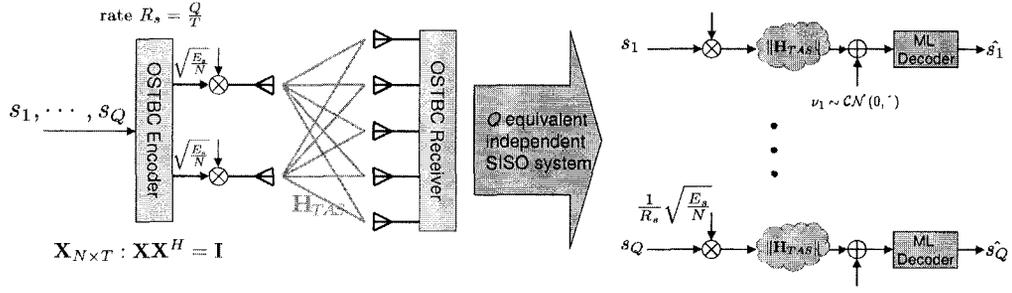
Figure 4.2: OSTBC MIMO system is equivalent to  $Q$  independent SISO systems
