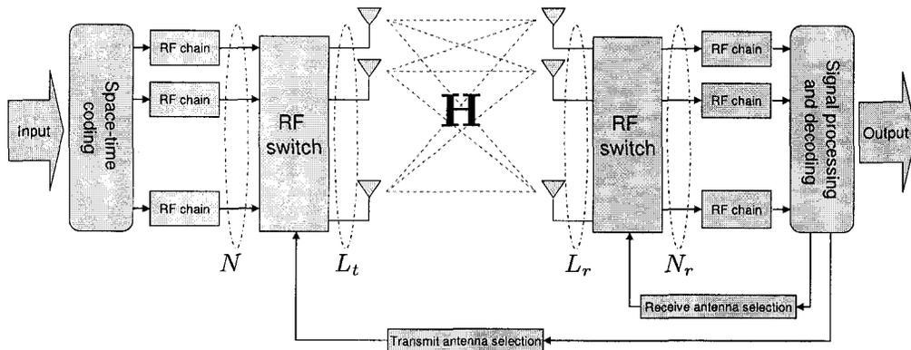
Figure 3.1: MIMO antenna selection system
