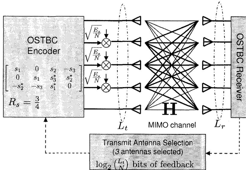
Figure 4.3: MIMO system using OSTBC of rate 3/4 and 3 transmit antenna selected
