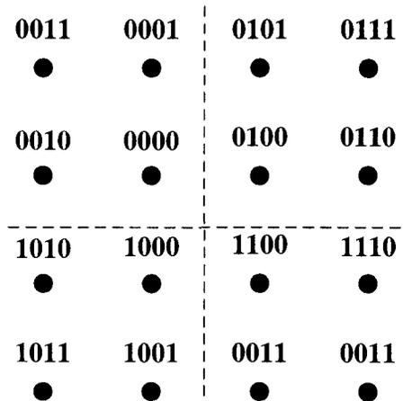
Figure 2.4: 16-QAM signal constellation Gray Mapping.
