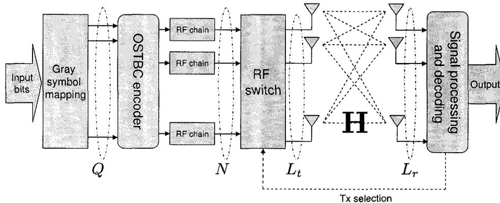
Figure 3.2: Transmit antenna selection scheme
