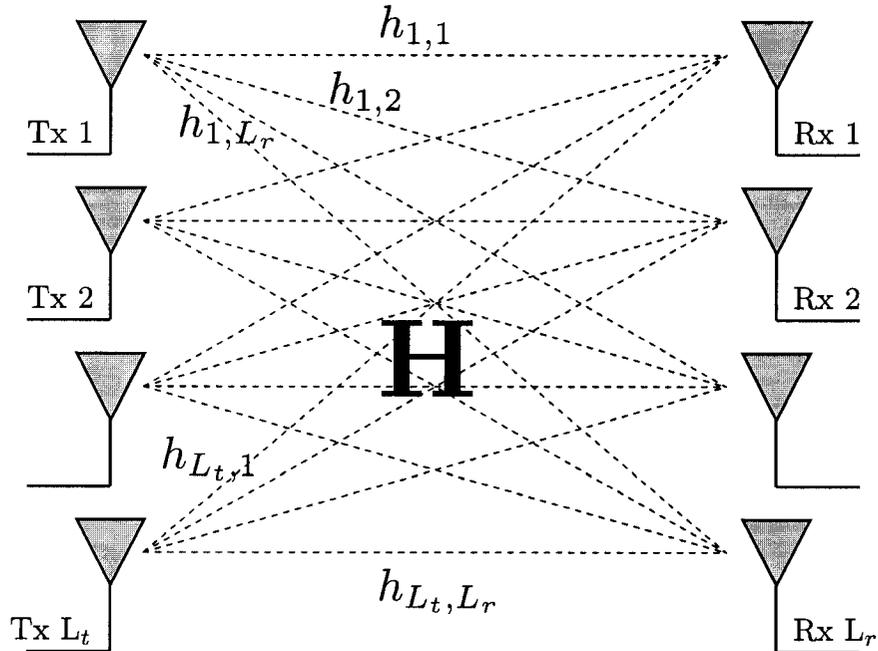
Figure 2.1: MIMO Channel Model
