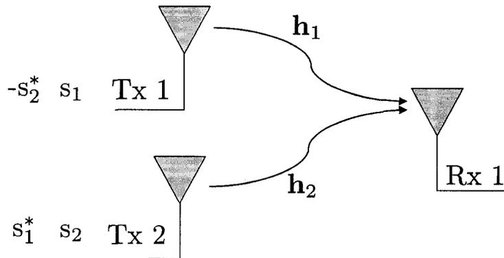
Figure 2.7: Alamouti Scheme with 2 transmit antenna and 1 receive antenna
