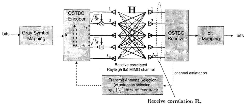
Figure 5.1: MIMO system using OSTBC over Transmit antenna selection in Rayleigh flat fading channel with receive correlation  $\mathbf{R}_r$
