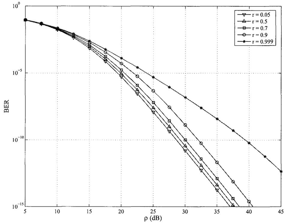
Figure 5.3: Comparison of the performance between different correlation parameter  $r$  for  $N = 2$  transmit antenna selection out of  $L_t = 3$  with  $L_r = 2$  correlated receive antennas, 16-QAM.
