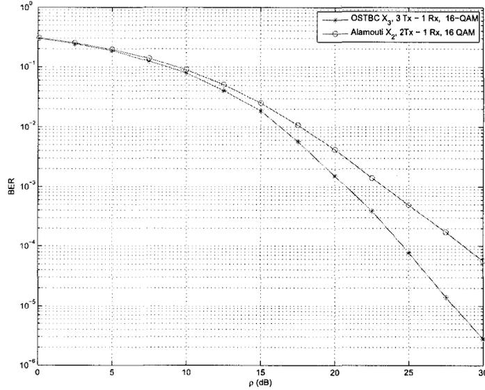
Figure 2.8: BER performance of OSTBCs using 16-QAM.
