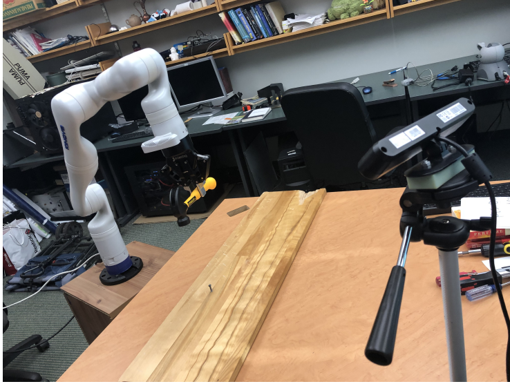
Figure 7.5: Experimental setup of the hammering task.
