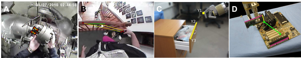
Figure 1.4: Examples of using geometric constraints to specify tasks, A and B are human task examples while C and D are robotic task examples. A: a tool insertion tasks [14] which is specified by two point coincidences. B: a wiping stairs handle task [14] which is specified by a point-to-line and point-to-point constraint. The point-to-line constraint means a point on the cloth stays contact with the stair handle. The point-to-point constraint means a point on the cloth should approach a point to the far end of the stair handle. C: an open drawer task [48] which is specified by a point-to-line constraint. D: a circuit board RAM insertion task [48] which is specified by a line-to-line alignment constraint and a point-to-point constraint.
