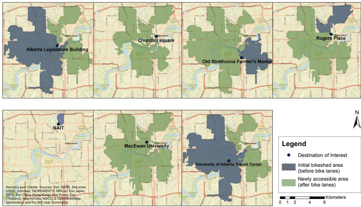
Figure 3 Bikeshed area for each destination before and after protected bike network construction.
