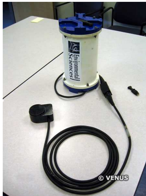
Figure 1.1: The ZAP transducer and pressure case [2]
