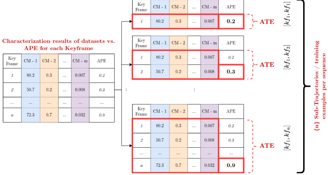
Figure 5.2: Extraction of training examples based on sub-trajectories and corresponding SLAM errors (APE and ATE)
