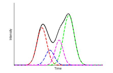
Fig. 5. Deconvolution of overlapping peaks. The black, solid trace represents the analytical signal observed at the detector, which is the sum of the four peaks represented by dashed lines.
