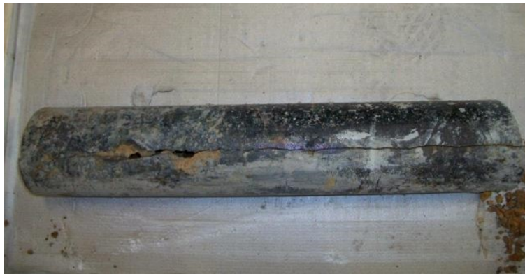
(a) Axial crack
