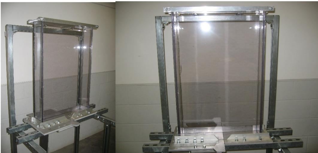
Figure 3-2 Granular flow apparatus (85 cm height  $\times$  50 cm width  $\times$  10 cm depth)
