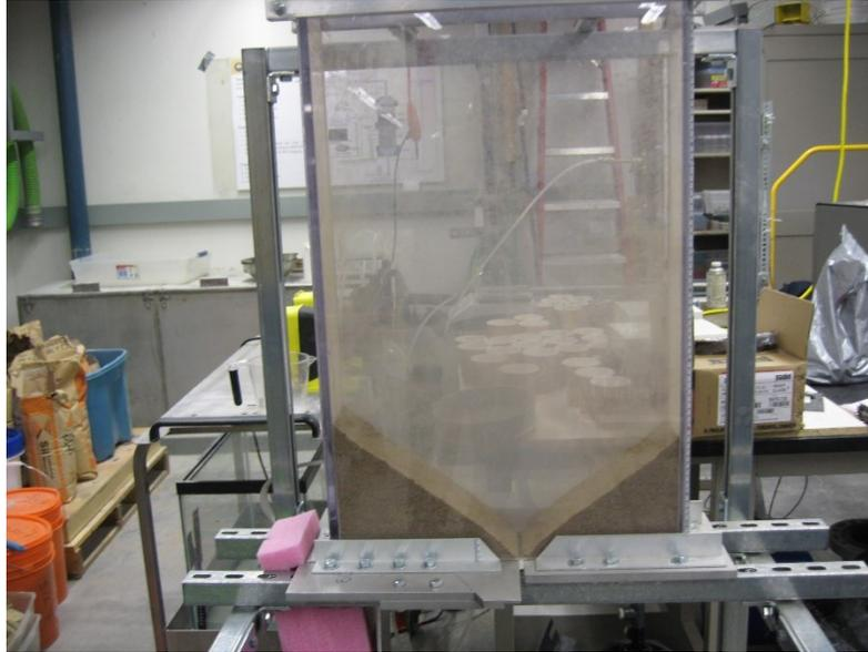
Figure 3-5: Stagnant zones after sand flow was completed.
