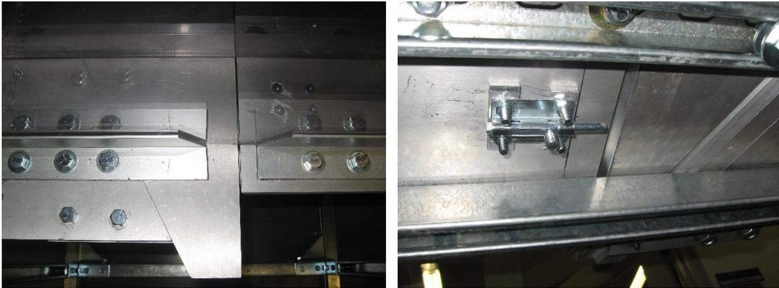
Figure 3-3 Right triangle plate for adjusting slot width (left) and control gate with lock below the slot (right)
