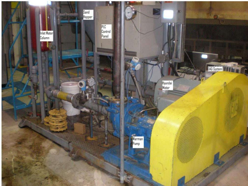
**Figure 27. Photo of Syncrude research slurry loop main components**
