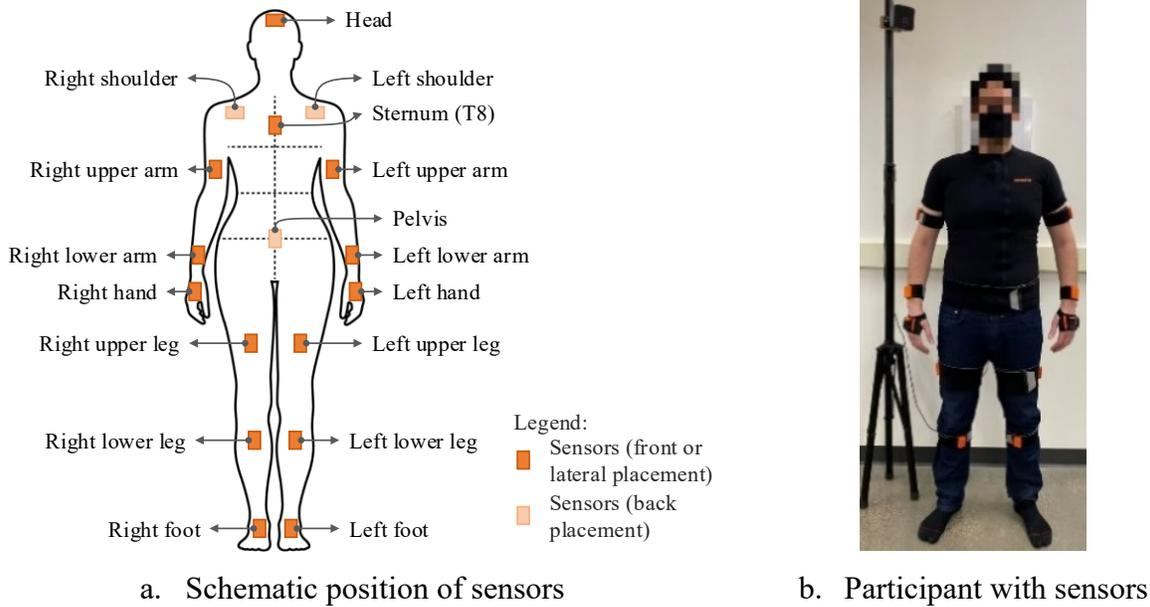
**Figure 5.3: IMUs used to capture body motion information.**
