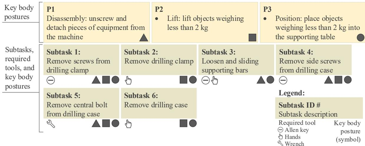
**Figure 4.4: Description of subtasks, required interactions, and key body postures.**
