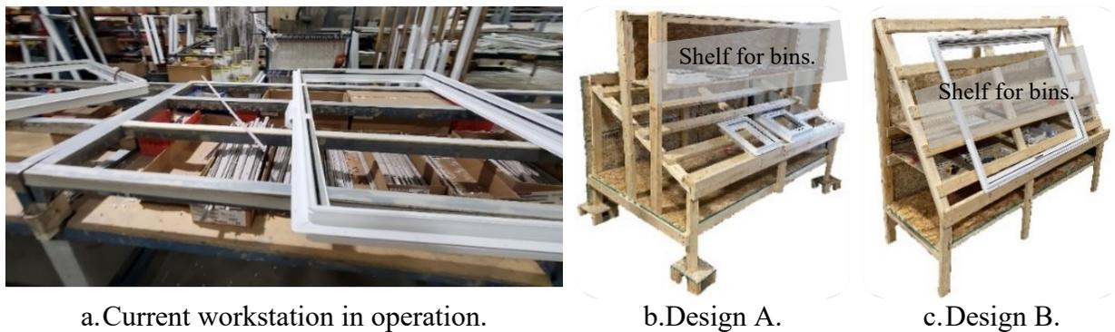
**Figure 5.4: Current workstation design and design options investigated in this study.**
