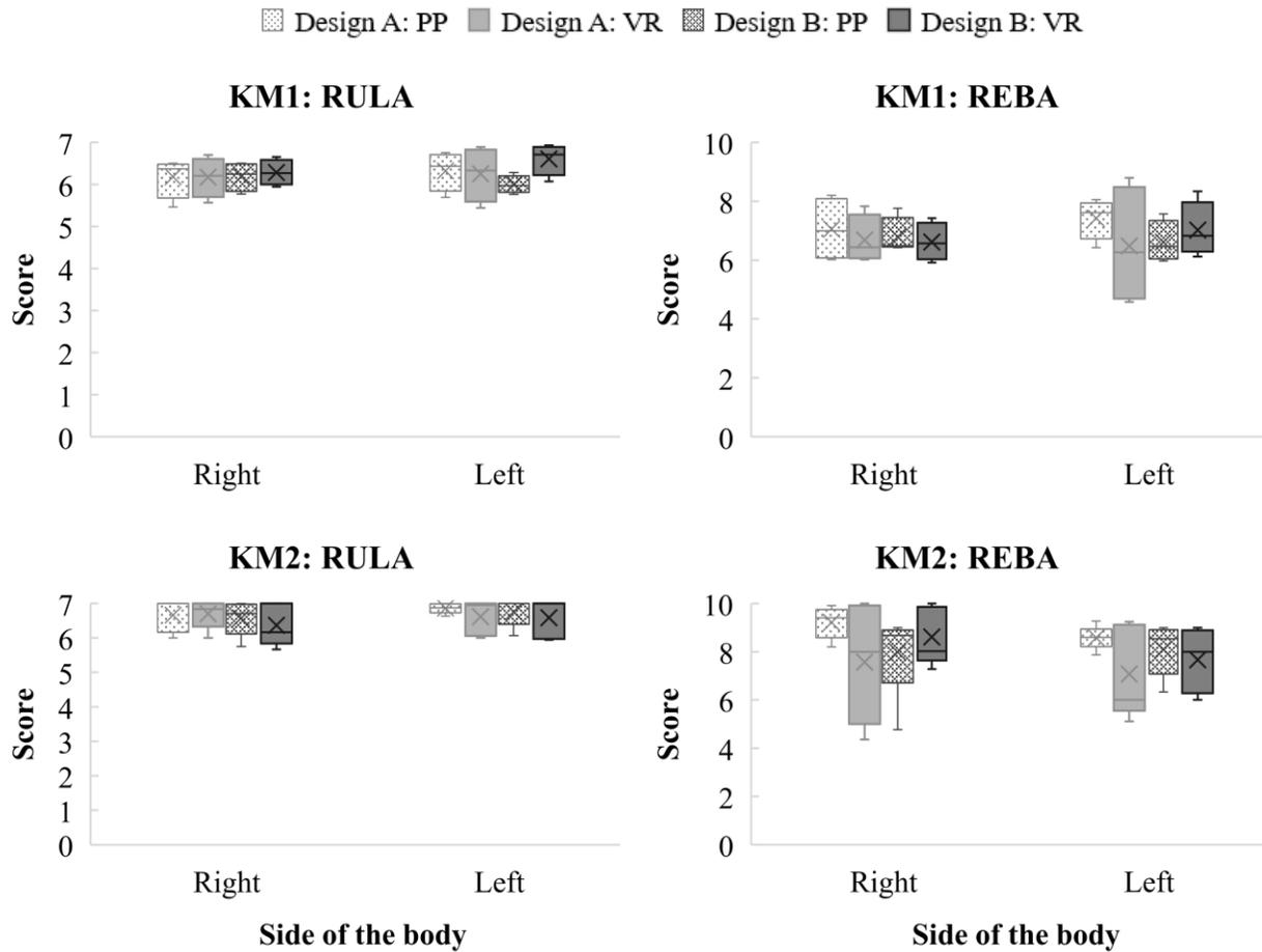
**Figure 5.8: Total RULA and REBA scores per key motions for both design options and environments.**
