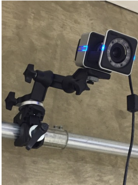
Figure 2.2: Image of the Vero v2.2 camera
