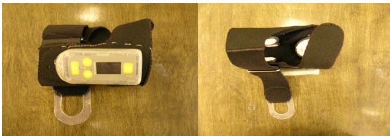
Figure 5.5: The SRS garment. The garment consisted of a wristlet containing a stimulator that was held in place in a rubberized holder similar in shape to a “galosh.” Wettable pad electrodes were electrically connected to the stimulator through insulated stainless steel wires sewn into the glove and leading to a connector in the stimulator holder. Velcro attachments on the electrodes allowed them to be positioned within the glove so as to contact the skin appropriately when the wristlet was donned. The wristlet was supplied with Velcro straps, buckles and loops that allowed the subject to don and doff the garment unaided within 2 minutes.
