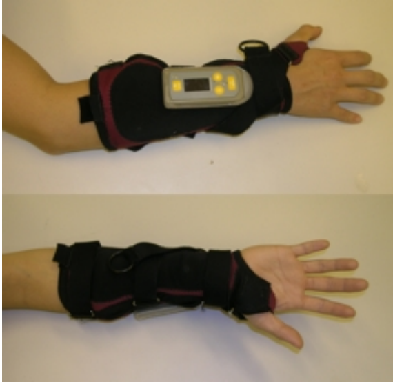
Figure 5.2: The “Hand-E-Stim”, an improved version of the Bionic Glove (Prochazka et al. 1997). It comprised a Neoprene garment with an in-built 3 channel stimulator and surface electrodes that were located over the motor points of the i) long finger extensors and thumb abductor, ii) long finger and thumb flexors and iii) flexor pollicis brevis. An indifferent surface electrode was located inside the garment just proximal to the wrist. The subject produced small tooth clicks that were detected by a wireless earpiece. This sent radio frequency trigger signals to switch the stimulator sequentially between the above motor points, to enable hand grasp and release.
