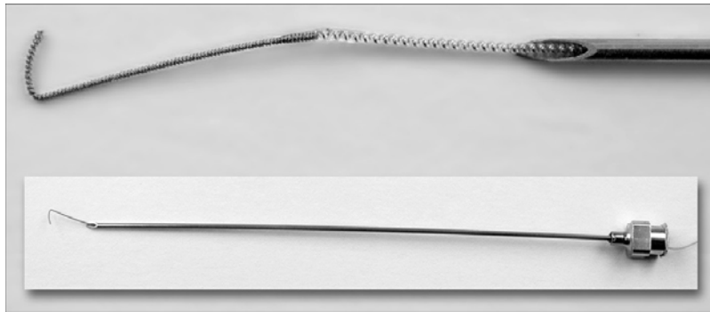
Figure 1.5: Percutaneous intramuscular electrode used in upper-limb FES applications. A 19-gauge needle was used to implant the electrodes. Top: Approximately 8 times actual size. Multifilament, Teflon-insulated, stainless steel wire (200 \mu m diameter) was wound around an arbor into a coil. A length of wire at the end of the electrode lead was deinsulated. The hook was formed by folding back the final deinsulated segment. Bottom: Approximately actual size of the needle loaded with an electrode (adapted from (Knutson et al. 2002)).
