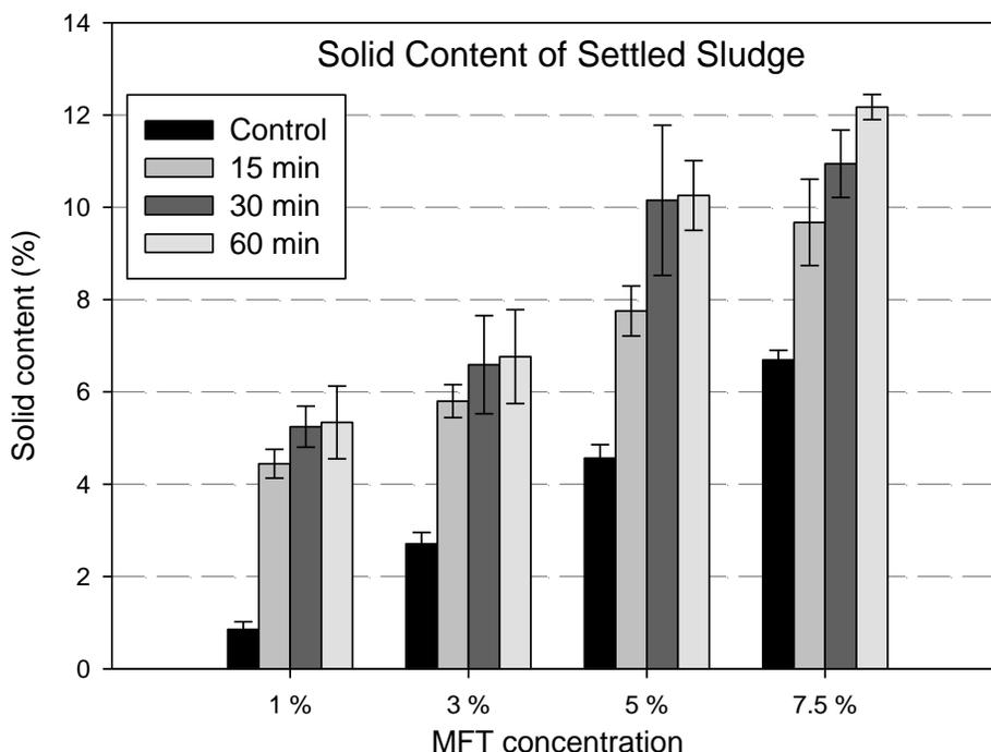
Figure 5. Solids content of MFT settled sludge. MFT suspensions with 1, 3, 5, and 7.5 wt% solid content were treated by 0-(control), 15-, 30-, and 60-minute ozonation. Settled sludge was obtained from the bottom of the suspensions after 24-hour settling. Error bars represent standard deviations of three measurements.
