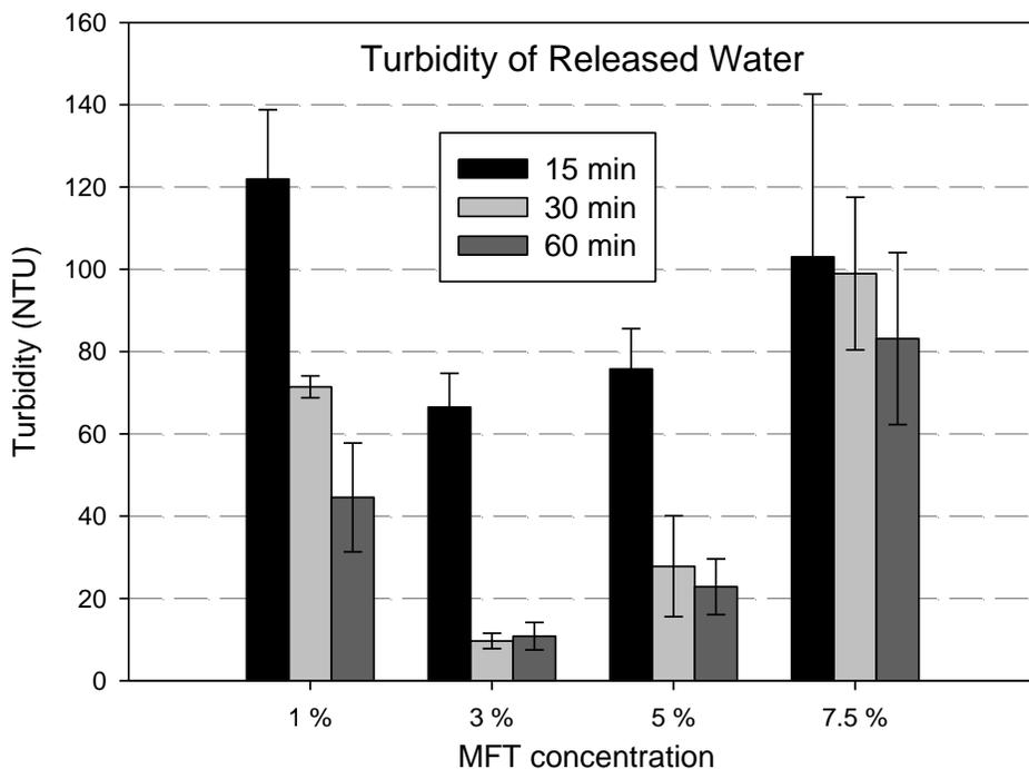
Figure 4. Turbidity of MFT release water generated by ozonation. MFT suspensions with 1, 3, 5, and 7.5 wt% solid content were treated by 15-, 30-, and 60-minute ozonation. Release water was obtained gently after 24-hour settling without causing turbulence. Error bars represent standard deviations of three measurements.
