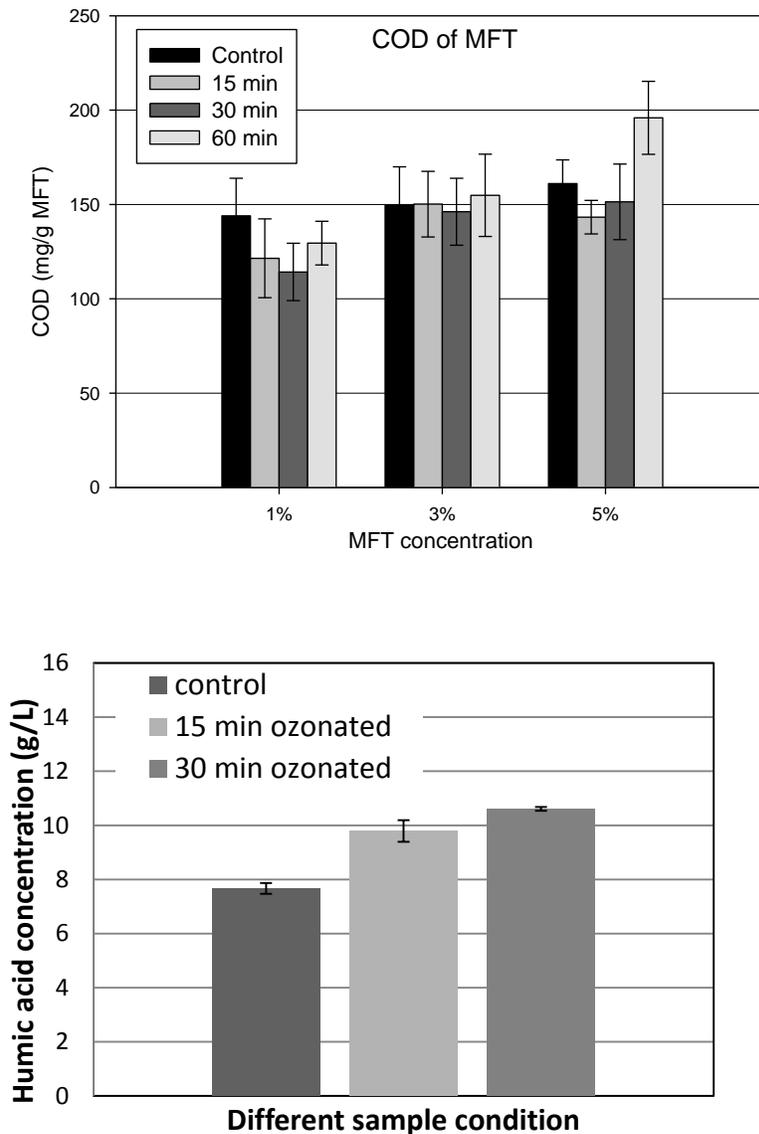
Figure 9. COD and humic acid concentrations in MFT samples before and after ozone treatment. MFT suspensions with 1, 3, and 5 wt% solids content were treated by 0-(control), 15-, 30-, and 60-minute ozonation for COD measurement. MFT suspensions with 3 wt% solid content were treated by 0-(control), 15-, and 30-minute ozonation for humic acid measurements. COD and humic acid were measured after 24-hour settling. Error bars represent standard deviations of three measurements.
