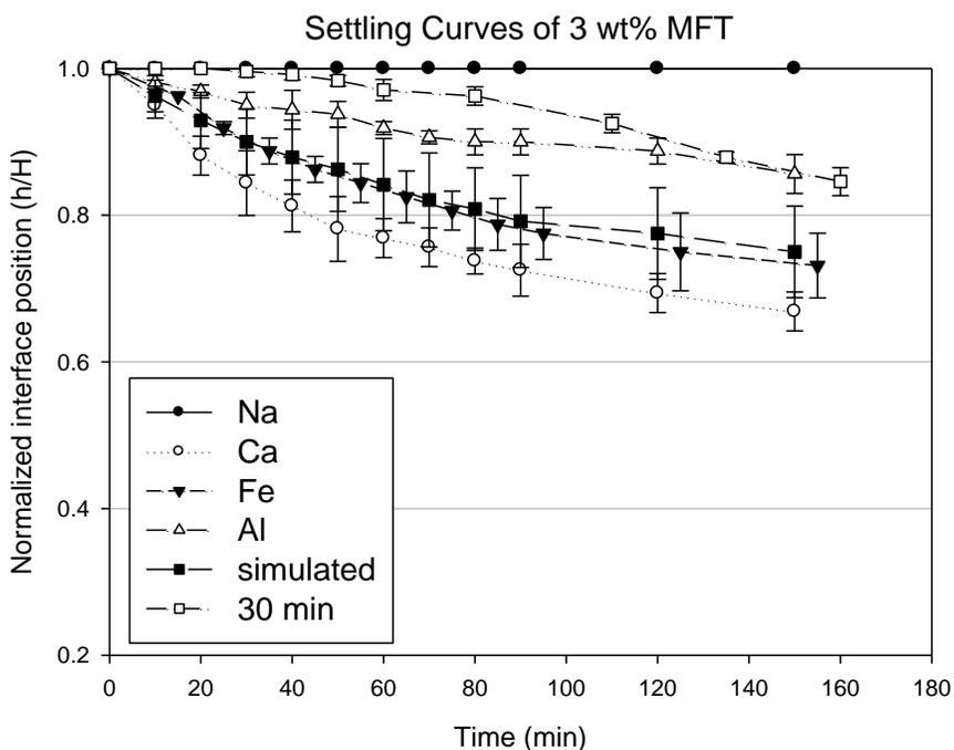
Figure 18. Settling curves of 3 wt% MFT after 24 hours of settling by salt addition. 3 wt% MFT was treated with  $\text{Na}_2\text{SO}_4$ ,  $\text{CaSO}_4$ ,  $\text{Fe}_2(\text{SO}_4)_3$  or  $\text{Al}_2(\text{SO}_4)_3$ . The simulated condition contains the type and amount of metal cations contained in the 3 wt% MFT sample after 30 minutes of ozonation. 3 wt% MFT settled by 30-minute ozonation is shown for comparison. Error bars represent standard deviations of three measurements.
