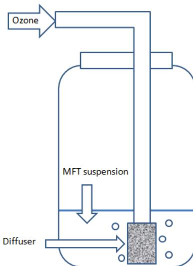
Figure 1. Schematic of MFT ozonation apparatus.
