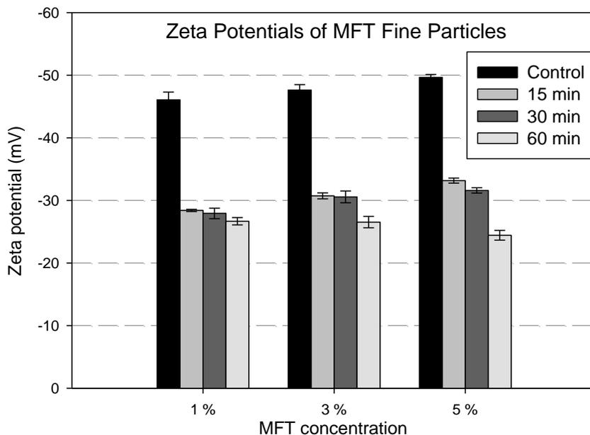
Figure 10. Zeta potentials of MFT fine particles. MFT suspensions with 1, 3, and 5 wt% solids content were treated by 0-(control), 15-, 30-, and 60-minute ozonation. The zeta potential was measured at  $22 \pm 1$  °C after 24-hour settling. Error bars represent standard deviations of three measurements.
