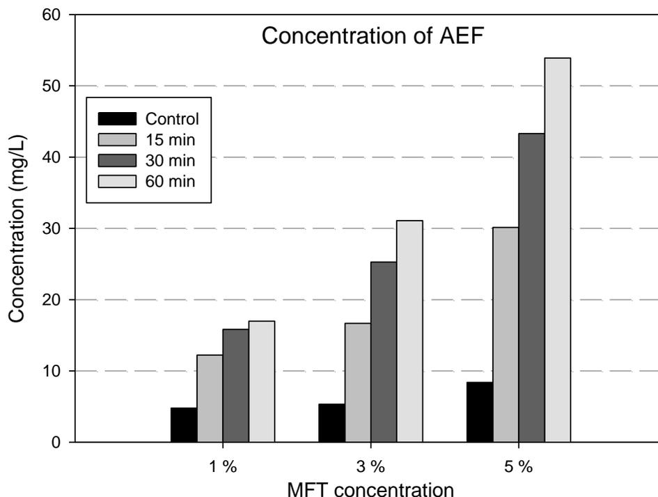
Figure 8. Acid extractable fraction concentration in MFT release water. MFT suspensions with 1, 3, and 5 wt% solids content were treated by 0-(control), 15-, 30-, and 60-minute ozonation. AEF concentration was measured after 24-hour settling.
