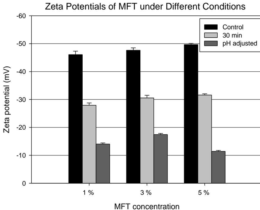
Figure 16. Zeta potentials of acidified and ozonated MFT suspensions. Zeta potential was measured at  $22 \pm 1$  °C after 24-hour settling. Ozone was applied for 30 minutes. Error bars represent standard deviations of three measurements.
