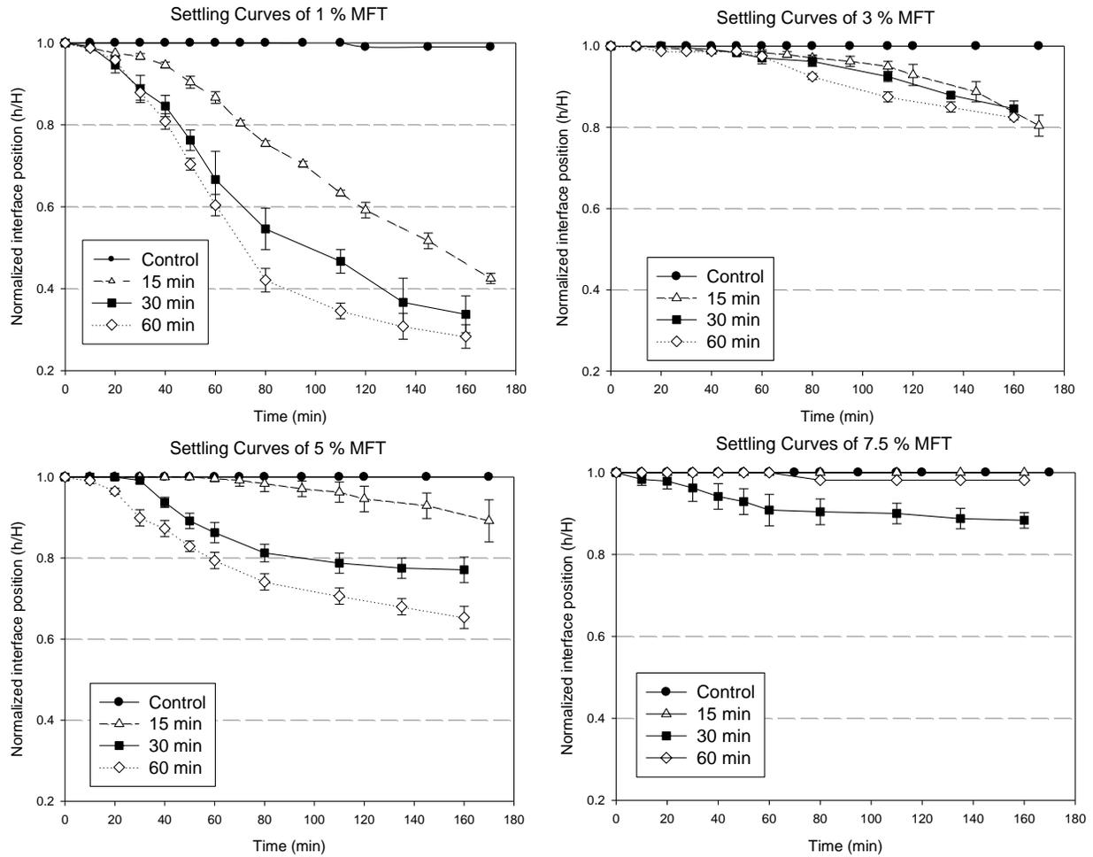
Figure 3. Settling curves of MFT suspensions under different ozonation conditions. MFT suspensions with 1, 3, 5, and 7.5 wt% solid content were treated with 0 (control), 15, 30, and 60 minutes of ozonation.  $H$  is the total height of the suspension;  $h$  represents the height of the solid-liquid interface. Error bars represent standard deviations of triplicate samples.
