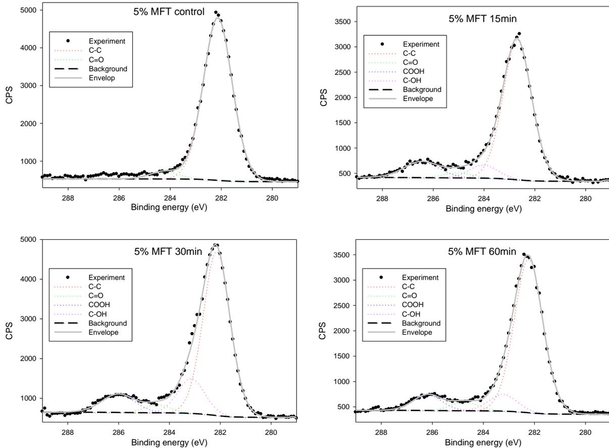
Figure 13. Surface chemical bonding of 5 wt% MFT. MFT suspensions with 5 wt% solids content were treated by 0-(control), 15-, 30-, and 60-minute ozonation. Counts per second (CPS) represents the strength of signal. A stronger signal reflects a relatively larger amount of chemical bonding. Coloured lines indicate the type of chemical bond.
