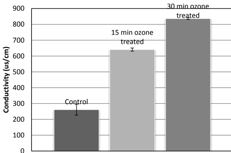
Figure 7. Conductivity of 3 wt% MFT suspensions after 24 hours settling. MFT suspensions were treated with 0-(control), 15-, and 30-minute ozonation. The conductivity was measured after 24-hour settling. Error bars represent standard deviations of three measurements.
