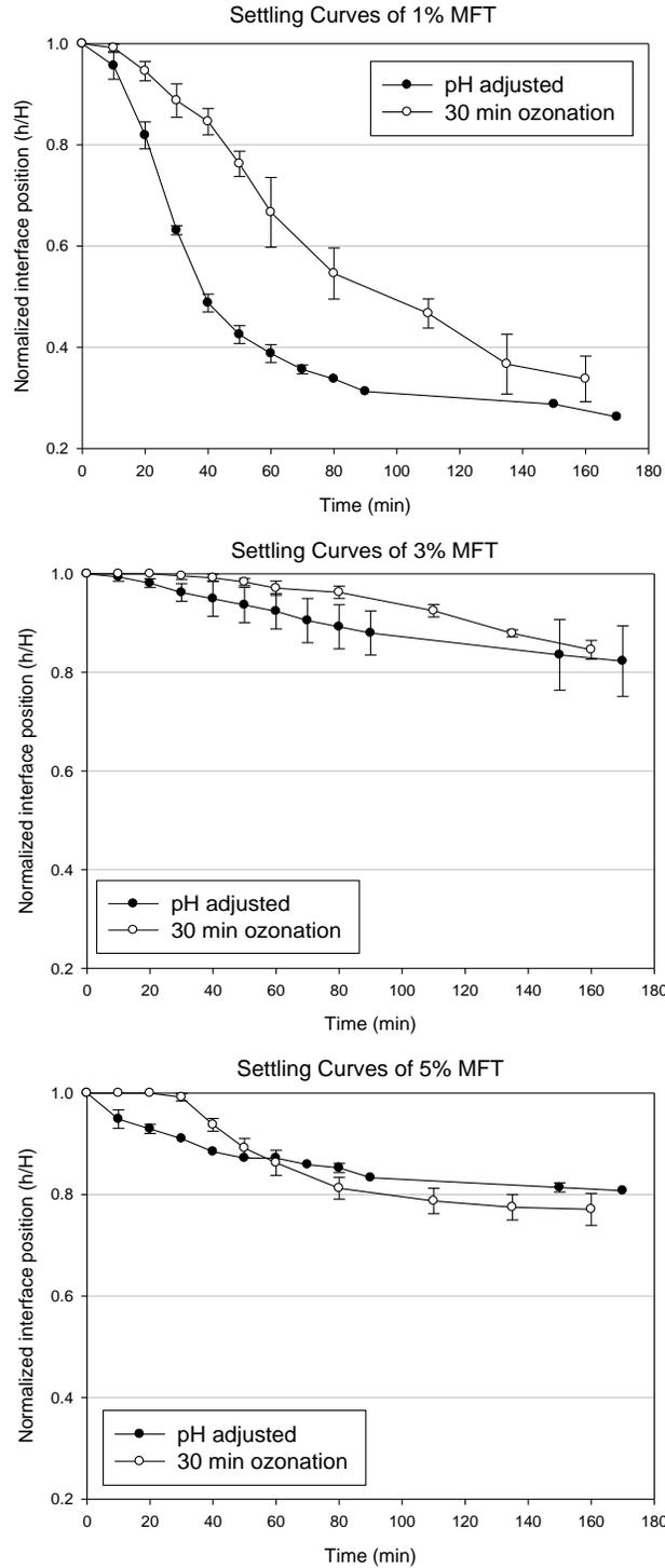
Figure 15. Settling curves of acidified and ozonated MFT. H is the total height of the suspension and h represents the height of solid-liquid interface. Error bars represent standard deviations of three measurements.
