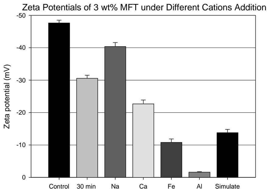
Figure 19. Zeta potentials of 3 wt% MFT samples after salt addition. The zeta potential was measured at  $22 \pm 1$  °C after 24-hour MFT settling. For comparison, the zeta potentials of 3 wt% MFT with 30-minute ozonation and without ozonation (control) are included. Error bars represent standard deviations of three measurements.
