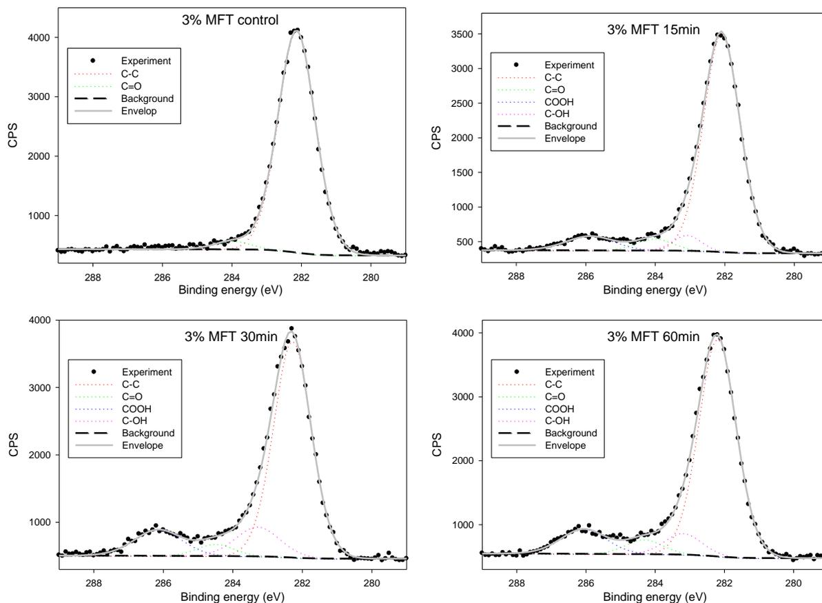
Figure 12. Surface chemical bonding of 3 wt% MFT. MFT suspensions with 3 wt% solids content were treated by 0-(control), 15-, 30-, and 60-minute ozonation. Counts per second (CPS) represents the strength of signal. A stronger signal reflects a relatively larger amount of chemical bonding. Coloured lines indicate the type of chemical bond.
