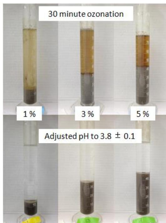
Figure 14. Photographs of MFT after adjusting the pH to  $3.8 \pm 0.1$  using concentrated hydrochloric acid and 24 hours of settling. The original pH values of 1, 3, and 5 wt% MFT were  $7.7 \pm 0.60$ ,  $8.7 \pm 0.07$ , and  $9.0 \pm 0.10$ , respectively. For comparison, images of MFT ozonated for 30 minutes and settled for 24 hours are also shown.
