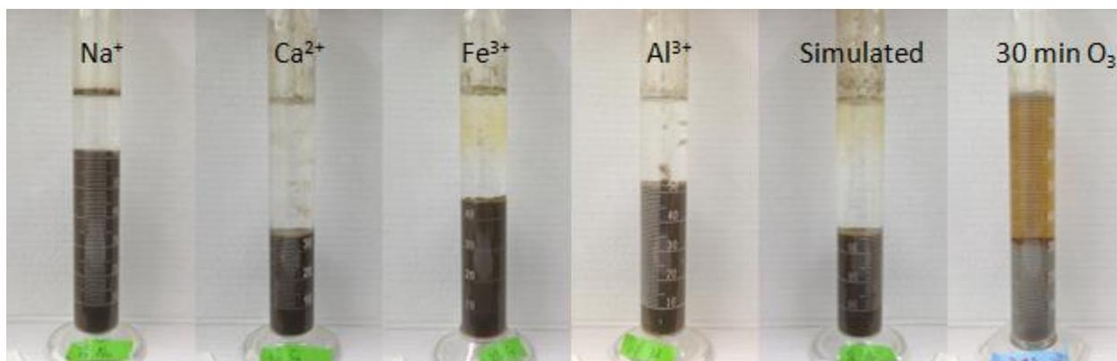
Figure 17. Photographs of 3 wt% MFT after 24 hours of settling by salt addition. 3 wt% MFT was treated with  $\text{Na}_2\text{SO}_4$ ,  $\text{CaSO}_4$ ,  $\text{Fe}_2(\text{SO}_4)_3$  or  $\text{Al}_2(\text{SO}_4)_3$ . The simulated condition contains the type and amount of metal cations contained in the 3 wt% MFT sample after 30 minutes of ozonation. 3 wt% MFT settled by 30-minute ozonation is shown for comparison.
