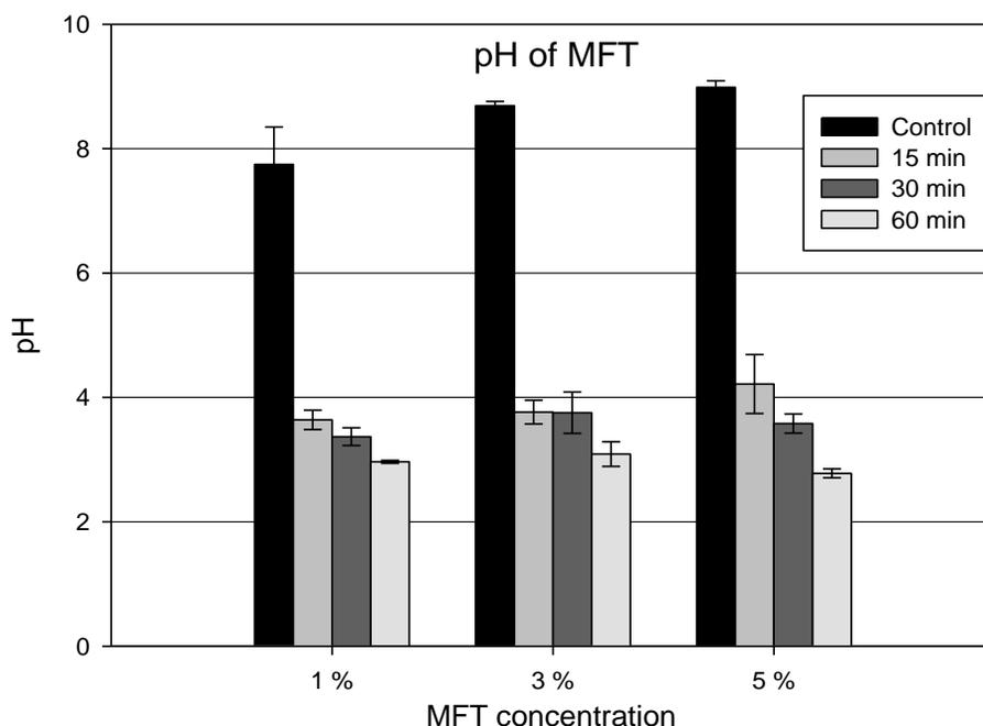
Figure 6. pH of MFT suspensions after 24 hours settling. MFT suspensions with 1, 3, and 5 wt% solids content were treated with 0-(control), 15-, 30-, and 60-minute ozonation. The pH was measured after 24-hour settling. Error bars represent standard deviations of three measurements.
