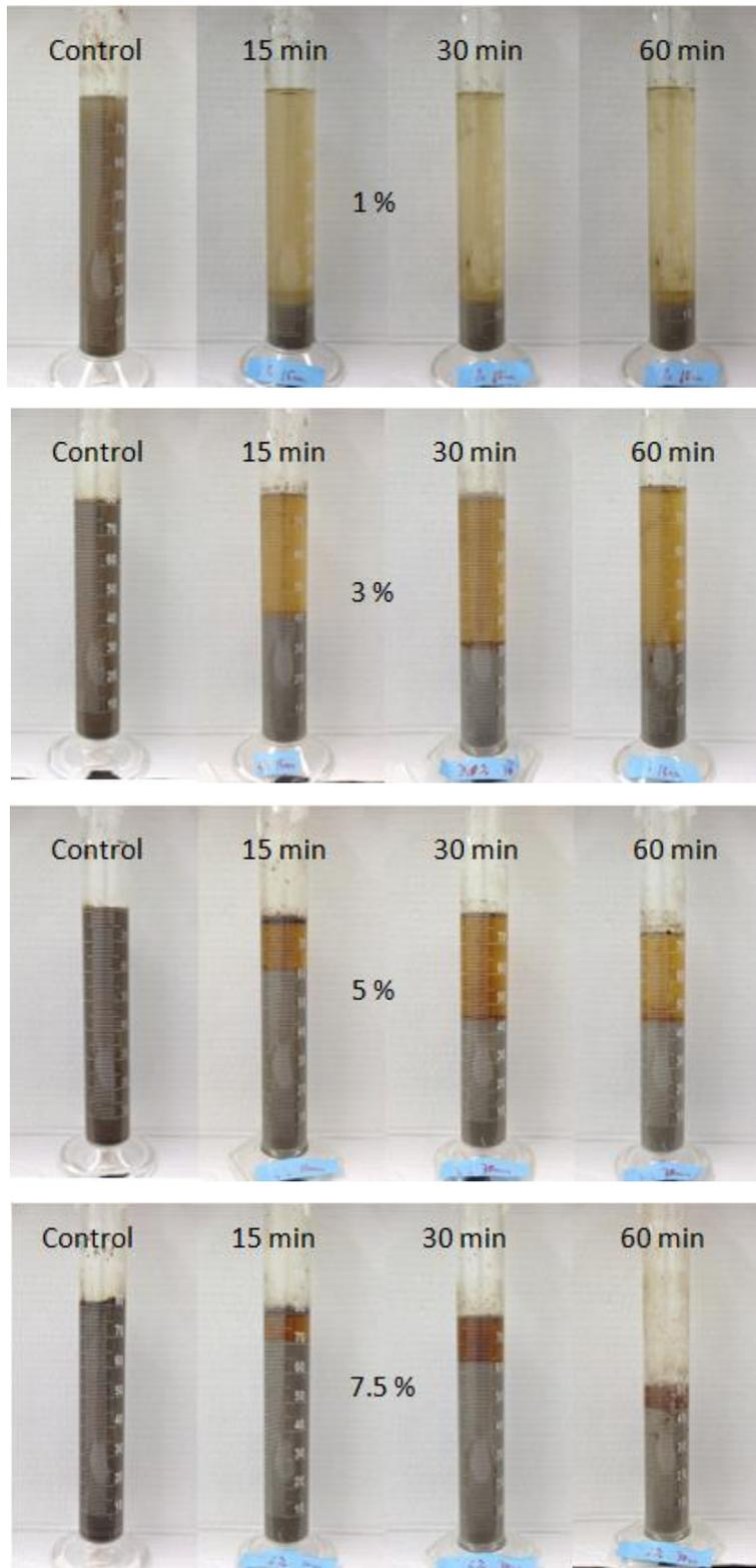
Figure 2. Photographs of MFT suspensions after 24 hours of settling. MFT suspensions with 1, 3, 5, and 7.5 wt% solid content were treated by ozonation for 0 (control), 15, 30, and 60 minutes.
