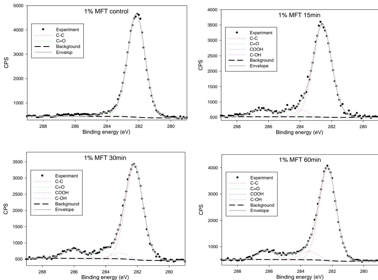
Figure 11. Surface chemical bonding of 1 wt% MFT. MFT suspensions with 1 wt% solids content were treated by 0-(control), 15-, 30-, and 60-minute ozonation. Counts per second (CPS) represent the strength of signal; a stronger signal reflects a relatively larger amount of chemical bonding. Coloured lines indicate the type of chemical bond.
