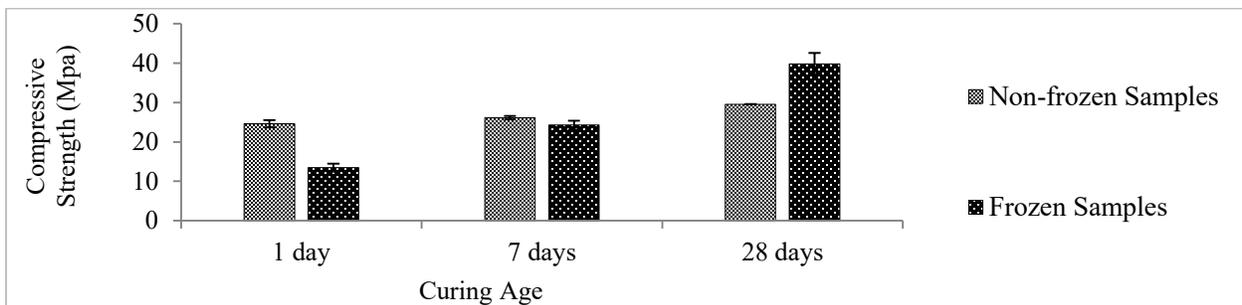
Figure 3-11: Effect of initial freezing on grout-1 at fluidic consistency (25% of water content)
