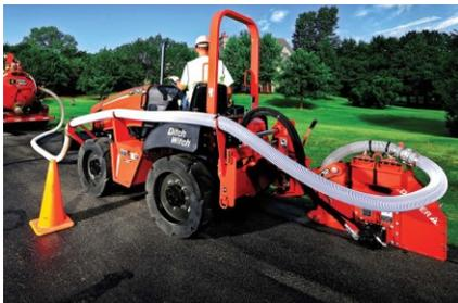
**Figure 2-4: MTT equipment of Ditch Witch (Ditch Witch 2010)**
