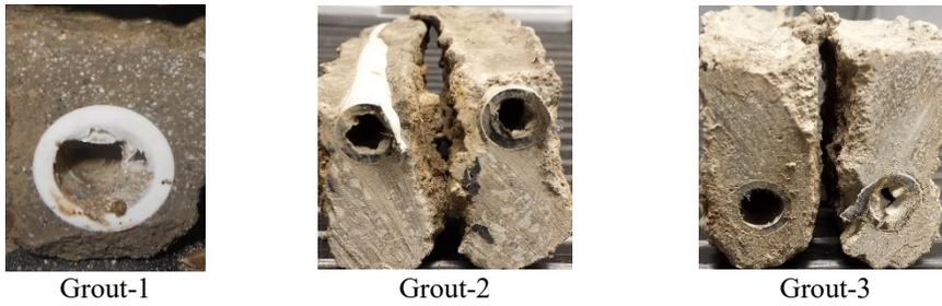
**Figure 3-9: Grout coverage around the conduit**
