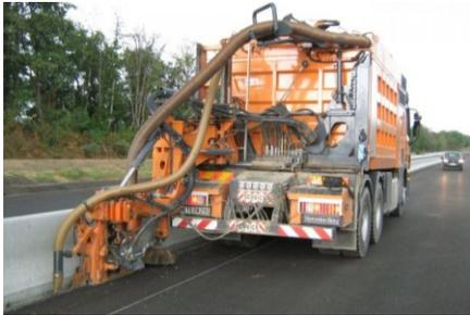
**Figure 2-5: Meteor for MTT machines (Marais 2012a)**
