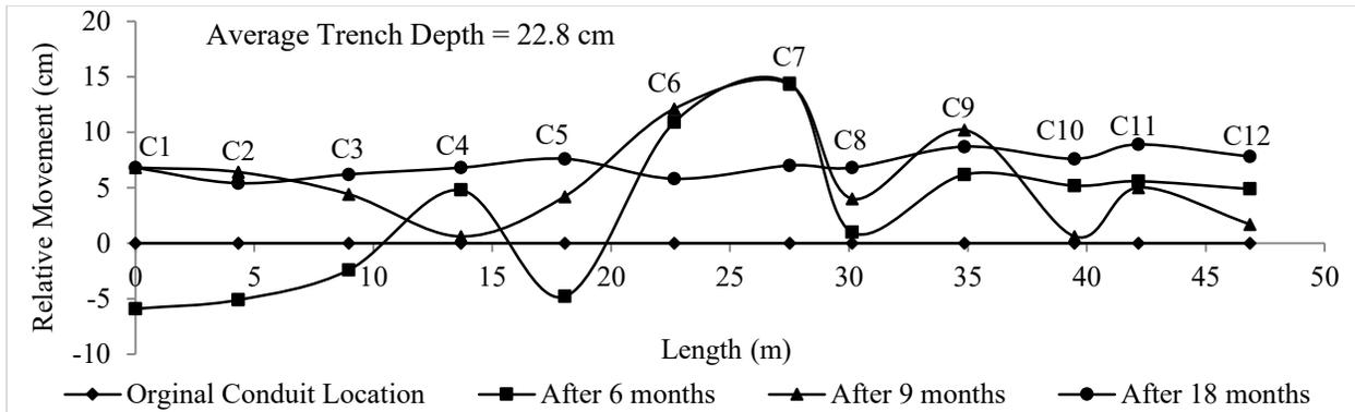
Figure 3-3: Conduit movement of VIF technology - Layout 3
