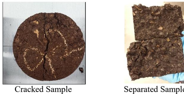
Figure 4-1: Types of sample failures
