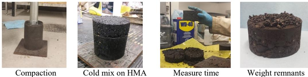
**Figure 4-3: Procedure of the adhesiveness test**
