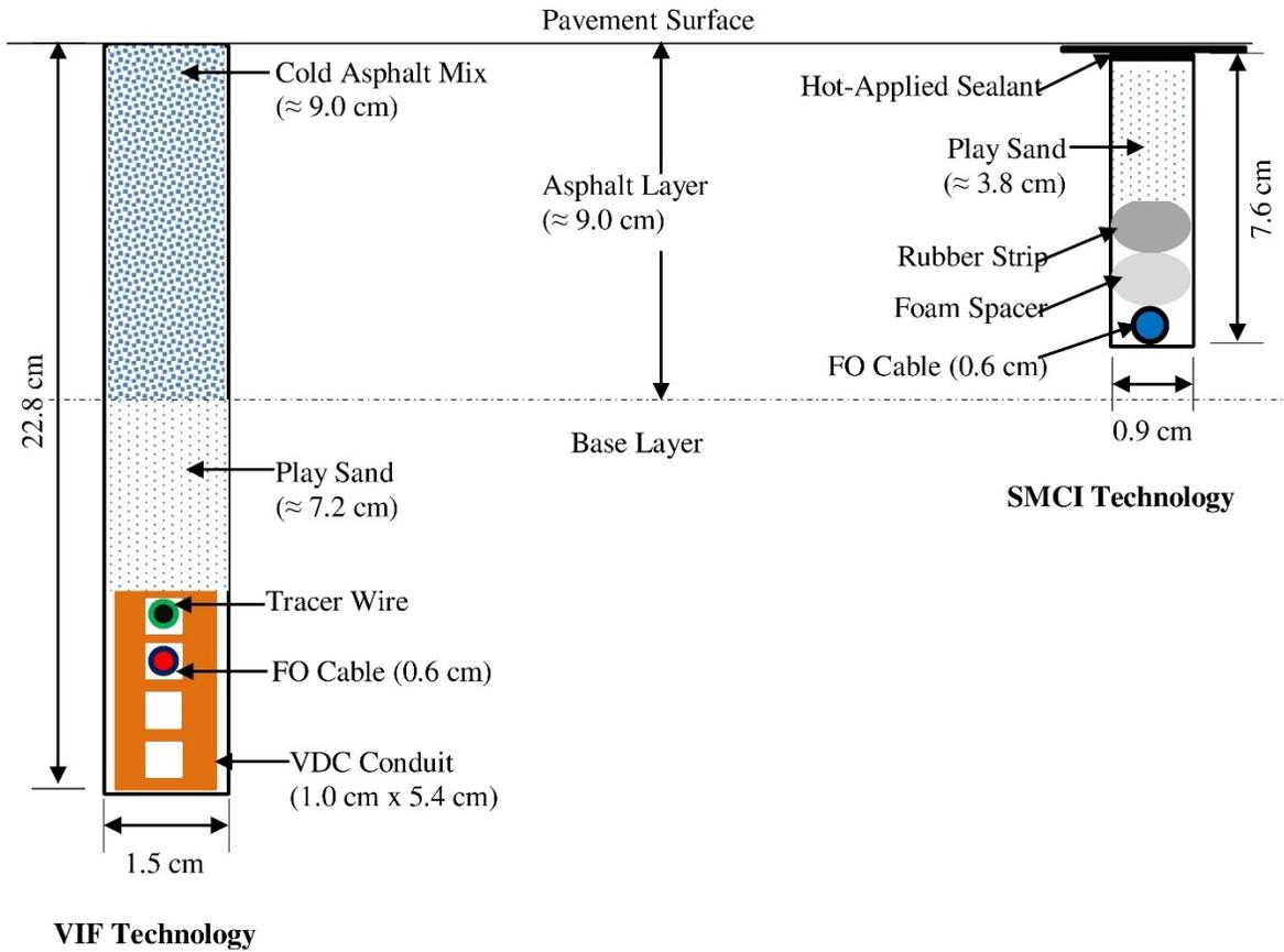
**Figure 3-2: Cross-sections and backfilling details of MTT pilot installations (not to scale)**
