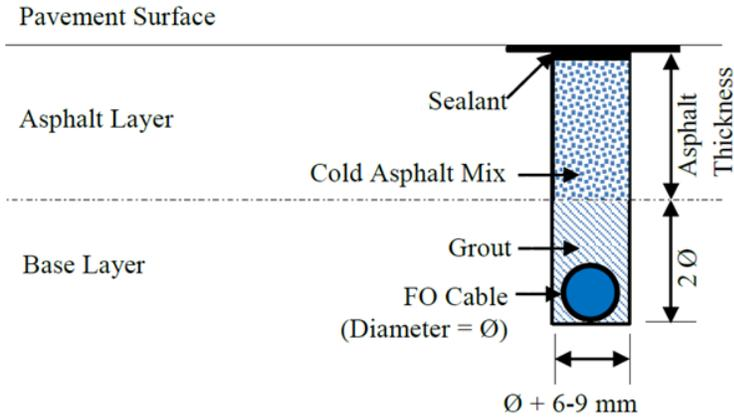
**Figure 3-7: Cross-section of modified MTT backfilling**
