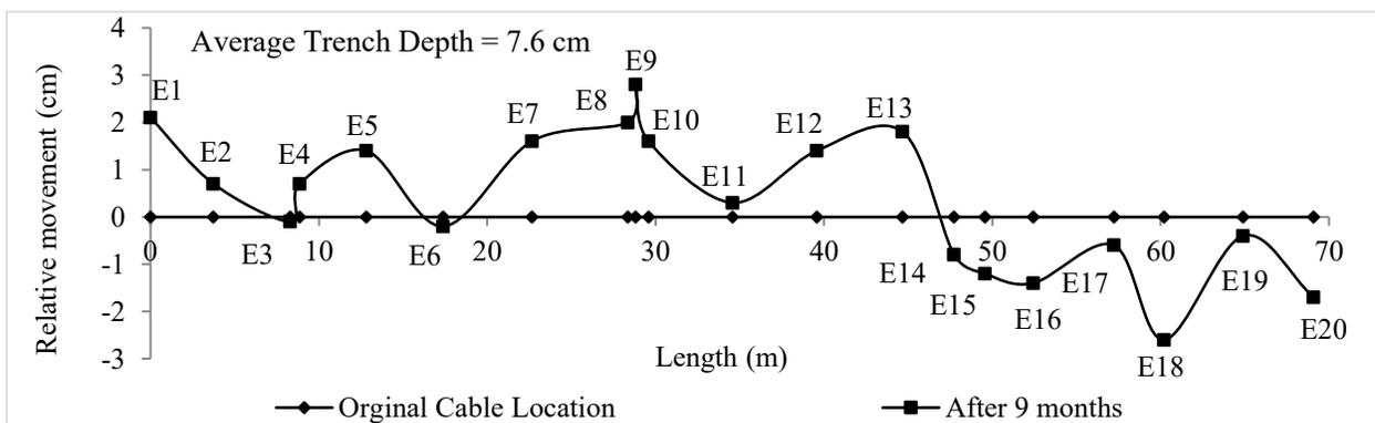
Figure 3-4: Conduit movement of SMCI technology - Layout 2
