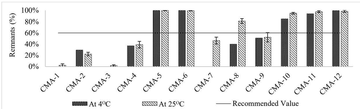
Figure 4-6: Results of cohesion (rolling sieve) test
