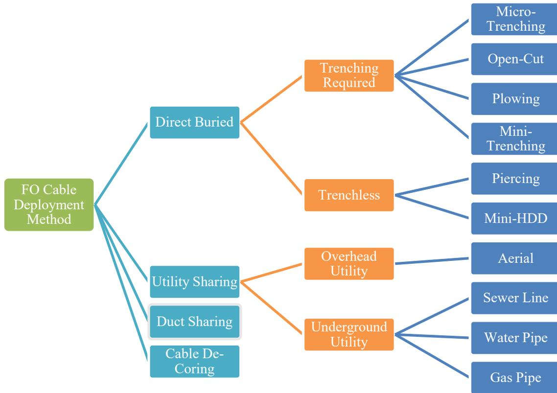
**Figure 2-1: FO network deployment methods**
