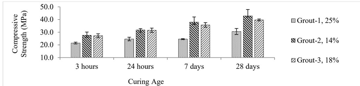
**Figure 3-10: Grout compressive strength test results**
