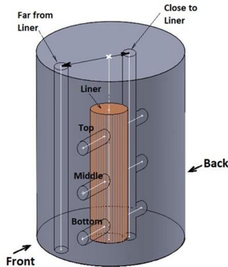
**Figure 10.** Schematic showing the locations of horizontal and vertical cores taken from the sand pack after the test
