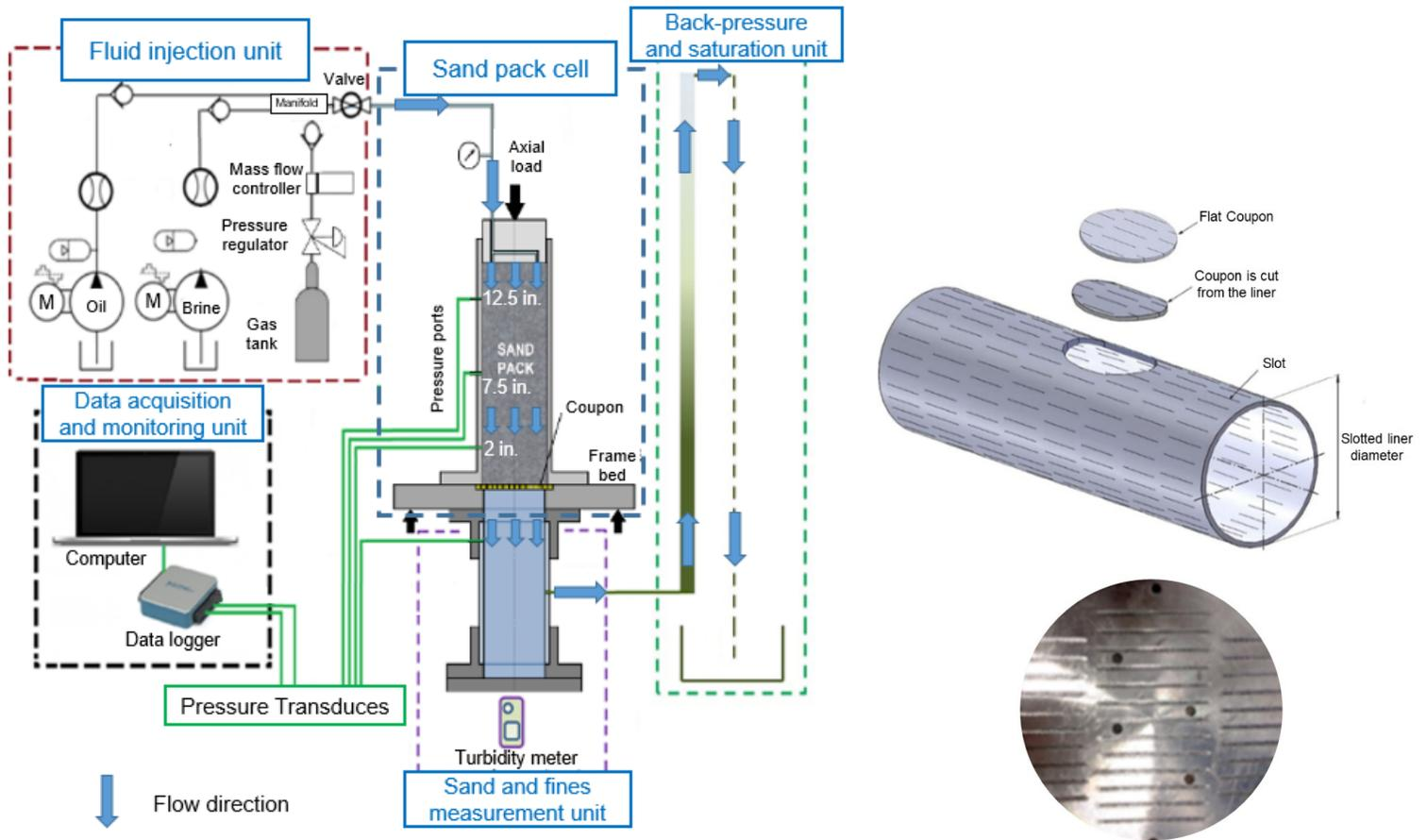
**Figure 2.** Typical schematics of a sand retention testing facility (Montero et al., 2020) and a coupon as a cut-out from a real screen
