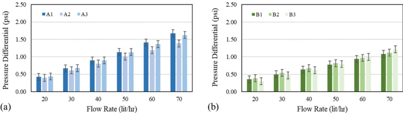
**Figure 9.** Differential pressure between the ports located a) far from, and b) close to the liner and a port located inside the liner in Test#2
