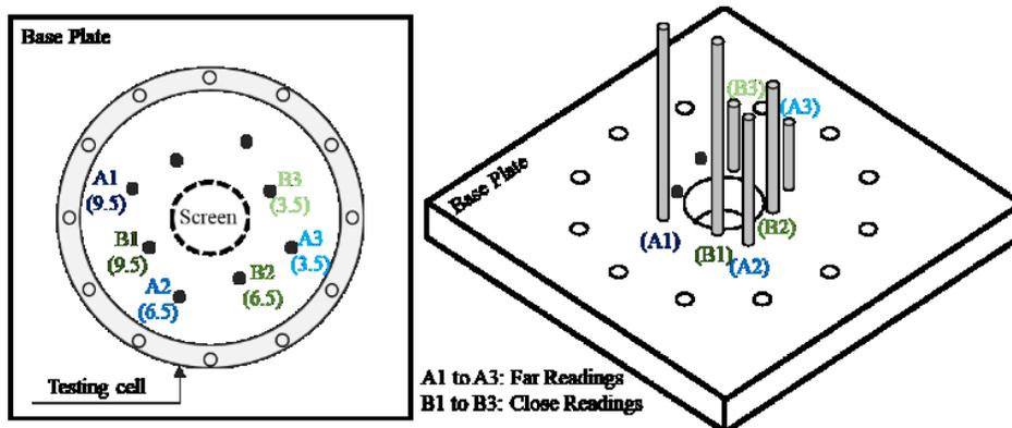
**Figure 5.** Schematic of the pressure port locations around the liner and their labels; top and side view (the numbers below each label is the height of the pressure port in inches)
