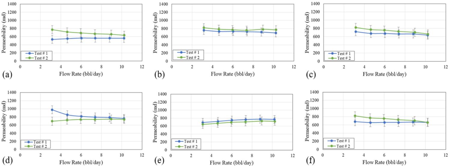
**Figure 15.** Comparing the permeability values calculated for Tests #1 and #2 at different locations; a) A1, b) A2, c) A3, d) B1, e) B2, and f) B3
