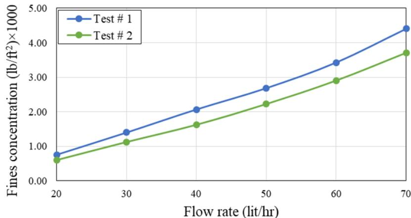
Figure 16. Cumulative produced fines concentration in the discharge water
