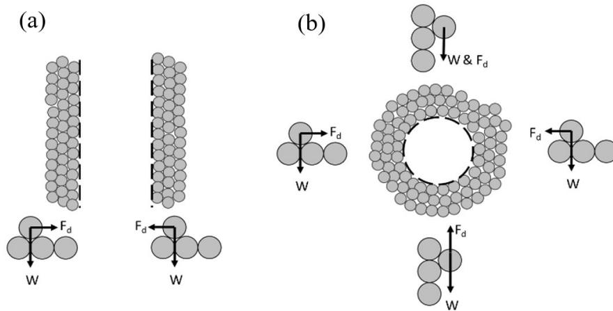
**Figure 3.** Physical forces acting on grains around the a) vertical, and b) horizontal wellbore in an unconsolidated oil sand reservoir
