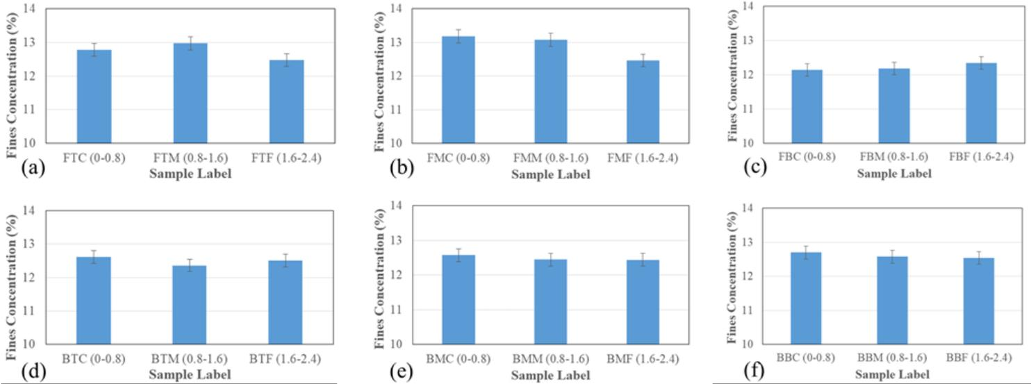
**Figure 11.** Fines concentration in the horizontal samples in Test#2 from the sand pack at a) Front side-Top, b) Front side-Middle, c) Front side-bottom, d) Backside-Top, e) Backside-Middle, and f) Backside-Bottom
