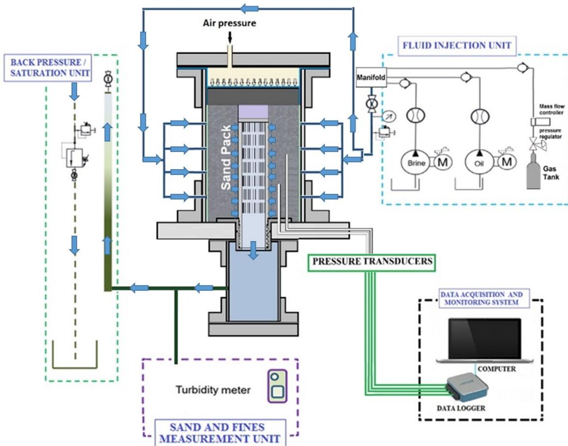
**Figure 4.** Full-scale Completion Test Facility (FCT); (blue arrows show the flow direction during the test)
