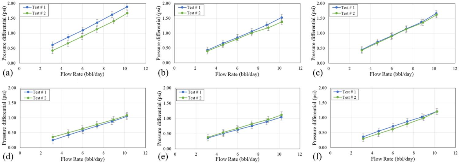
**Figure 14.** Comparing the differential pressures recorded in Tests #1 and #2 at different measurement locations; a) A1, b) A2, c) A3, d) B1, e) B2, and f) B3
