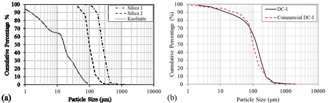
Figure 6. a) PSD curves for three commercial sands, and b) PSD curves for original DC-I (Abram and Cain, 2014), and replicated DC-I from the commercial sands
