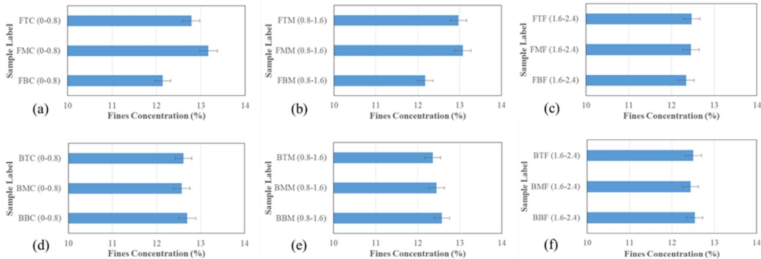
**Figure 12.** Fines concentration inside the samples located at different distances from the liner, a) Front side-Close to the liner, b) Front side-Middle distance to the liner, c) Front side-Far from the liner, d) Backside-Close to the liner, e) Backside-Middle distance to the liner, and f) Backside-Far from the liner
