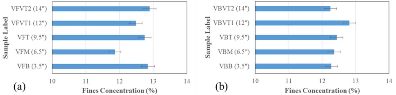
**Figure 13.** Fines concentration inside the vertical samples, a) Front side-Far from the liner, and b) Backside-Close to the liner
