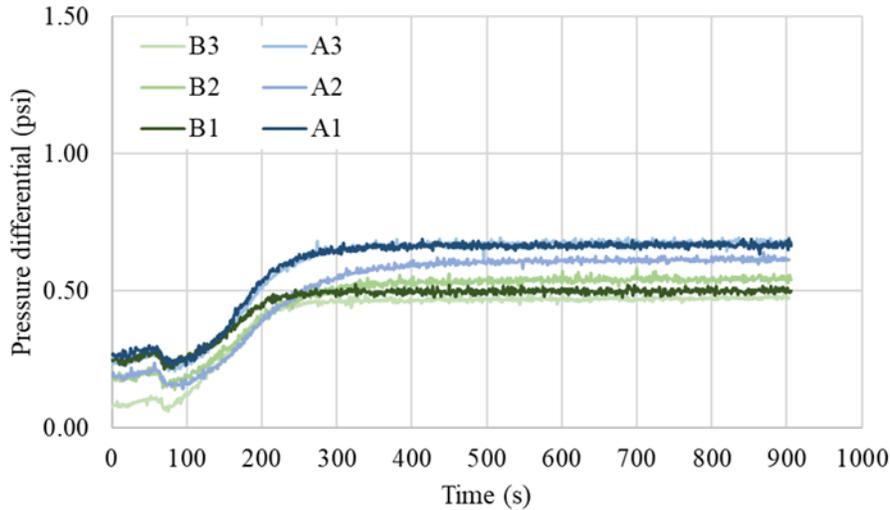
**Figure 8.** Pressure stabilization at the different pressure ports when injecting brine at 30 lit/hr in Test#2
