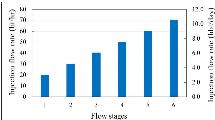
**Figure 7.** Step rate flow for single-phase brine injection during the FCT
