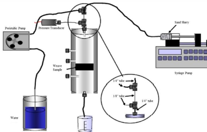
**Figure 1.** Typical schematics of a slurry-type sand retention testing facility (after Montero et al., 2018)
