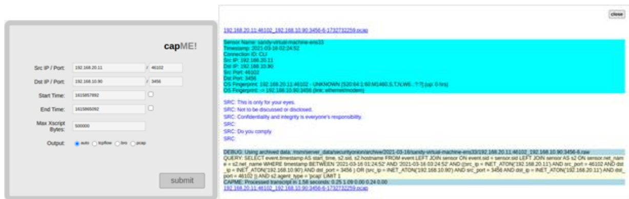
Fig. 74. CapMe view and auto option view for view full transcript with an option to download pcap
