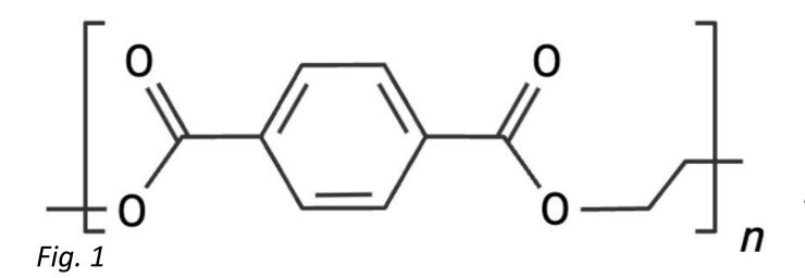
PET (Fig. 1) is an example of a thermoplastic. PET is commonly used in plastic bottles. It is capable of being re-melted and re-formed into a new bottle or formed into a different plastic object. Additionally, PET is the most wasted type of plastic.
