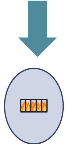
(Fig. 6) The shreds are melted and put through an extruder.
