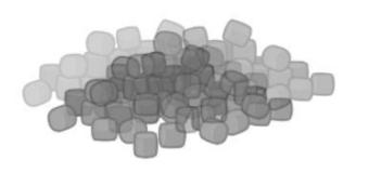
(Fig. 7) The extruder creates pellets, which can later be melted into filaments.
