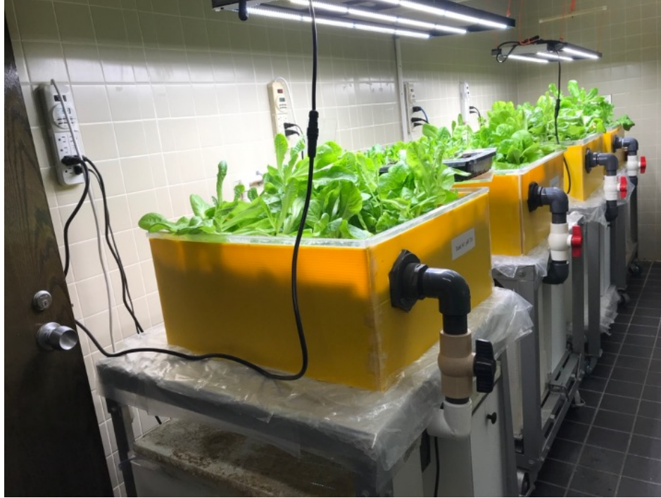
Figure 3.1 Four floating raft aquaponics mini-systems were built. Each mini-system consisted of a recirculating aquaculture unit and a hydroponic bed above the system. Each hydroponic tank contained a single raft supporting 14 plants equipped with overhead LED lighting operating 18 h/d.
