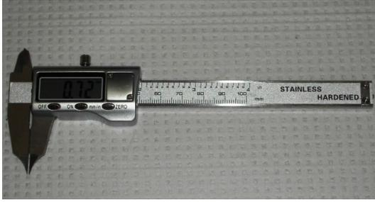
Figure 3-7: Digital calipers.
