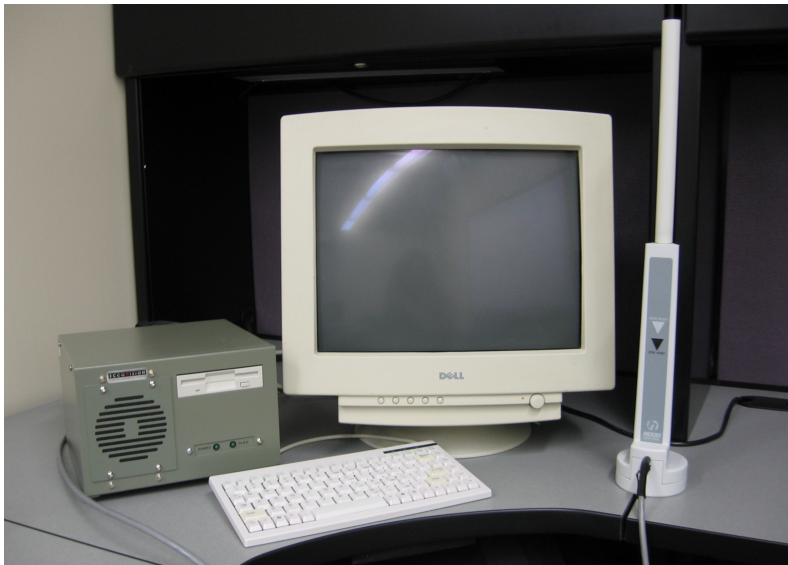
Figure 3-5: Eccovision® 4.50 acoustic rhinometer
