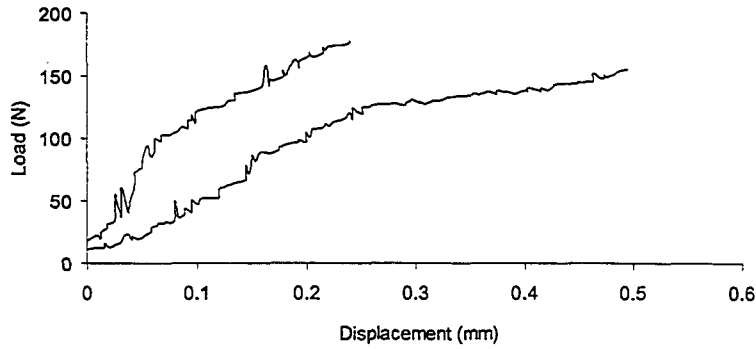
Figure D16 Load displacement curve for Tekflex PM on split limestone substrate.
