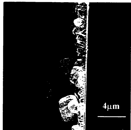
Fig. 4.10 Cleaved cross-section images of the deposits obtained at different ON times at a constant peak current density of 10 \text{ mA/cm}^2 and OFF time of 8 ms.
