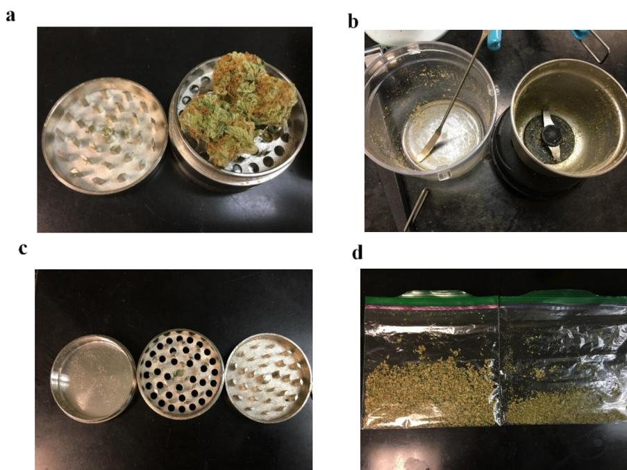
**Figure 2.3 Pulverization of cannabis raw samples using manual grinder and electric blender.** (a) manual grinder and (b) electric blender. (c) The inside of manual grinder is relatively clean without much resin left behind whereas there is a layer of resin stuck to the inside of the cup of the electric blender. (d) The resultant particle size is larger using the manual grinder (left) than the electric blender (right).
