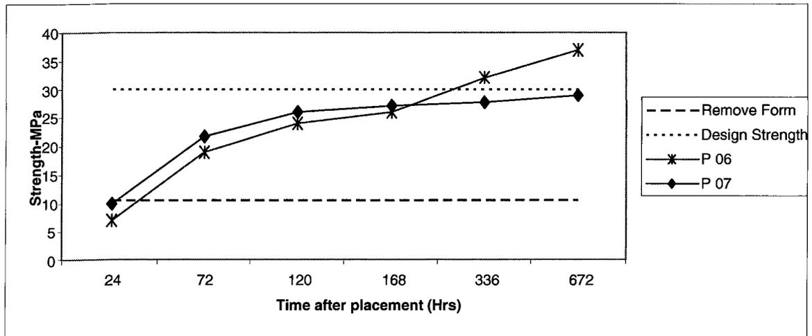
*Figure 4.6 Strength Development Curve of Vessel Base*
