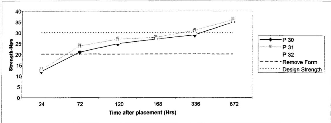
Figure 4.18 Strength Development Curve of the Equipment Table Top
