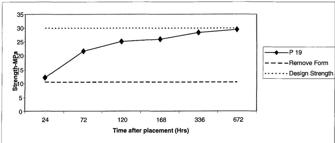
*Figure 4.12 Strength Development Curve of Exchanger Structure Pier*
