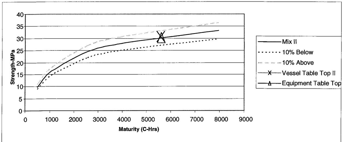
Figure 4.20 Verification of Strength-Maturity Relationship Curve of Design Mix II
