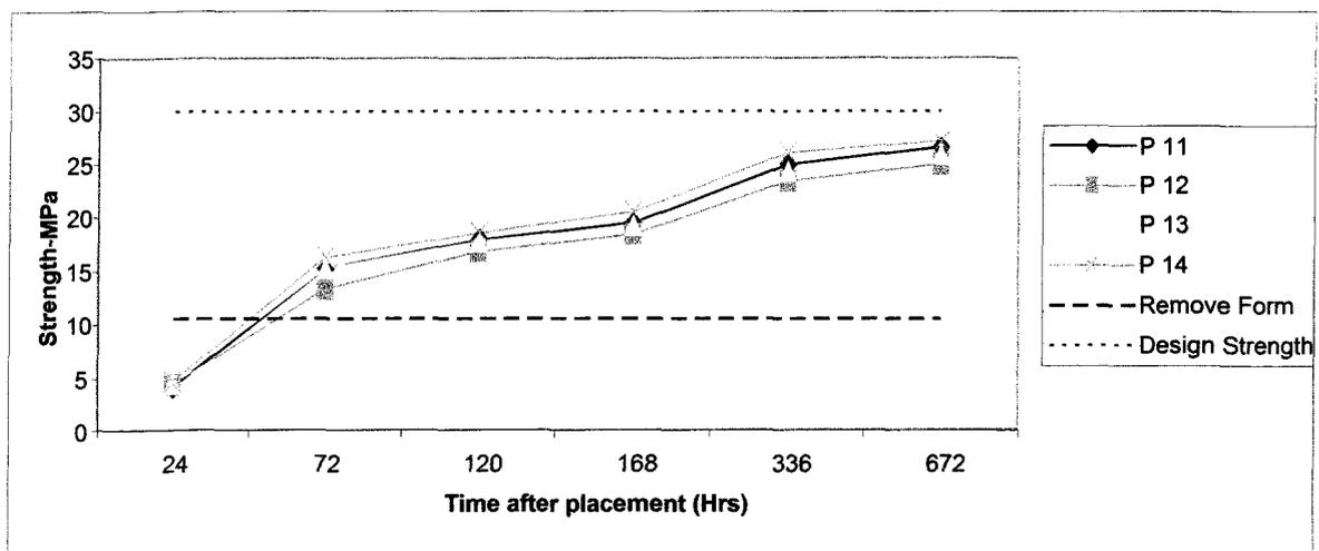
Figure 4.8 Strength Development Curve of Substation Paving Slab
