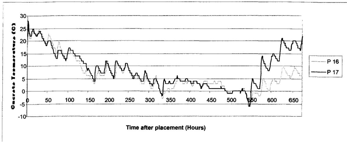
*Figure 4.9 Concrete Temperature Developments for the Steel Structure Base*
