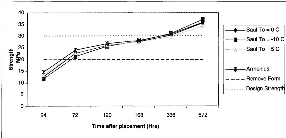
Figure 5.8 Datum temperature sensitivity analysis of the equipment table top
