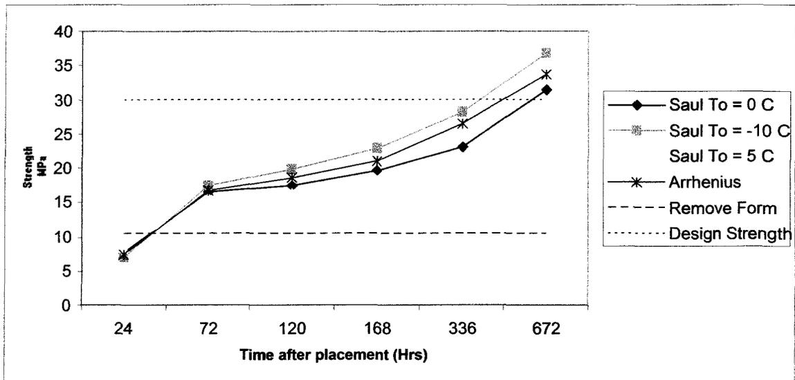
Figure 5.6 Datum temperature sensitivity analysis of building grade beam
