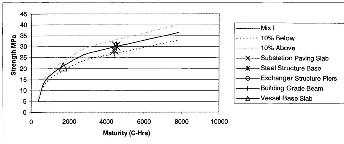
*Figure 4.19 Verification of Strength-Maturity Relationship Curve of Design Mix I*
