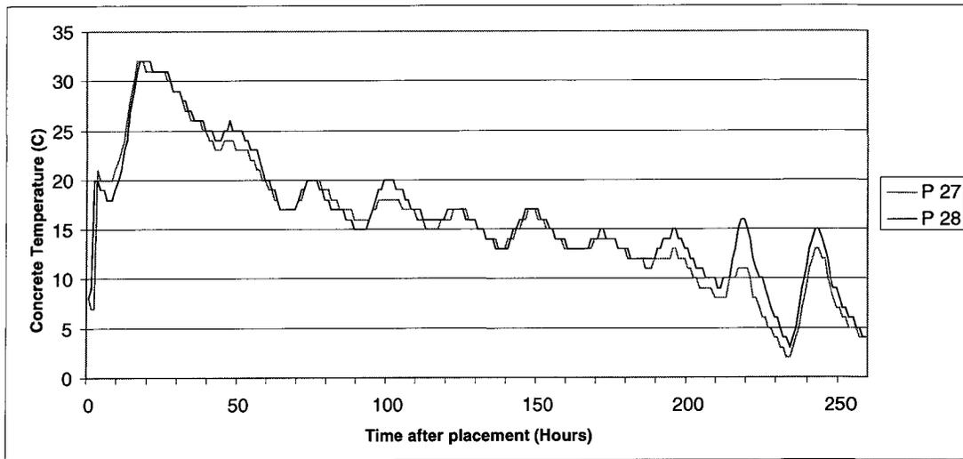
*Figure 4.15 Concrete Temperature Developments for the Vessel Table Top II*
