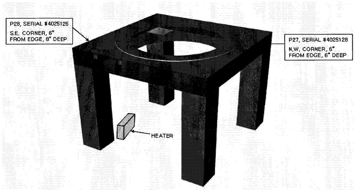
Figure A.7 Location IX, Vessel Table Top II
