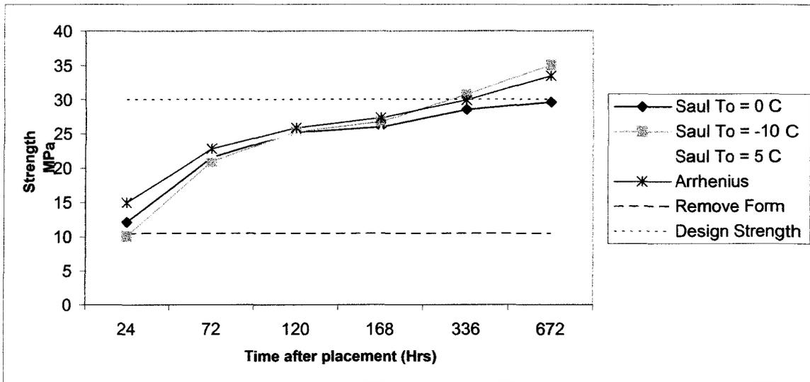
Figure 5.5 Datum temperature sensitivity analysis of exchanger structure pier
