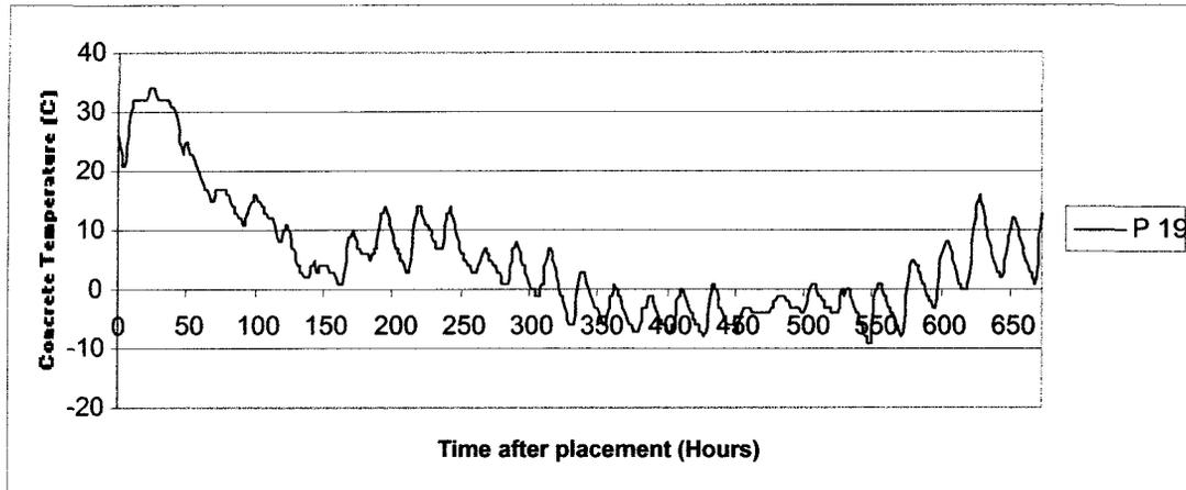
*Figure 4.11 Concrete Temperature Developments for the Exchanger Structure Piers*
