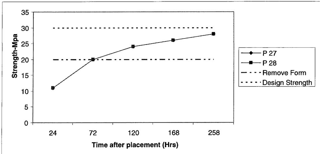
*Figure 4.16 Strength Development Curve of Vessel Table Top II*
