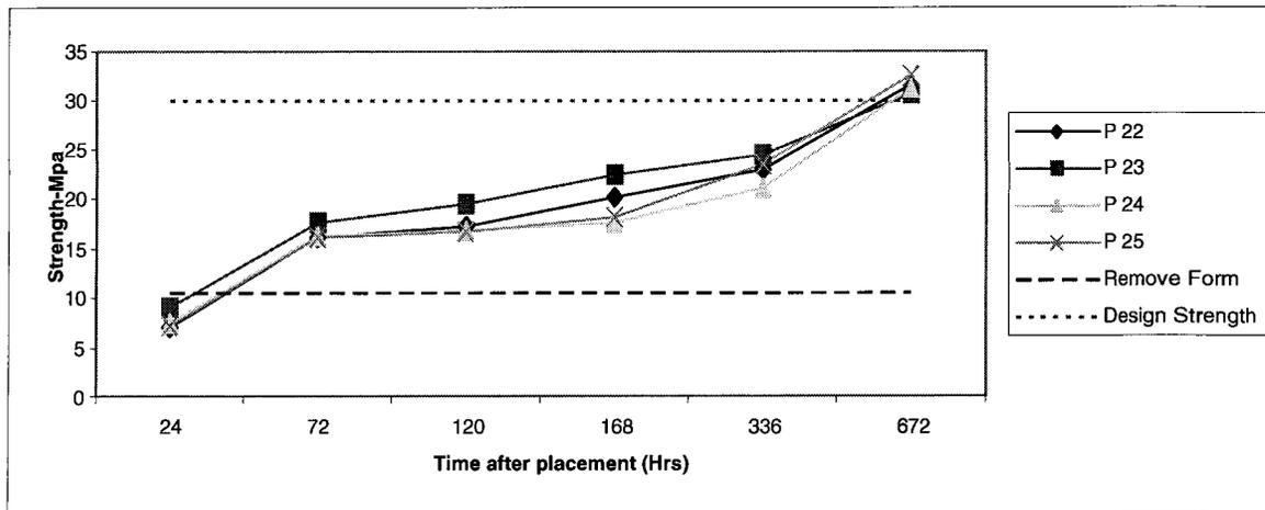
*Figure 4.14 Strength Development Curve of Building Grade Beam*
