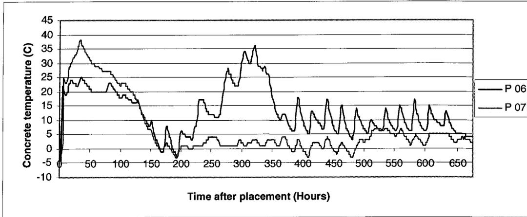
*Figure 4.5 Concrete Temperature Developments for the Vessel Base*
