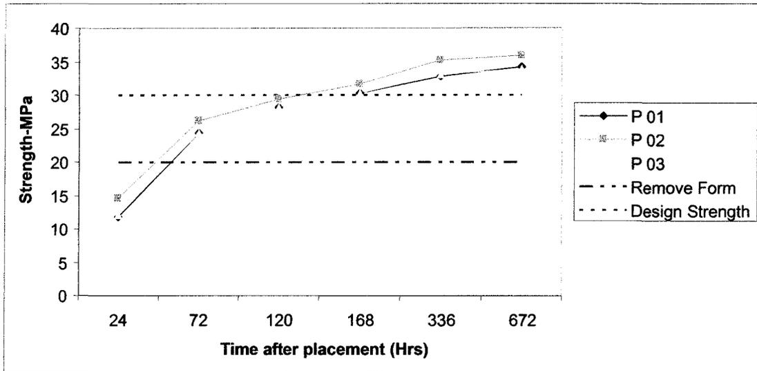
Figure 4.4 Strength Development Curve of Vessel Table Top I
