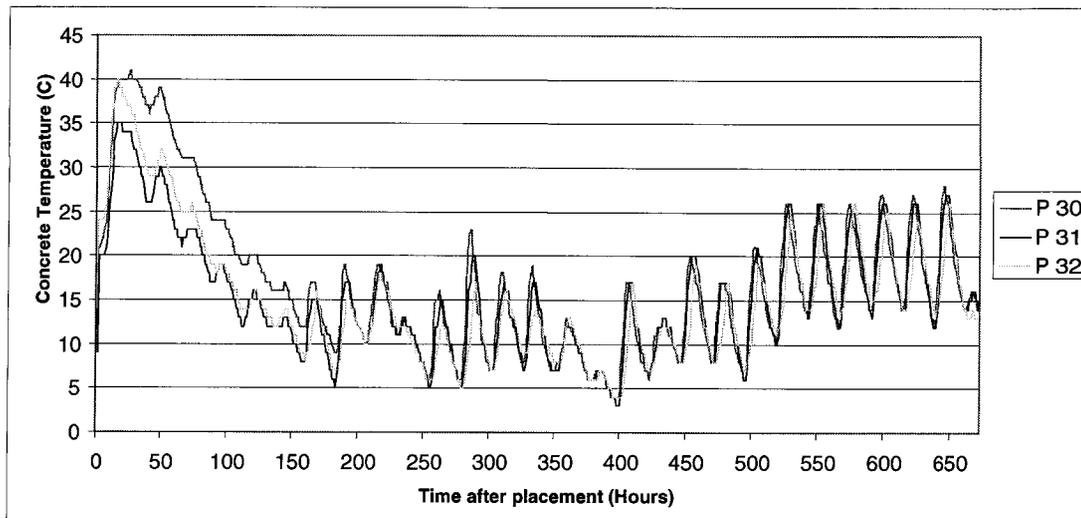
*Figure 4.17 Concrete Temperature Development for the Equipment Table Top*
