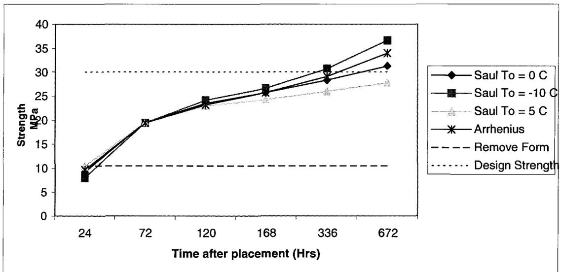
*Figure 5.4 Datum temperature sensitivity analysis of steel structure base*
