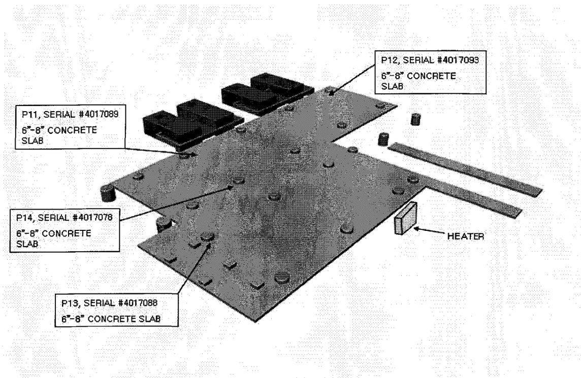
*Figure 3.2 Location V, logger and heater placement*
