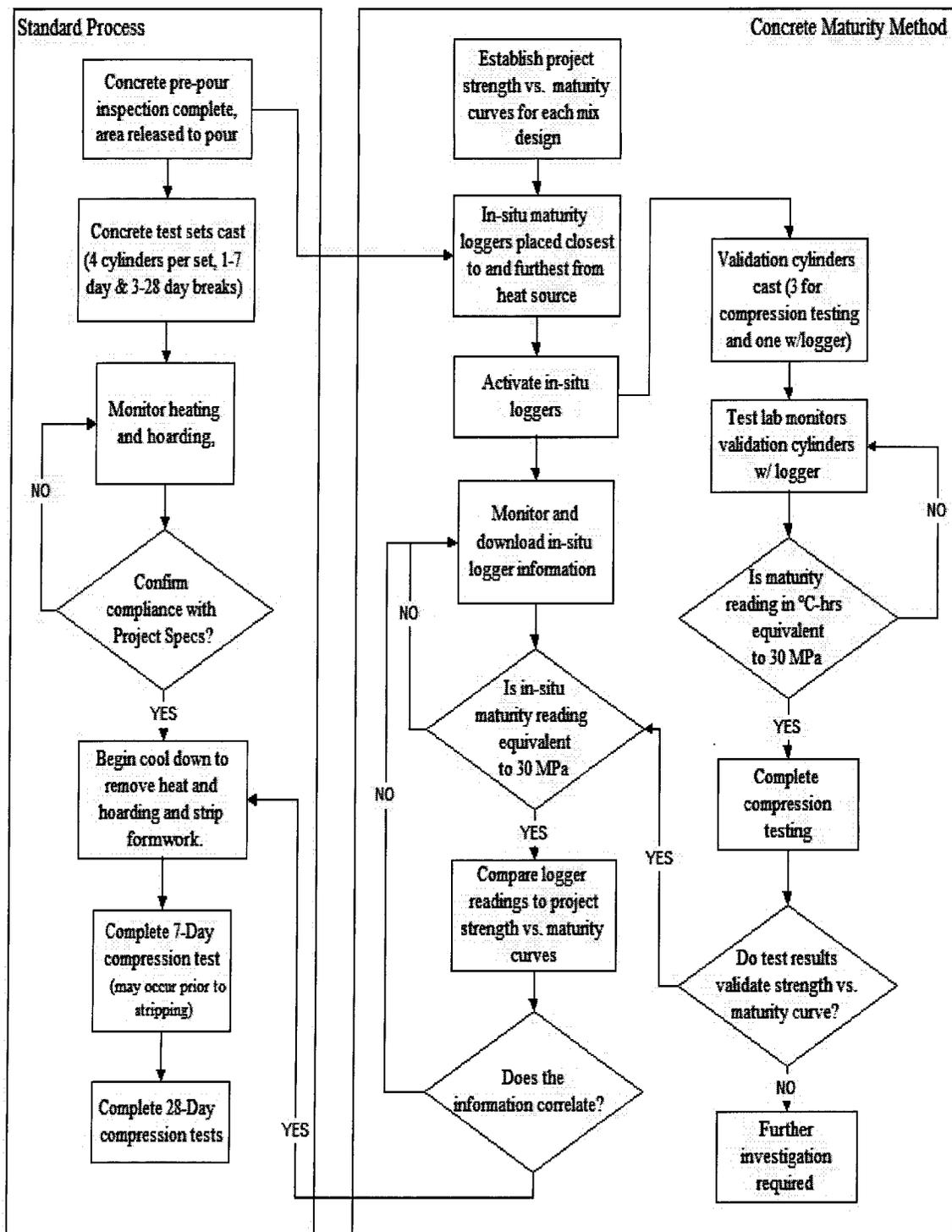
Figure 3.3 Process Flowchart
