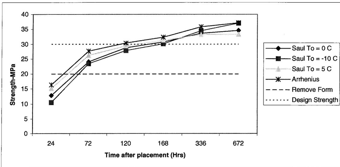
Figure 5.1 Datum temperature sensitivity analysis of vessel table top I
