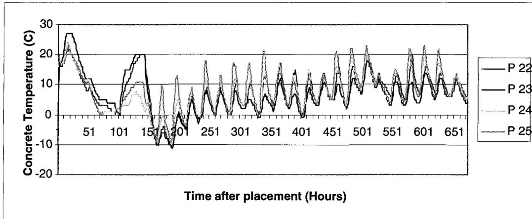
*Figure 4.13 Concrete Temperature Development for the Building Grade Beam*
