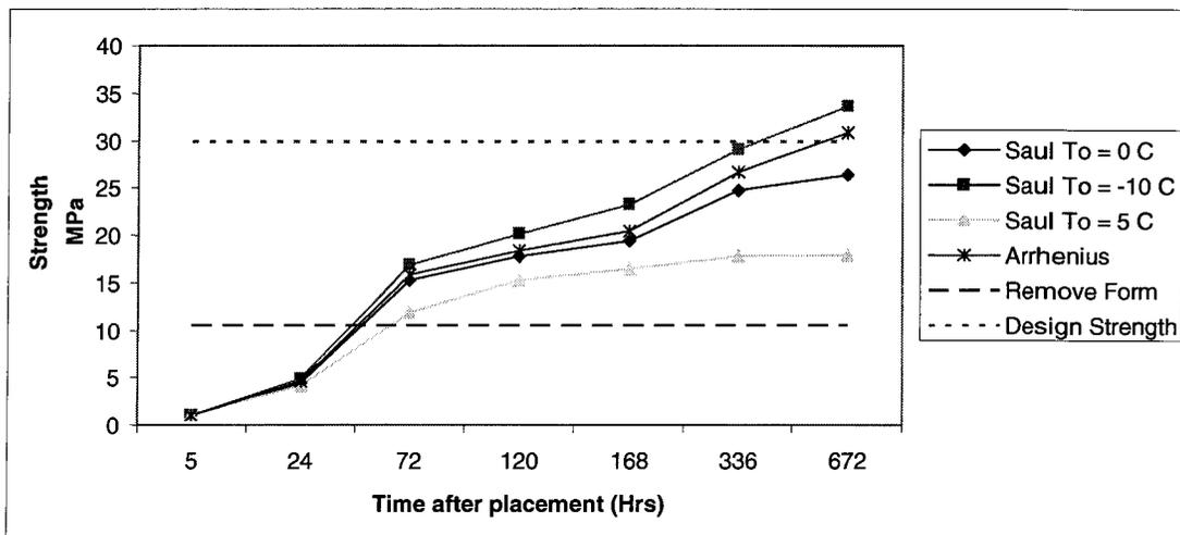
Figure 5.3 Datum temperature sensitivity analysis of substation paving slab
