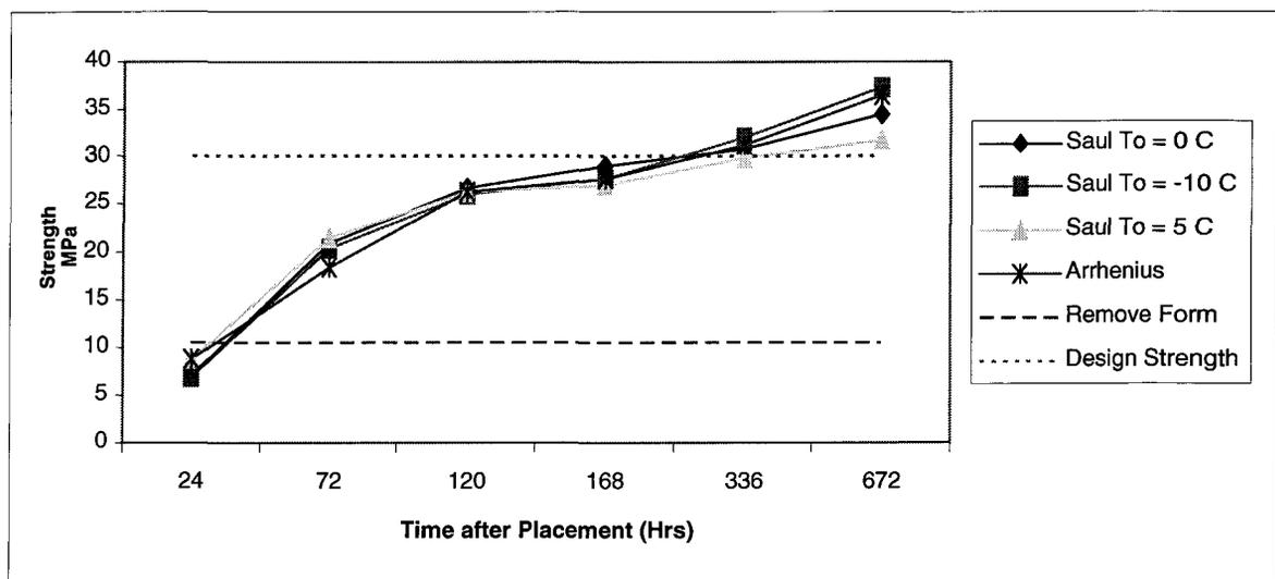
*Figure 5.2 Datum temperature sensitivity analysis of vessel base*
