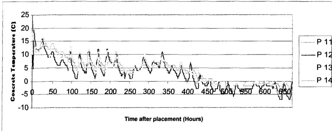
Figure 4.7 Concrete Temperature Developments for the Substation Paving Slab
