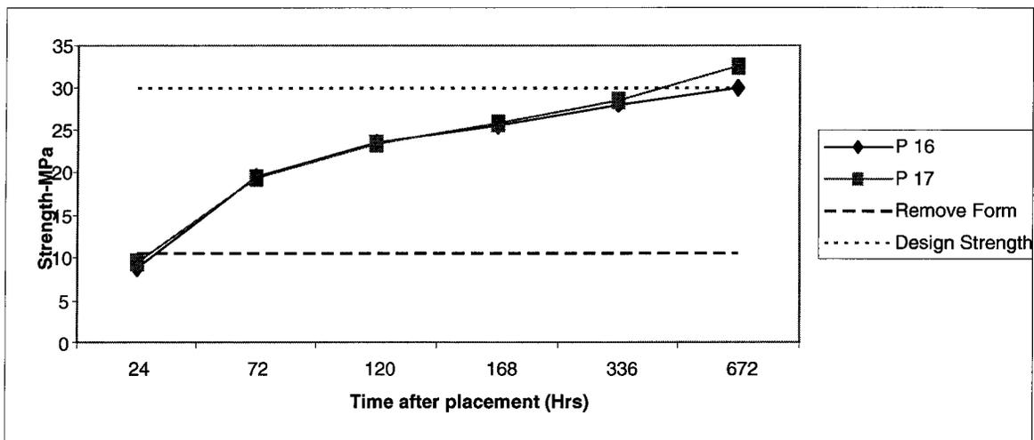
*Figure 4.10 Strength Development Curve of Steel Structure Base*
