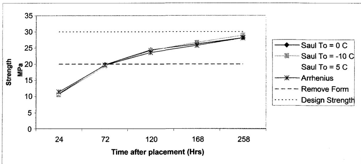
*Figure 5.7 Datum temperature sensitivity analysis of vessel table top II*
