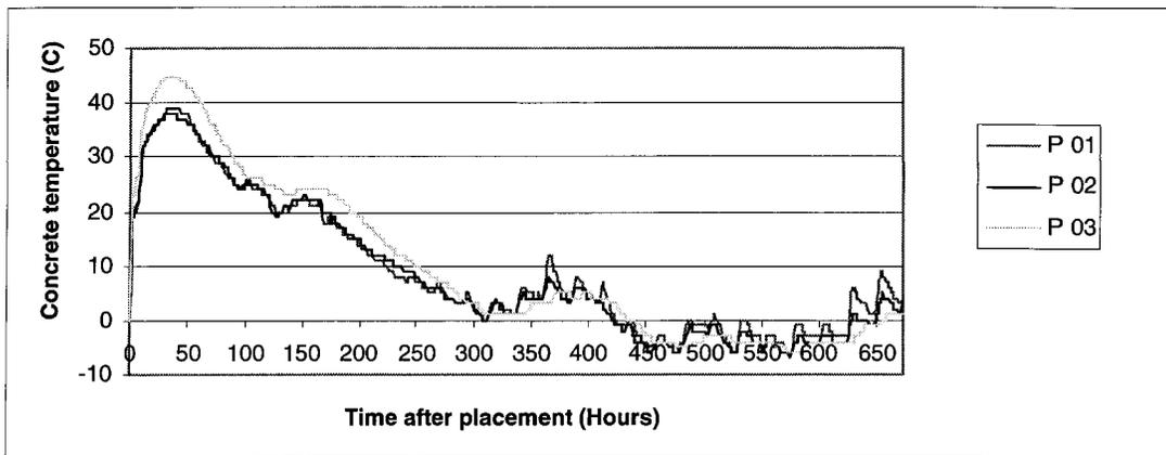
*Figure 4.3 Concrete Temperature Developments for Vessel Table Top I*
