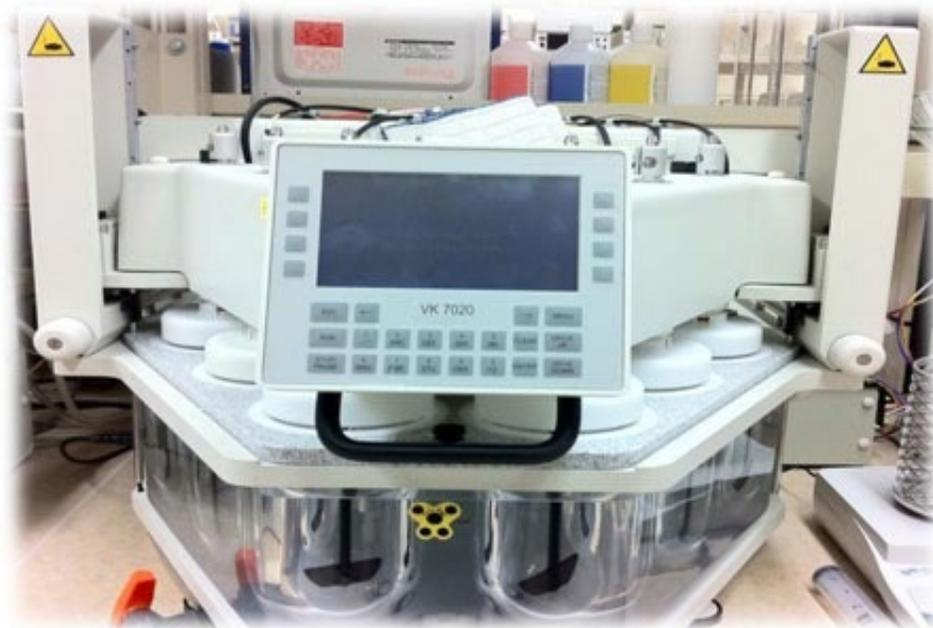
**Figure 1.3 - The USP Dissolution Apparatus 2**
