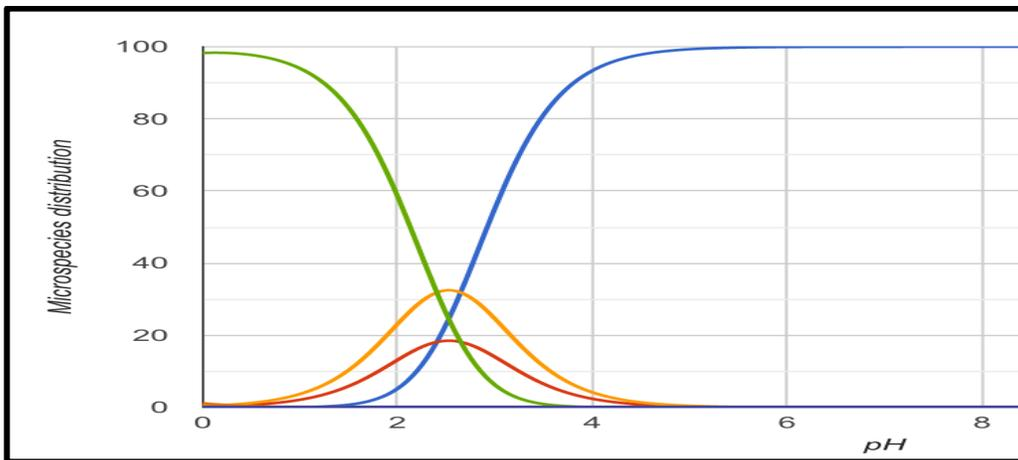
**Figure 2.1 – Microspecies distribution of ritonavir functional groups obtained from Chemicalize database, the green line represents the microspecies distribution of the functional groups with its strongest basic pKa.**
