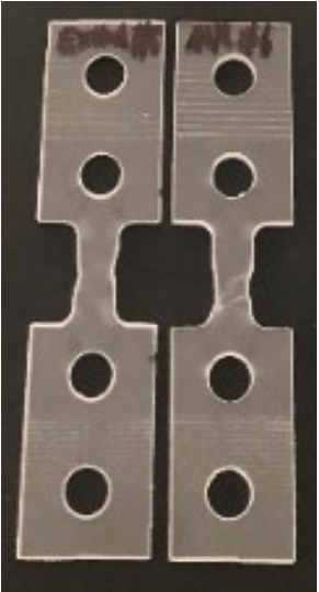
Figure 2-12 Gripping method two for extruded PETG dog-bone specimens with holes after the MR tests
