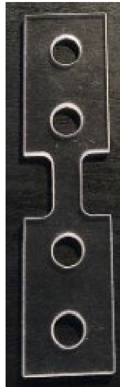
Figure 2-3 Sample water jetted PETG dog-bone specimen (with holes)
