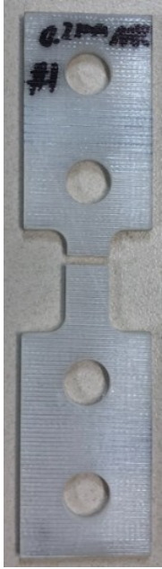
Figure 3-2 [90°] 3D printed PETG specimen with holes after MR tests using gripping method one
