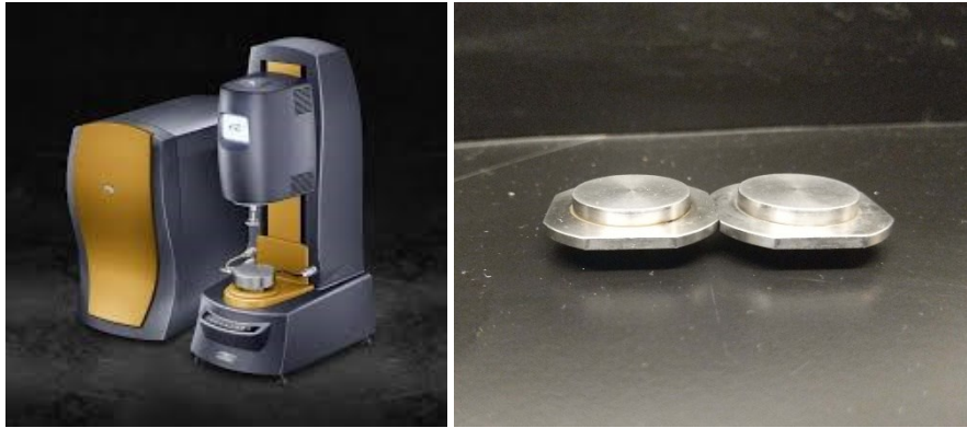
Figure 3.1 Discovery HR-1 Rheometer and Pelletier plates [31].
