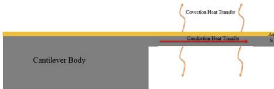
Figure 7.1. The heat transfer of a bi-material cantilever. There are two heat transfer mechanisms: first, conduction of heat inside the cantilever. Second, convection of heat to air around the cantilever by conduction mechanism.
