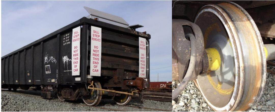
**Figure 2-2.** Photograph of the instrumented wheelsets (IWS) system installed on the Gondola railcar to collect the data used for this study. Wheatstone bridge strain gauges and connectors are covered in yellow epoxy coating, which is visible in the photograph (Images by Michael T. Hendry).
