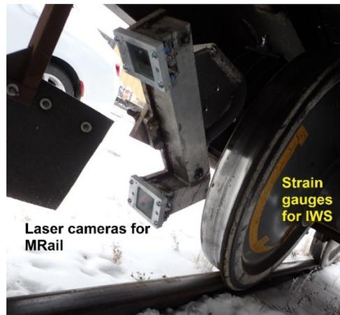
**Figure 5-1.** Photograph the train-mounted system with instrumented wheelset (IWS) and MRail systems installed on the Gondola railcar to collect the data used for this study (image credit: Michael T. Hendry).
