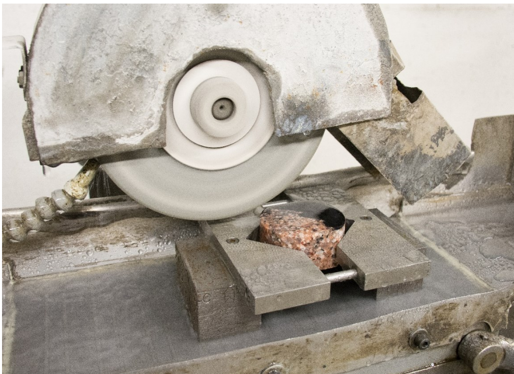
Figure B.4: Grinding a Lac du Bonnet granite sample using a surface grinder
