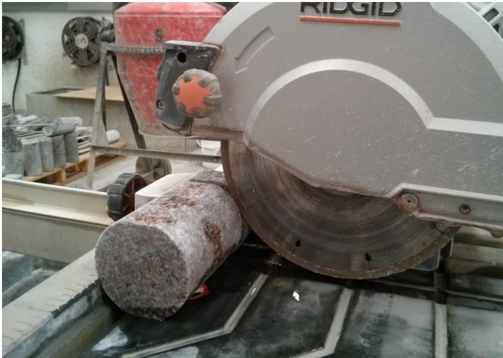
Figure B.3: Cutting a Lac du Bonnet granite core using a diamond saw
