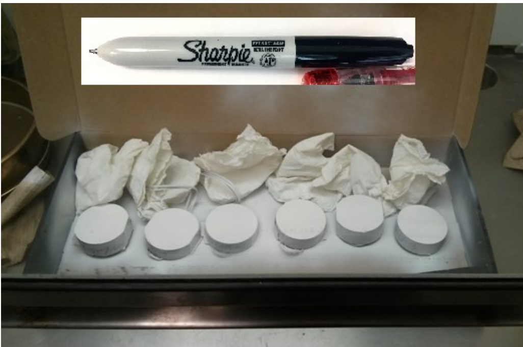
Figure B.6: Preparing a Lac du Bonnet granite sample for DIC measurement. A layer of white paint was sprayed first and then using an ultra fine sharpie black spackle pattern was made
