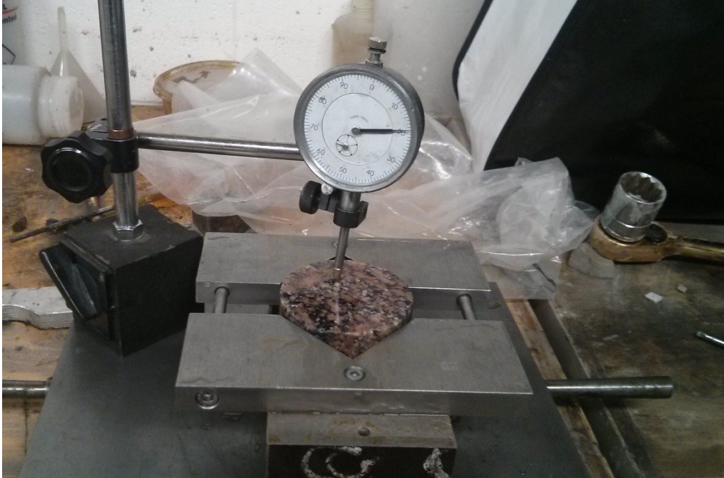
Figure B.5: Inspecting the flatness of a Lac du Bonnet granite sample
