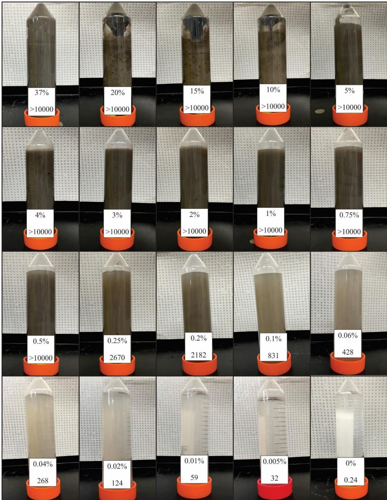
**Figure A.2.** MFT samples with different solid contents (First number in each picture shows the solid content of MFT suspension (wt. %), and the second one shows the turbidity value in NTU).
