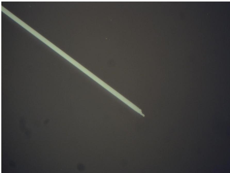
**Figure 3.13.** Capillary filling of 40 wt.% bitumen diluted in heptol (80:20) at  $t= 1.4$  s.
