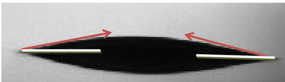
**Figure 3.18.** The measured bulk contact angle of 5 wt.% bitumen in heptol (80:20) on borofloat glass 0.3 s after the contact. The mean contact angle was about 12 degree.
