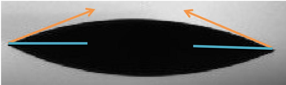
**Figure 3.17.** The measured bulk contact angle of 40 wt.% bitumen in heptol (80:20) on borofloat glass 0.3 s after the contact. The mean contact angle was about 26 degree.
