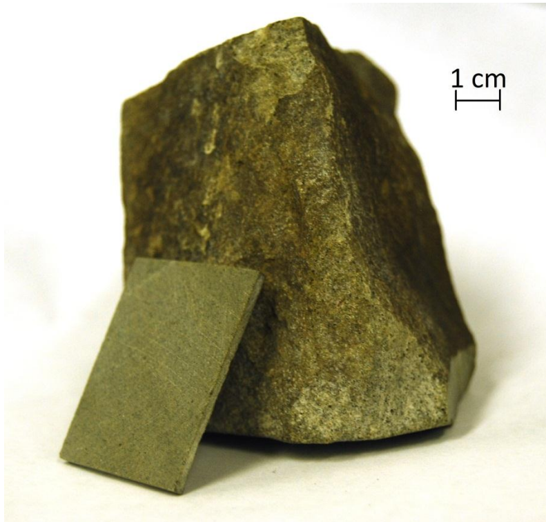
Figure 7. British Columbia natural zeolite and a liquid separation membrane.
