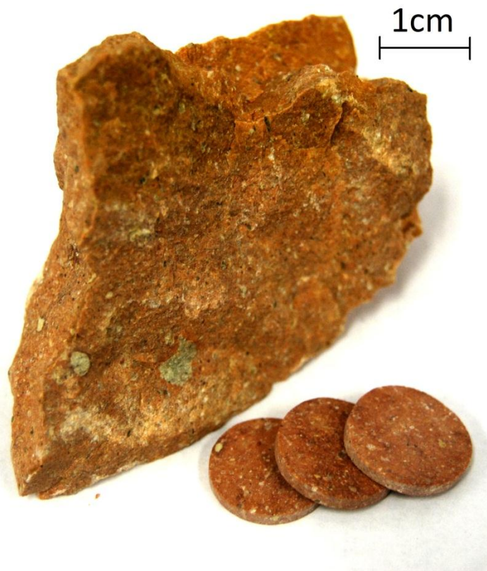
Figure 6. Castle Mountain natural zeolite and gas separation membranes.
