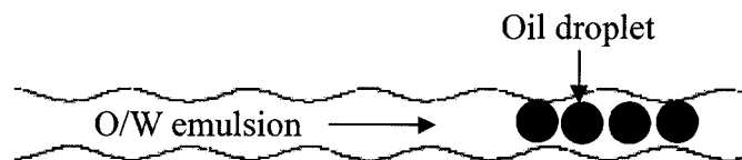
Figure 2.1 Piston-like flow in low aspect-ratio channel
