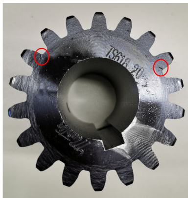
(a) Two nonadjacent tooth cracks (Scenario 1)
