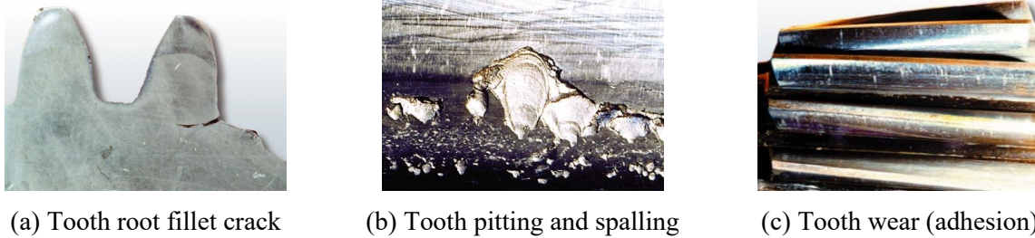
Fig. 1.5: Gear tooth fault modes [12]
