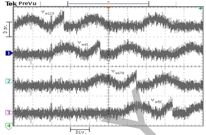
Fig. 11. Real-time synthesis of variable wind speed signals for the four groups of wind turbines.  $x$  axis: 10 s/div.,  $y$  axis: 5.65 m/s/div.
