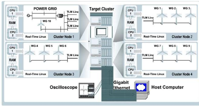
Fig. 10. Distribution of subsystems across the real-time simulator nodes [59].
