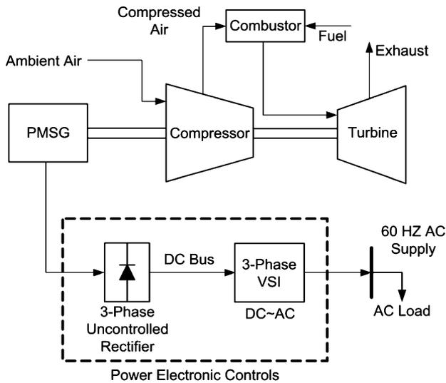
Fig. 3. Example A: Block diagram of the simulated  $\mu$ TG system.
