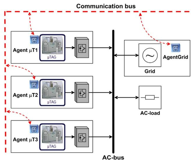
Fig. 5. Example B: Architecture of the multiagent system.
