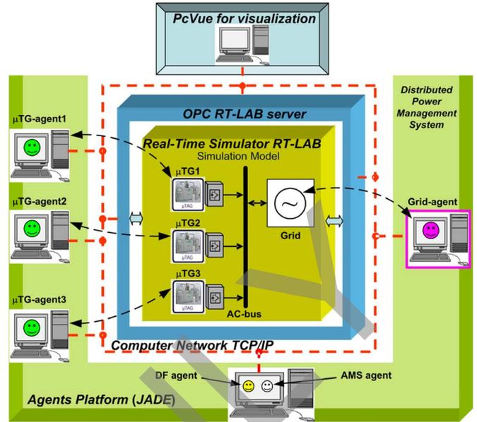
Fig. 7. Example B: Structure of the real-time simulation platform.
