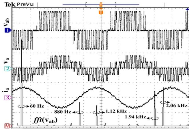
Fig. 13. Real-time trace of the interface converter line voltage, line-to-ground voltage, line current, and harmonic spectrum of line voltage.  $x$  axis: 0.4 ms/div,  $y$  axis:  $V_{ab}$  (1 kV/div.),  $V_a$  (1 kV/div.), and  $I_a$  (1 kA/div.).
