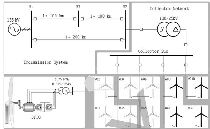
Fig. 9. Single-line diagram of the grid-connected wind farm [59].
