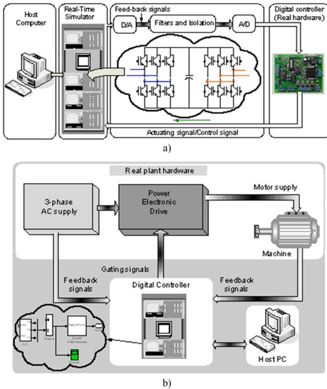
Fig. 1. Applications of real-time digital simulators. (a) Hardware-in-the-loop simulation. (b) Controller prototyping.
