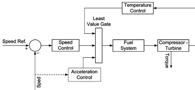
Fig. 2. Block diagram of a microturbine.
