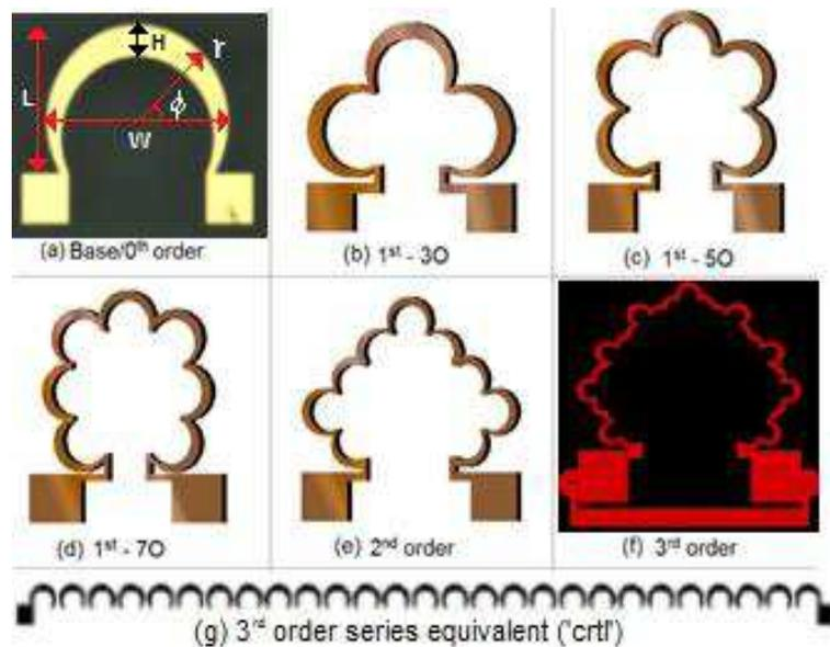
Figure 3.1: The (a) fabricated base inductor and dimensional definitions; the set of 1<sup>st</sup> order structures consisting of (b) 3 bases, (c) 5 bases, (d) 7 bases; (e) the 2<sup>nd</sup>-30 order fractal and (f) the 3<sup>rd</sup>-30 order simulated fractal; (g) an example of a control (ctrl) structure: shown is the 3<sup>rd</sup> order series equivalent.
