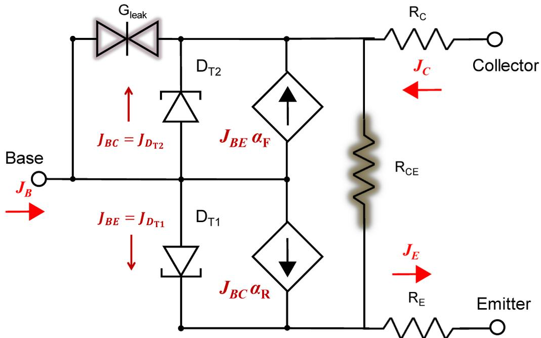
Figure 5.17: The TJT circuit model based on Ebers-Moll highlighting the major sources of non-idealities to be corrected. This includes  $G_{leak}$  which represents junction leakages at the base which are eventually collected at the collector.  $R_{CE}$  is the parasitic resistance between the emitter and collector. The diodes  $D_{T1}$  and  $D_{T2}$  represent the tunneling emitter and the referred-base-collector junctions, respectively.
