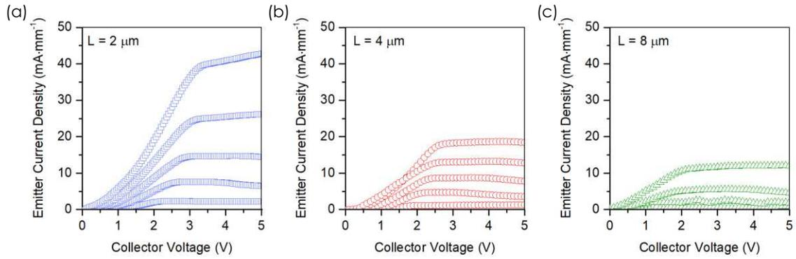
Figure 5.22: Measured family of emitter curves with improved isolation layer between n-ZnO and p-Si at non-overlapping region. The devices varied only in emitter-to-collector distances where (a)  $L_{EC} = 2 \mu\text{m}$ , (b)  $L_{EC} = 4 \mu\text{m}$  and (c)  $L_{EC} = 8 \mu\text{m}$ .  $V_{BE}$  was taken from 0 V to 5 V.
