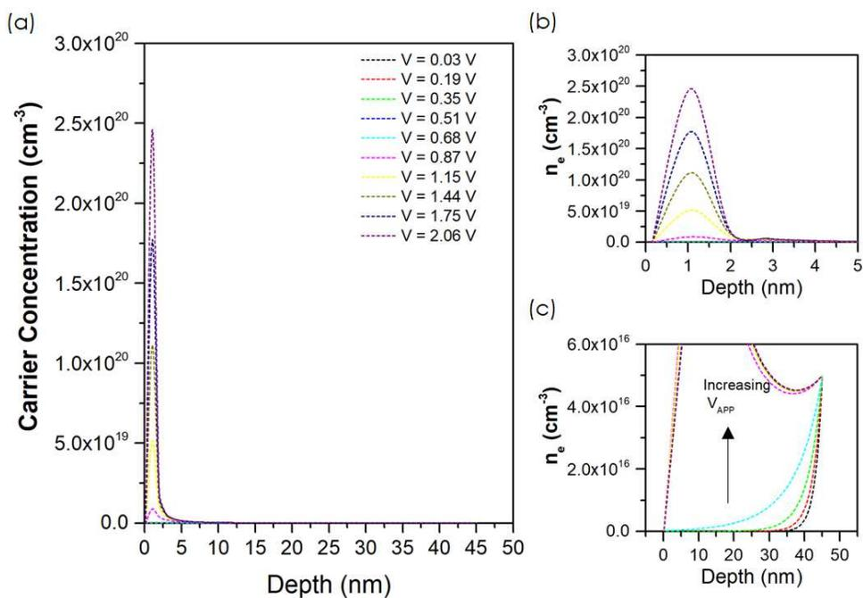
Figure 4.12: The 30 cycles HfO<sub>2</sub> electron distribution within the ZnO active layer at various applied biases  $V_{APP}$ . The overall distribution is shown in (a). A magnified view within the first 5 nm from the surface is shown in (b) at accumulation voltages and (c) is the overall distribution at voltages from depletion to the onset of accumulation. The centroid at 2V  $\sim$ 1.1 V for 30 cycles.
