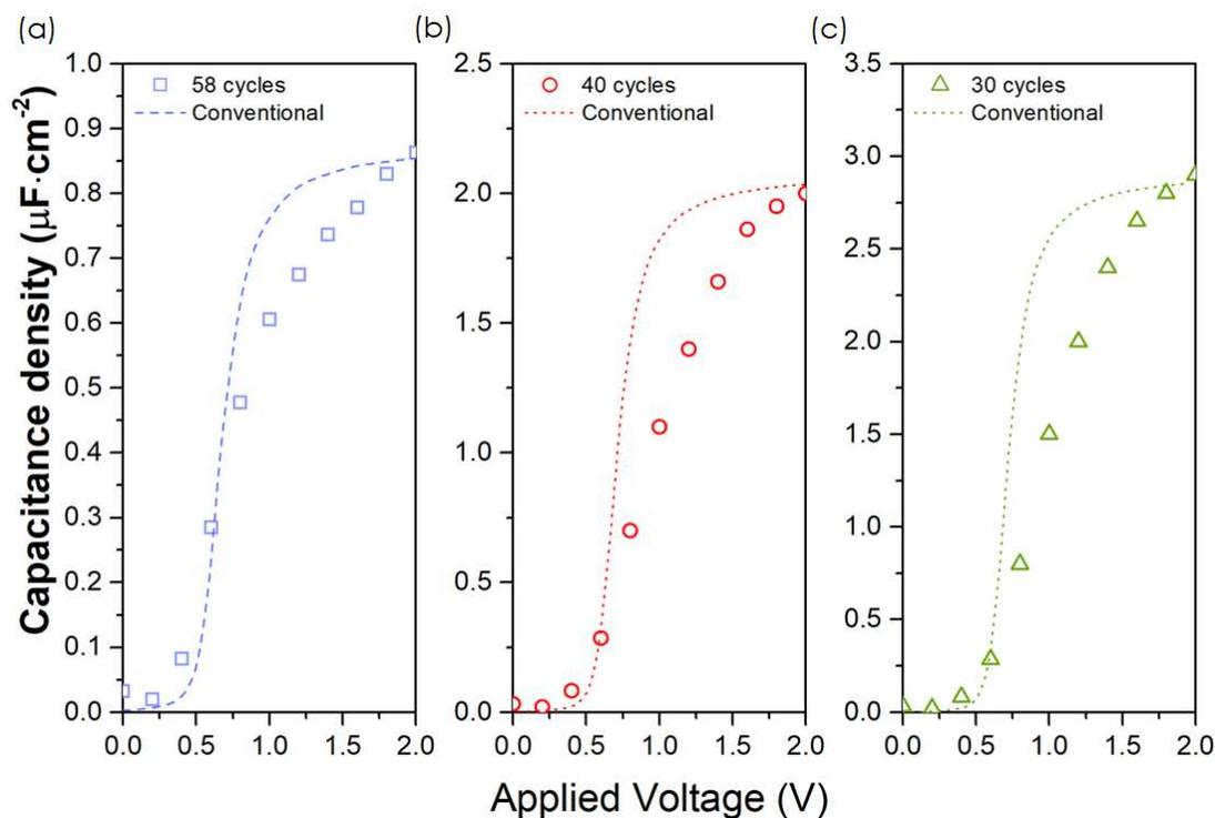
Figure 4.6: Comparison between measurement and conventional CV model for (a) 58 cycles of  $\text{HfO}_2$ ; (b) 40 cycles; and (c) 30 cycles. Overall, the fitting is demonstrably poor, even with the dielectric constant corrected matching  $C_{ACC}$ . The main issue comes with the difference in rate of depletion which cannot be explained by defects or parasitic components alone.
