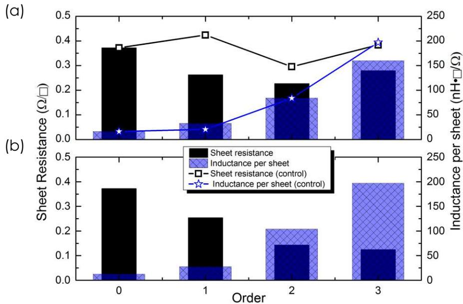
Figure 3.4: Measured sheet resistance and inductance per square analysis for each fractal order based on 1<sup>st</sup>-3<sup>o</sup> geometry extracted from (a) the original structures and its equivalent series layout (control); and, (b) with electrode width doubled from the original. Here, smaller black bars and larger checkered bars mean higher inductance per square area of resistance.
