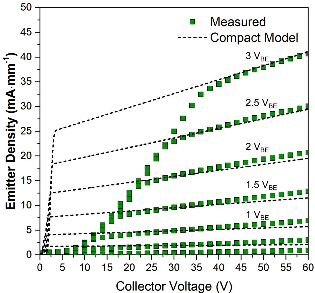
Figure 5.19: The simulated emitter family of curves based on the compact model compared to the  $L_{EC} = 10 \mu\text{m}$  TWT measured results. The goal of the compact model was to understand the behaviour of the TWT without the effects of recombination effects of  $G_{leak}$  such that  $V_{CE,SAT} = V_{BE}$ .
