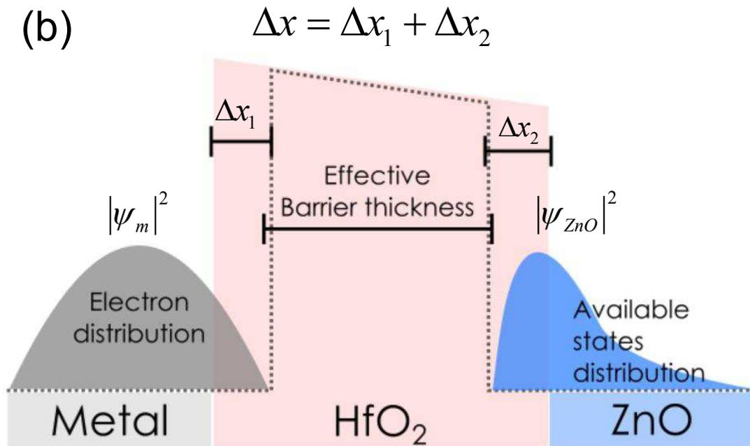
Figure 5.24: Alternative proposed interpretation of  $\Delta x$  and the effective barrier thickness. In (a) the ZnO electron wave function penetrates the barrier; and, (b) both the metal and the ZnO distribution penetrate the barrier by  $\Delta x_1$  and  $\Delta x_2$ . The sum of which gives  $\Delta x$ . These cases also lead to an effective thinning of the barrier.
