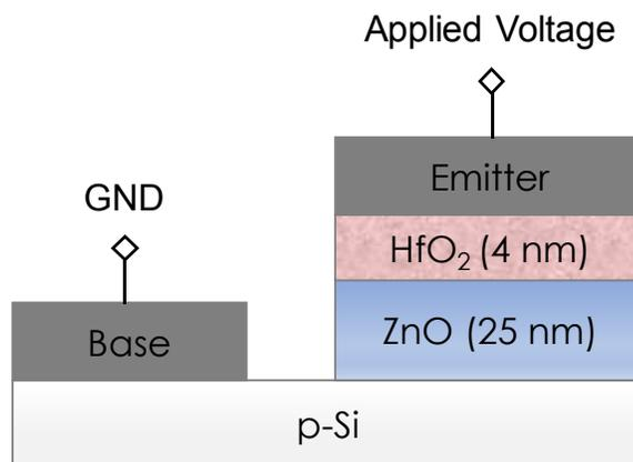
Figure 5.2: The MOSCAP structure simulated in Crosslight TCAD consisting of the active layer n-ZnO on top of a p-Si substrate that behaves as a supply for holes. A 4 nm HfO<sub>2</sub> is deposited on top of n-ZnO to form the barrier layer. The structure is completed with a base and emitter made of Al/Au.
