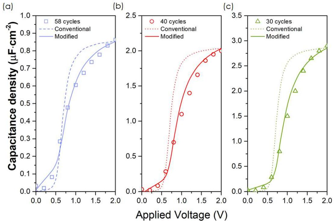
Figure 4.16: Comparison between measurement, conventional and modified CV model for (a) 58 cycles of  $\text{HfO}_2$ ; (b) 40 cycles; and (c) 30 cycles. The modified which takes into consideration both the geometrical thickness of the film and an exponentially-graded doping shows a much improved measured-model matching than the conventional CV extraction method.
