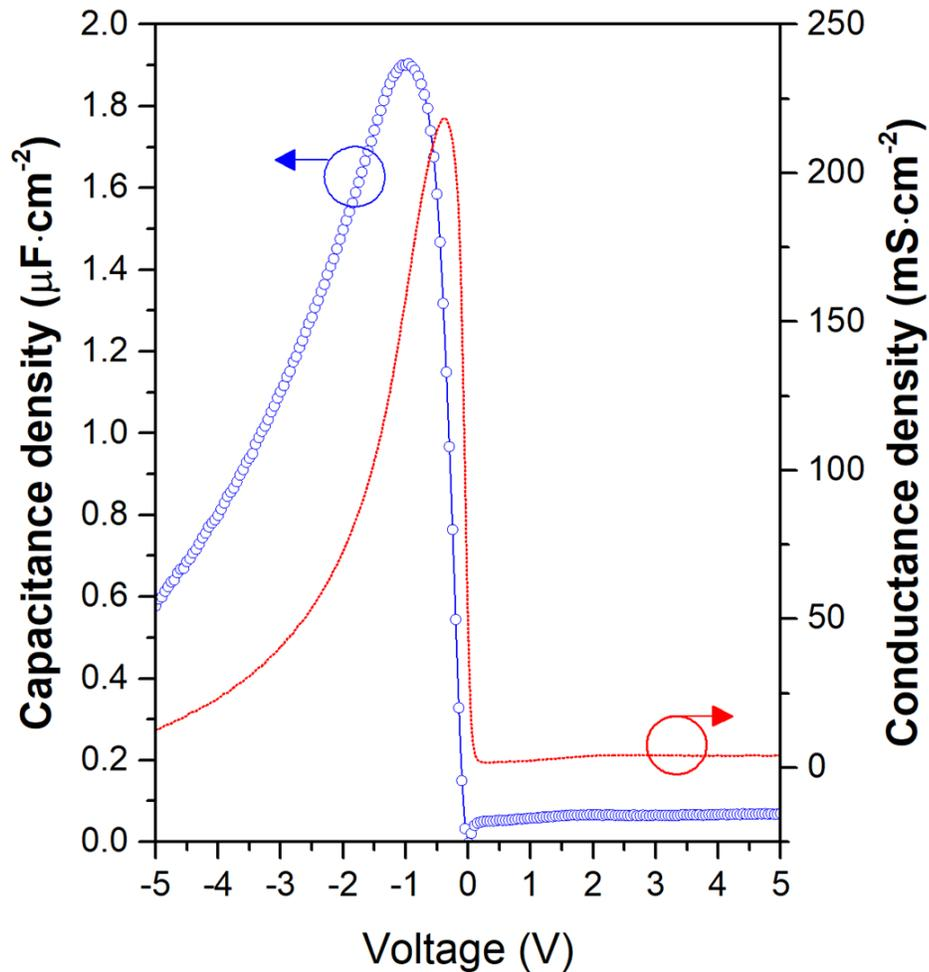
Figure 5.4: The HfO<sub>2</sub>/n-ZnO/p-Si MOSCAP showing the (a) measured CV which is consistent with proposed electrical operations. Furthermore, conductance curve reveals that control over charge is maintained beyond  $V_{EB} < 0$  V before leakage degrades the GV. At  $V_{EB} > 2$  V, there is no control of charge during accumulation.
