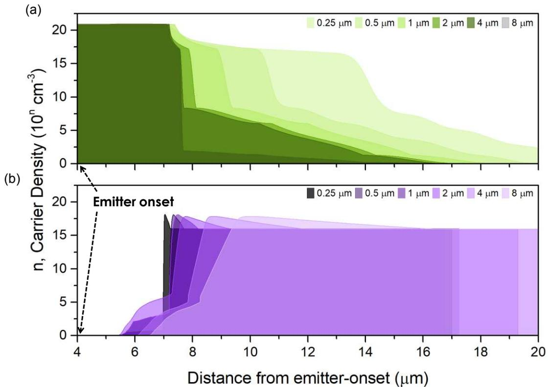
Figure 5.21: Simulated distribution of (a) holes and (b) electrons from the on-set of the emitter where the inversion channel is formed to the on-set of the collector for various emitter-collector distances  $L_{EC}$ . Some of the advantages of a scaled  $L_{EC}$  is a smaller recombination region and shorter resistance path.
