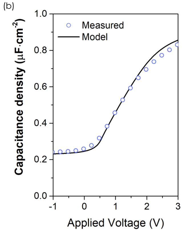
In this model, the non-uniform dopant distribution was also assumed. However, in stark contrast, the initial dopant profile for a TALD ZnO grown on an ohmic metal showed higher concentration at the metal surface than the insulator surface. It therefore suggests that there has to be a high doped region present at the ohmic-semiconductor interface in order to achieve a good ohmic contact. The distribution of the non-mobile ionic species (here, donors) are shown in Figure 4.20.
