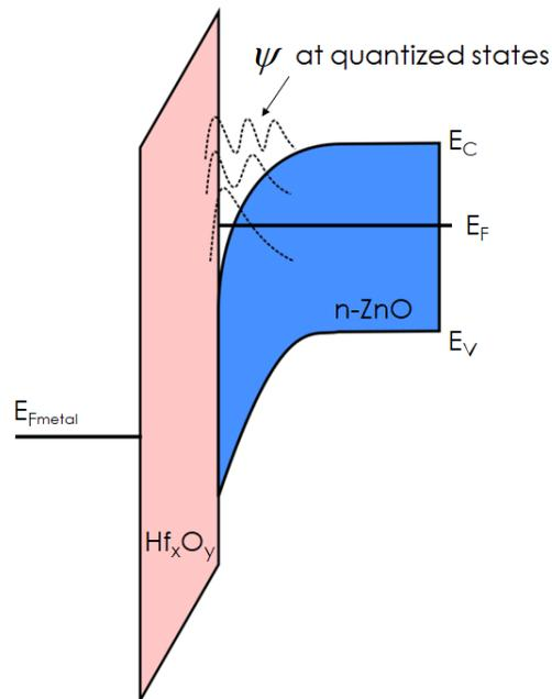
Figure 4.4: Band diagram of accumulation-biased MOSCAP. The wavefunction  $\psi$  exists in quantized energy states and dictate the distribution of carriers in the triangular well formed by the high barrier potential of the dielectric layer and surface band banding of ZnO.
