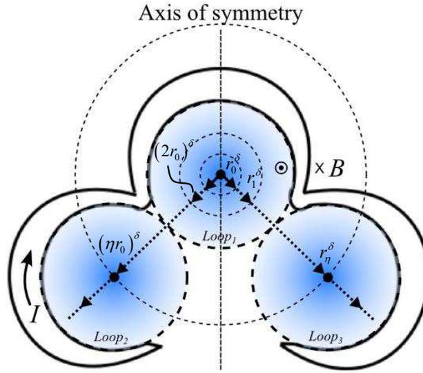
Figure 3.5: The essential geometrical parameters for the fractal dimensionality approach. Here, the 1<sup>st</sup>-3<sup>0</sup> order is used as an example.
