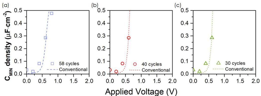
Figure 4.7: Deep depletion region comparison between measurement and conventional CV model for (a) 58 cycles of  $\text{HfO}_2$ ; (b) 40 cycles; and (c) 30 cycles. The absolute  $C_{MIN}$  of both measured and model data are in respectable agreement, implying that the defect level are not heavily influencing the deep depletion region.
