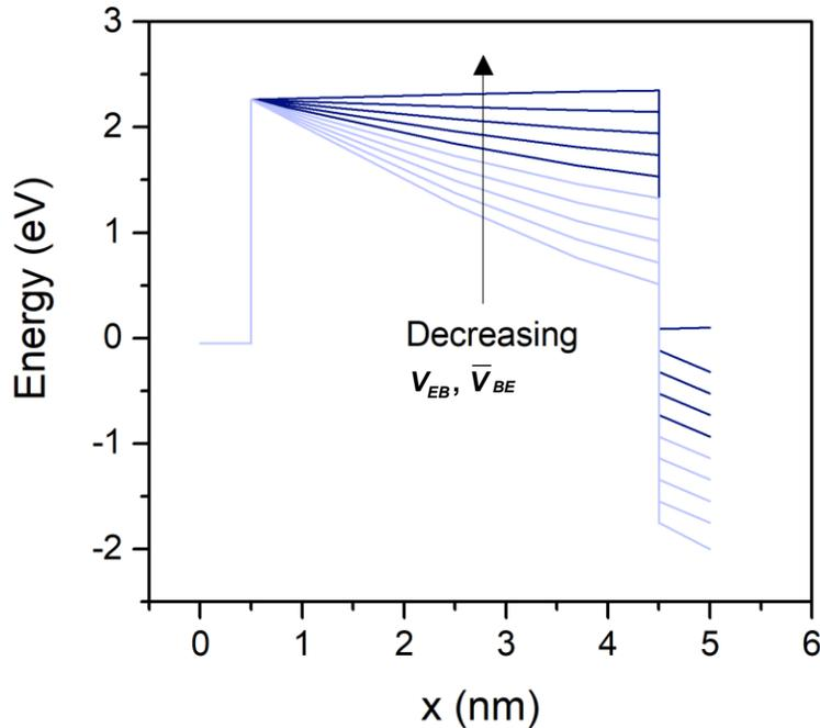
Figure 5.8: The dynamic band profile of the tunneling emitter as the applied voltage  $V_{EB}$  is varied from 0 V to 2 V. The barrier bends downward in response to the negative bias and the ZnO conduction band edge bends down as it gets further depleted.
