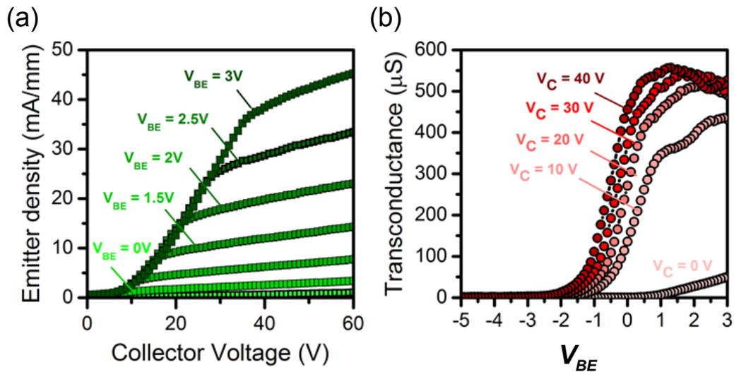
Figure 5.16: The measured TJT family curves in common-emitter mode from  $V_{BE} = 0V$  to  $3V$ ; (c) the transconductance of the TJT in the common-emitter mode.
