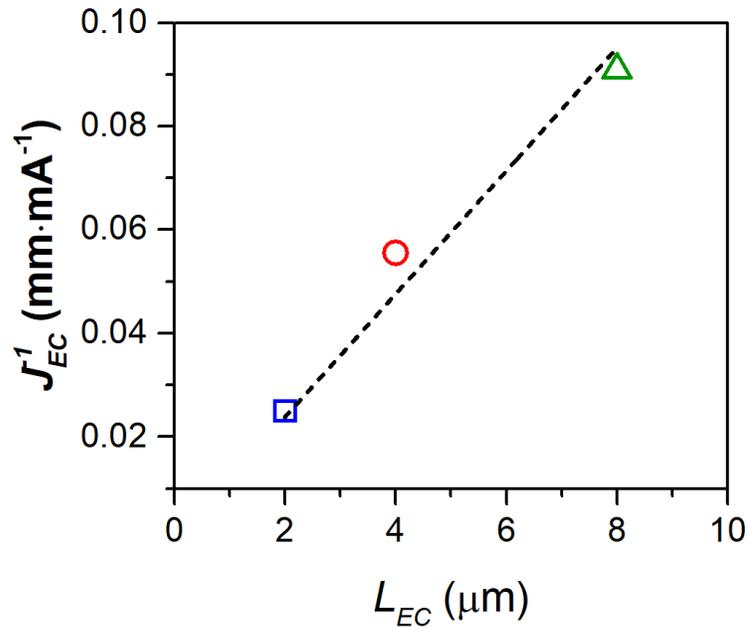
Figure 5.23: With an improved silicon nitride layer, current leakage from of the p-Si substrate to the collector electrode was minimized revealing increasing current densities as  $L_{EC}$  is shortened, suggesting that the device can improve its performance at scaled dimensions.
