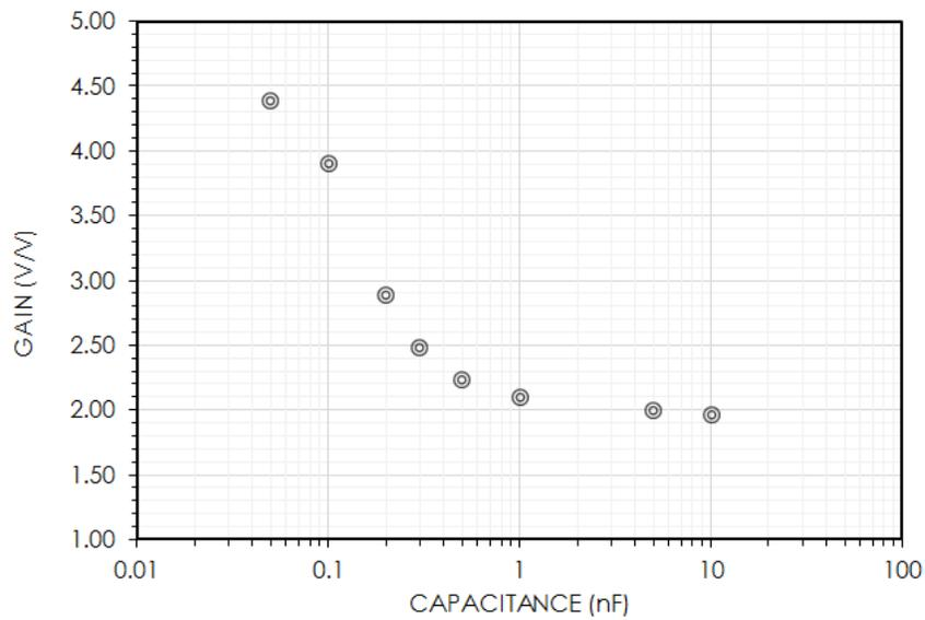
Figure 2.3: Gain response of an open-loop circuit with varying capacitance with a normalized scale. The cut-off frequency  $\sim 110$  MHz corresponded with the 1 nF turn-on of the varactor capacitance where the gain only minimally varied.
