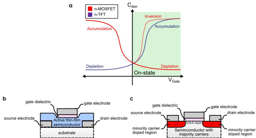
Figure 5.1: a) Shows the CV of n-TFT and n-MOSFET; b) the active thin-film of the TFT operated at accumulation region where the channel is made of majority carriers; and c) the n-MOSFET operates in the inversion region where the minority carrier doped regions at the source and drain supplies the channel with minority carriers.
