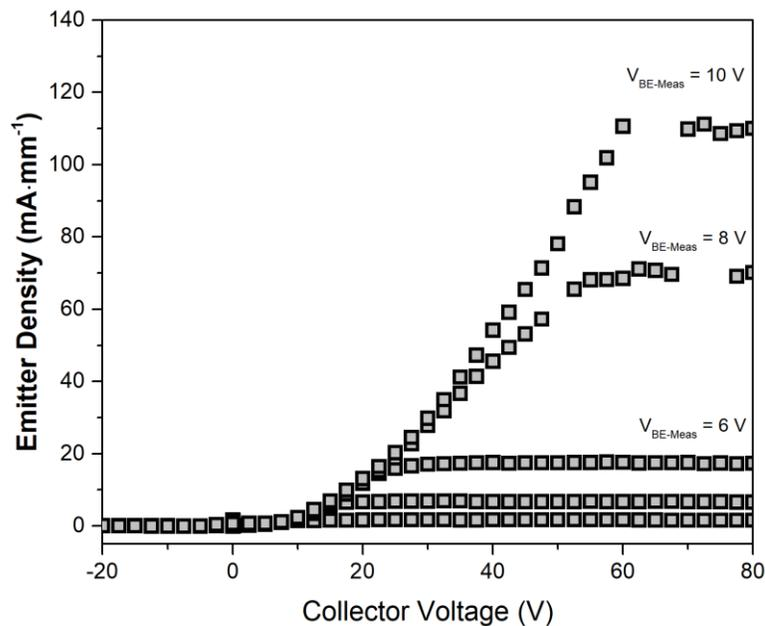
Figure 6.2: The TJT's current density can reach as high as  $115 \text{ mA}\cdot\text{mm}^{-1}$  when biased at a higher base voltage. In this case, the high density was reached at a bias of 10  $V_{BE}$  and 80  $V_{CE}$ . The TJT did not exhibit breakdown at these operating values and thus can be used for applications requiring power tolerances.
