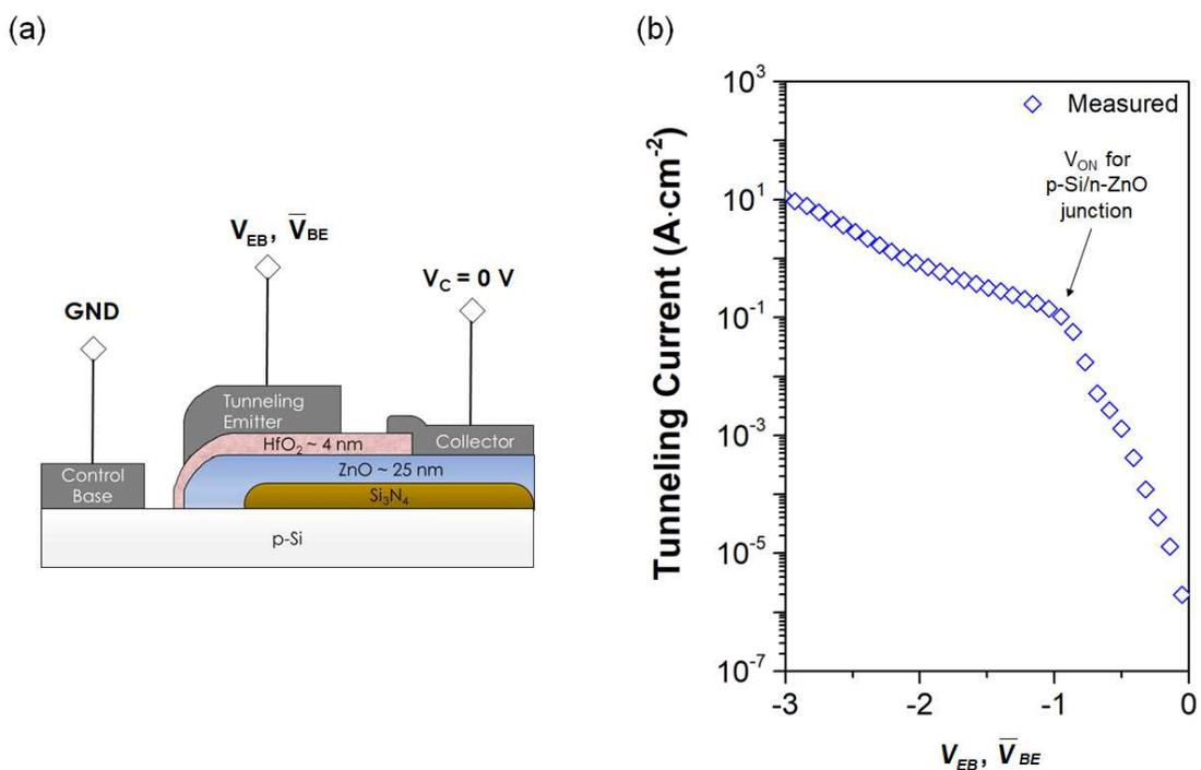
Figure 5.7: (a) The bias scheme of the TJT to measure the tunneling current at the emitter and, (b) the corresponding measured tunneling current density. The tunneling emitter was operating at inversion. The voltage where measured CV deviated from the expected CV is labeled as " $V_{ON}$ " and is the point where the p-Si/n-ZnO junction is turned on.
