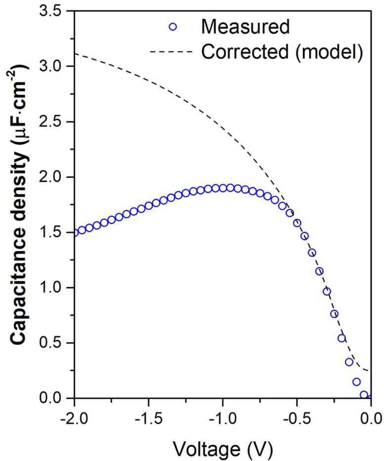
Figure 5.5: Simulated CV characteristics of the HfO<sub>2</sub>/n-ZnO/p-Si MOSCAP. Using the modified Schrödinger-Poisson equation, the model predicted the corrected inversion capacitance to be 3.1 μF·cm<sup>-2</sup>. The correction removed the additional junction effects contributing to the degradation of the inversion capacitance.
