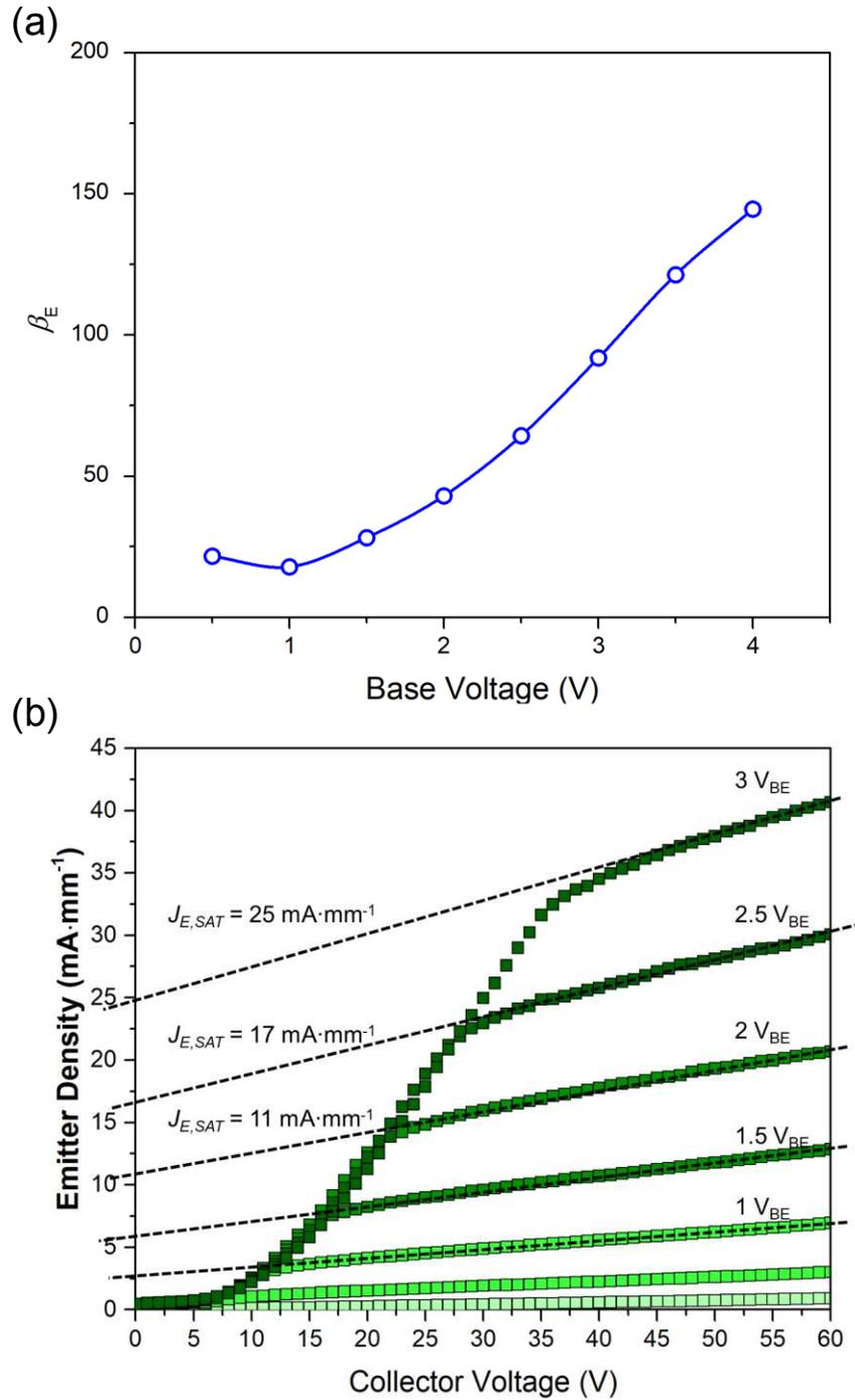
Figure 5.18: The TJT's (a) differential emitter gain for the TJT used to calculate  $\alpha_R$  for the compact model and (b) the estimated saturation current independent of junction leakages extrapolated from the slope of the measured current to when  $V_C = 0$  V.
