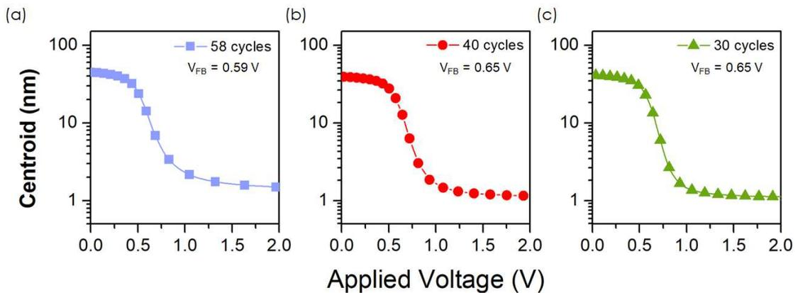
Figure 4.14: Calculated centroids for (a) 58 cycles of  $\text{HfO}_2$ ; (b) 40 cycles; and (c) 30 cycles. As the voltage increases, the electrons become more concentrated at the insulator-semiconductor interface but does not reach interface due to quantum effects. The centroid location increases as the field reverse pushing the electrons to the opposite direction.
