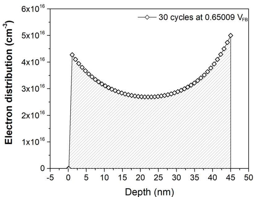
Figure 4.13: An example of the carrier distribution at flatband for 30 cycles HfO<sub>2</sub>. In a uniform distribution, the carriers also be uniform, but in an exponentially-graded dopant profile, a 'saddle-like' electron distribution is revealed.
