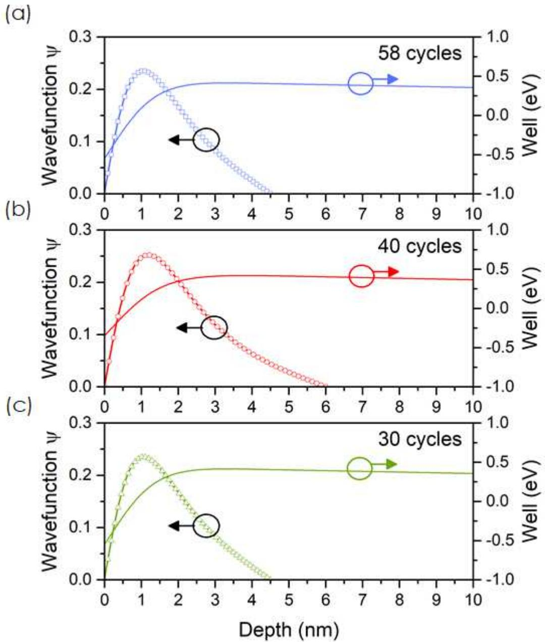
Figure 4.15: The lowest energy level wavefunction and the quantum well formed at 2V applied voltage for (a) 58 cycles of HfO<sub>2</sub>; (b) 40 cycles; and (c) 30 cycles measured data with respect to applied voltage at the gate. Due to the quantum well formed from the band-bending of the conduction can, the corresponding electrons are distributed according to the wavefunction.
