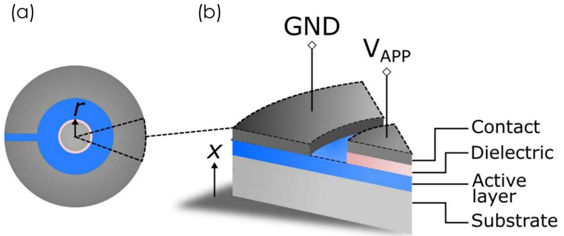
Figure 4.2: The structure of the circular MOSCAP (a) as in a top-down view; and a cross-section slice of showing its constituent layers. In this work, the substrate is sapphire, the active layer is a 30 nm of PEALD ZnO, followed by PEALD HfO<sub>2</sub> and Cr and the gate metal. The x direction tracks the thickness or depth of the structure, while the r tracks the lateral dimension.
