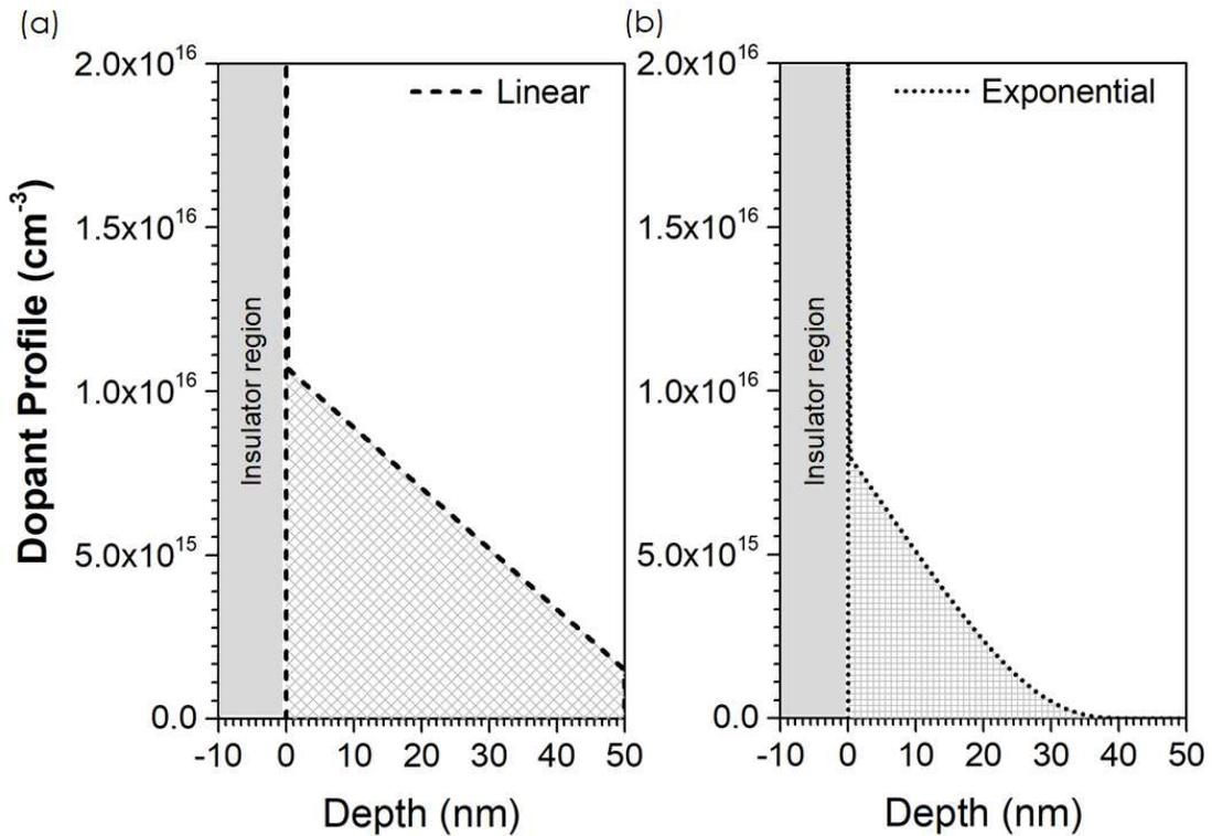
Figure 4.18: The revised dopant profile in PEALD ZnO that was distributed (a) linearly and (b) exponentially. Ultimately, exponentially-graded profile showed a better fit, but the important finding was that a highly doped surface relative to the rest of the film was necessary in order to resolve the CV behavior at lower voltages. The discontinuity  $x_1$  represents the edge of the doped surface and the onset of the film's body. This surface depth was tuned until an acceptable fit was achieved.
