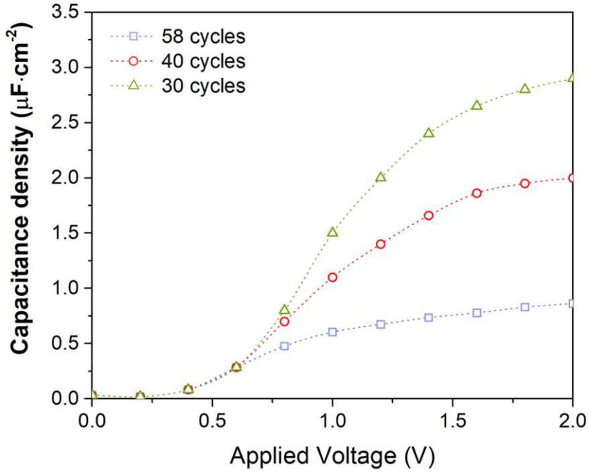
Figure 4.3: The CV measurement of 58, 40 and 30 cycles of HfO<sub>2</sub> measured from 0 V to 2 V at 10kHz frequency with an AC voltage of 30 mV<sub>AC</sub>. All three cycles were grown on the same layer with the bottom adjacent layer being 30 nm of PEALD ZnO.
