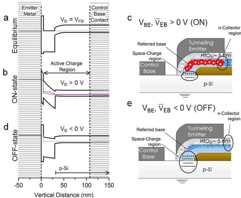
Figure 5.13: Band diagram elaborating on the of Al/ $\text{HfO}_2$ / $\text{ZnO}$ /p-Si tri-heterojunction during a) Equilibrium voltage where  $V_B = 0$  V; b) ON-state indicating the active charge region which determines the minimum film thickness required for a p-type carrier source; and c) the predicted carrier distributions showing the inversion layer or referred base; d) OFF-state and e) the almost fully depleted majority carriers of both ZnO and p-Si.
