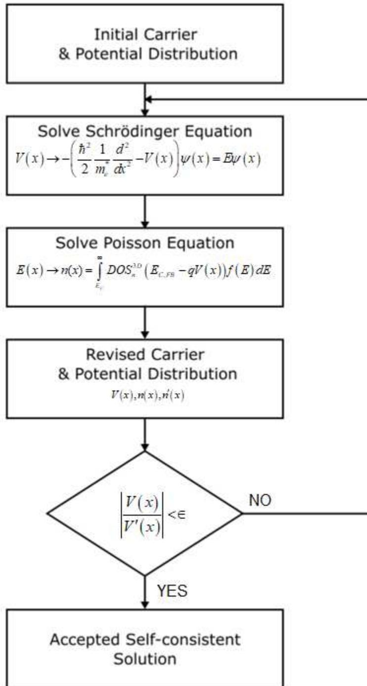
Figure 4.5: Schrödinger-Poisson self-consistent flow chart. Initial guesses are made for both initial carrier and potential distribution and calculated first with the Schrödinger equation. The solution is then applied to the Poisson-equation. The carrier and the potential solution are combined to give a revised solution. If the new potential correction is less than  $\epsilon$ , then the solution is accepted as self-consistent.
