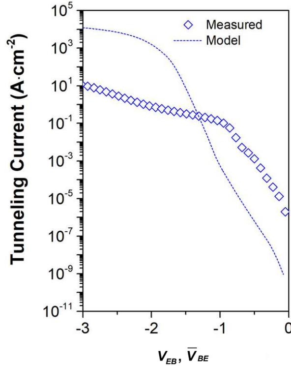
Figure 5.9: Tunneling current of the emitter was modeled using a Schrödinger-Poisson transfer matrix method. There is significant mismatch between measured and model at the calibration region (0V to -0.9 V) when considering a 4 nm barrier thickness (the physical barrier thickness of HfO<sub>2</sub> layer).
