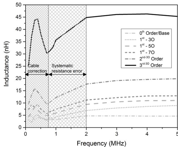
Figure 3.2: Raw inductance measurement of the loop inductor and its subsequent higher order fractal geometries using the Keithley 4200 SCS CVU.
