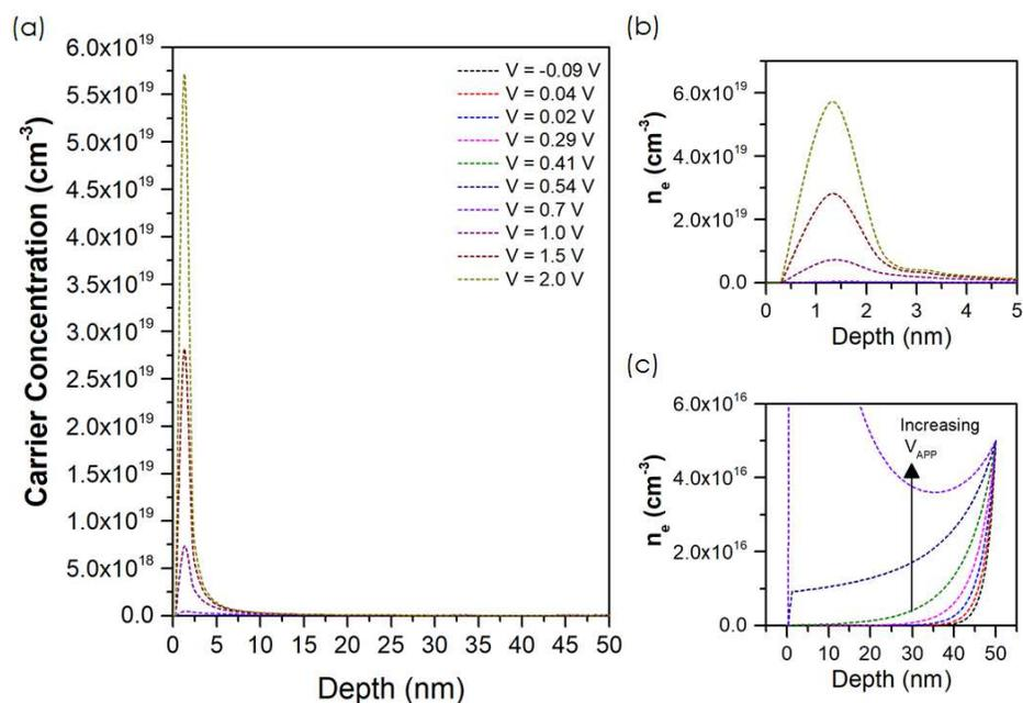
Figure 4.10: The 58 cycles HfO<sub>2</sub> electron distribution within the ZnO active layer at various applied biases  $V_{APP}$ . The overall distribution is shown in (a). A magnified view within the first 5 nm from the surface is shown in (b) at accumulation voltages and (c) is the overall distribution at voltages from depletion to the onset of accumulation. The centroid at 2V is  $\sim 1.5$  nm for 58 cycles.
