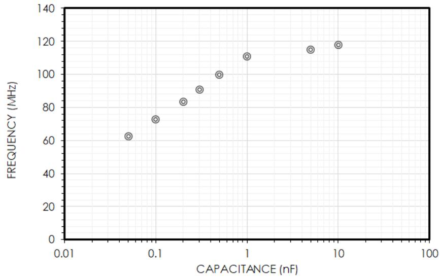
Figure 2.2: Frequency response of the open-loop circuit with varying capacitance. The frequency increases with capacitance due to critical coupling of the varactor diode as it approaches its turn-on voltage. At 1 pF, the varactor is nearly short-circuited leading to the saturation of the oscillation frequency.
