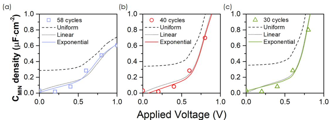
Figure 4.9: Using the modified model, various dopant profiles are simulated and compared with deep depletion region for (a) 58 cycles of  $\text{HfO}_2$ ; (b) 40 cycles; and (c) 30 cycles measured data. Uniform distribution failed to match  $C_{MIN}$ , but a revised linear and exponential model showed better fits including predicting the correct pivot voltage. The revised non-uniform distributions are discussed in Section 4.2.5.
