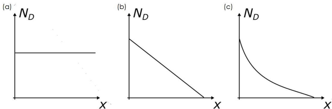
Figure 4.8: The dopant profile considered in this work include (a) uniform, which is the most common assumption, and the non-uniform profiles which are distributed (b) linearly and (c) exponentially. For the revised model, non-uniform distribution had to be considered in order to predict the CV behavior below 0.6V.
