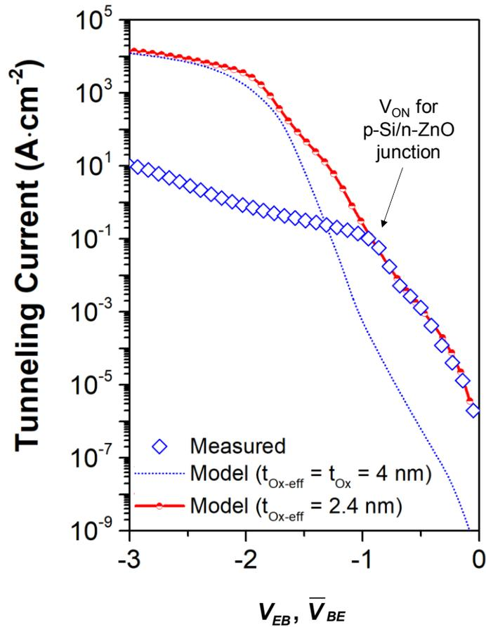
Figure 5.12: The revised model that compensates  $\Delta x$  by effective thinning of the barrier compared to the measured data and the previous models. With the compensation, the revised model provided a strong match with the calibration region. The model also predicts the tunneling current density at voltages below -0.9 V where the current and capacitance began to degrade. At 3 V, the current density reaches 10<sup>4</sup> mA·mm<sup>-1</sup>.
