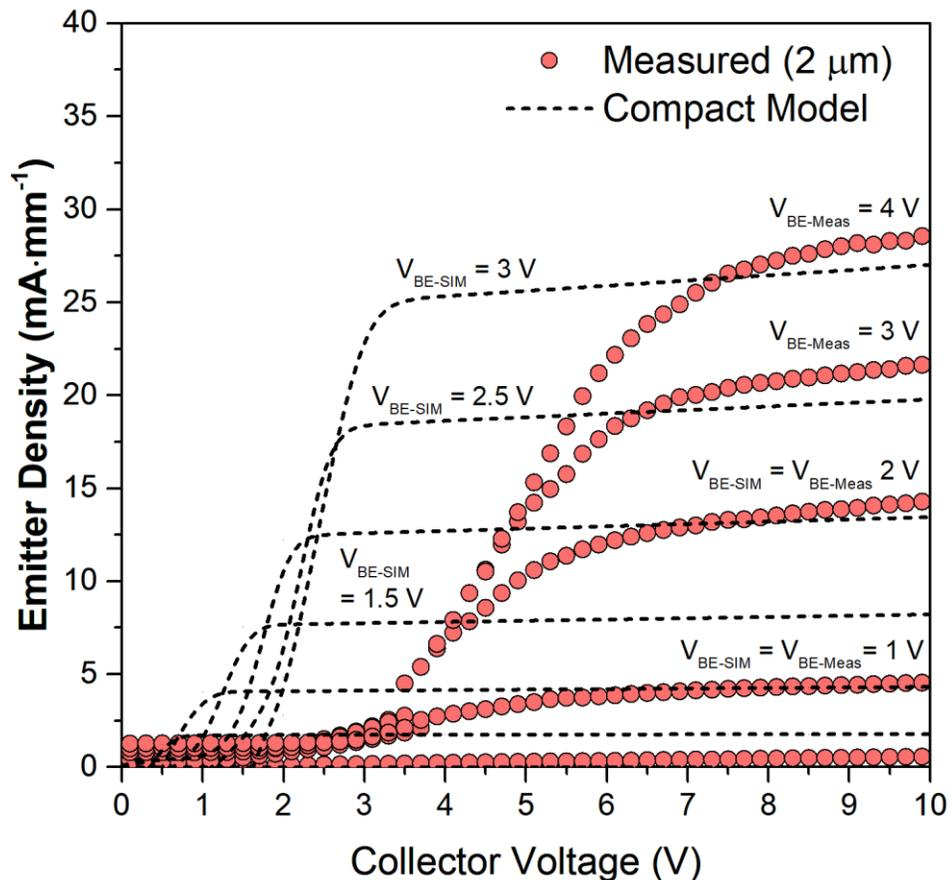
Figure 5.20: The measured results for a  $L_{EC} = 2 \mu\text{m}$  TJT with the compact model. Reducing the emitter to collector distance reduced both  $R_{EC}$  and the current lost due to recombination. As  $V_{BE}$  increases, the measured data revealed a lower transconductance than the predictions of the compact model, indicating that additional some degradation in current at higher base-emitter voltages.
