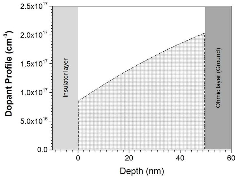
Figure 4.20: The dopant profile which yielded the best fit for the TALD ZnO grown ohmic substrate MOSCAP. At the Ohmic edge, the TALD ZnO film had higher dopant concentration than the insulator edge.
