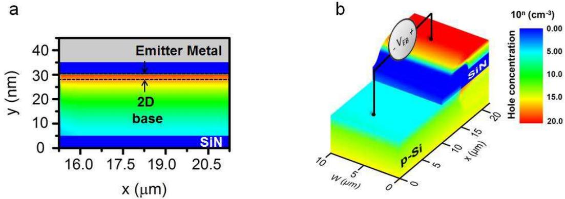
Figure 5.3: The distribution of holes at the a)  $\text{HfO}_2/\text{ZnO}$  region isolated from the p-Si holes source showing lateral uniformity and reaching hole concentration of up to  $10^{20} \text{ cm}^{-3}$  at the 2D referred base; b) the hole distribution of the full device from the onset of the p-Si control base to the edge of collector contact biased at  $V_{EB} = -5\text{V}$ .
