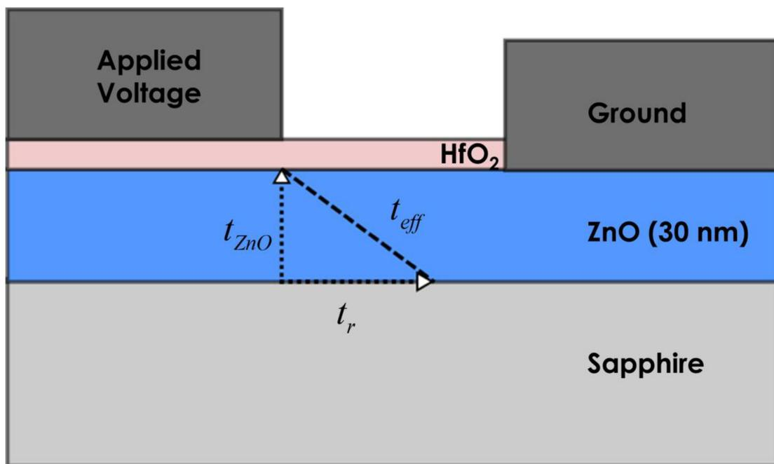
Figure 4.17: The geometrical interpretation of  $t_{eff}$ . The effective thickness for cases exceeded the actual thickness of the film. However, since the field as both a parallel  $t_z$  and a perpendicular  $t_r$  component,  $t_{eff}$  is interpreted as the Pythagoras sum of these two components.
