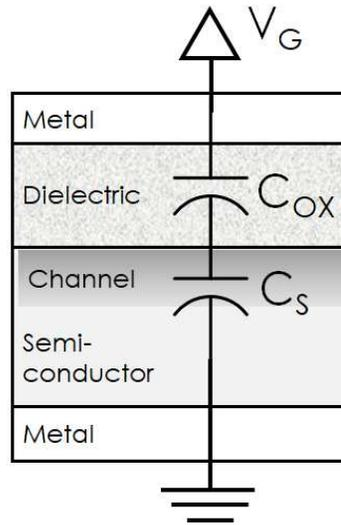
Figure 4.1: Equivalent circuit model of a MOSCAP containing two capacitors in series:  $C_{OX}$  which represents the capacitance arising for the insulator and is constant throughout the voltage range, and  $C_S$  representing the channel capacitance which does vary with the gate voltage  $V_G$ .
