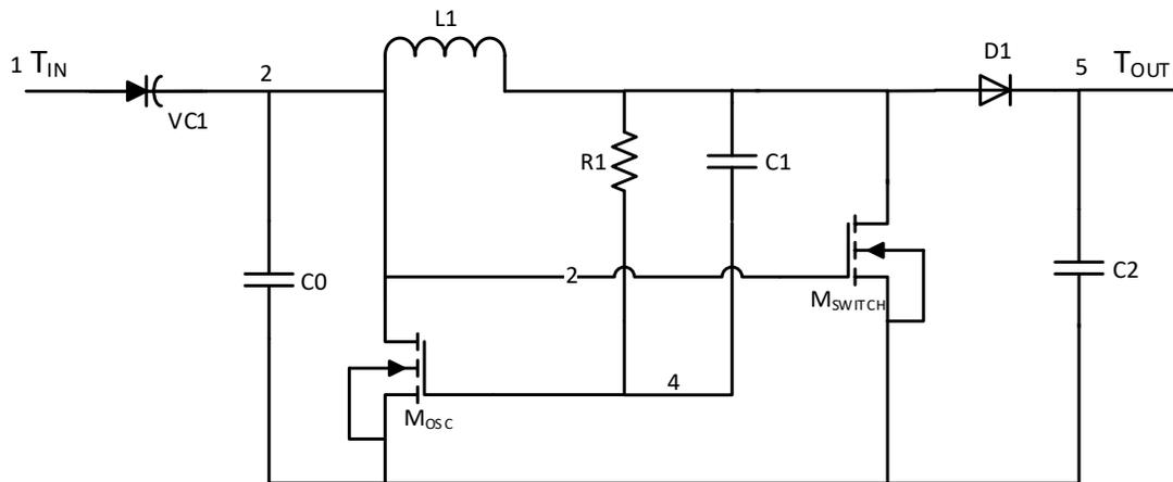
Figure 2.1: Proposed open-loop circuit schematic of a gain-varying self-oscillating boost converter. The inductive component  $L1$  and the transistors  $M_{OSC}$  and  $M_{SWITCH}$  are of particular interest for realizing circuit using thin-film components.
