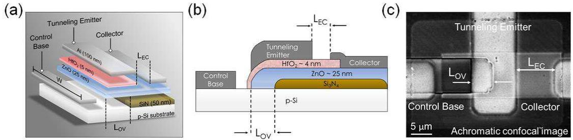
Figure 5.6: Overview of the thin tunneling junction transistor (TJT) based on p-Si/n-ZnO/HfO<sub>2</sub> tri-heterojunction: a) the fabrication process layers beginning from a bare p-Si substrate to the final metal layer; b) cross-section of a completed device along with the key terminals including the control base, tunneling emitter and collector; c) achromatic confocal microscopic top-view of a sample completed device;  $L_{OV} = 5 \mu\text{m}$ ,  $L_{EC} = 10 \mu\text{m}$ .
