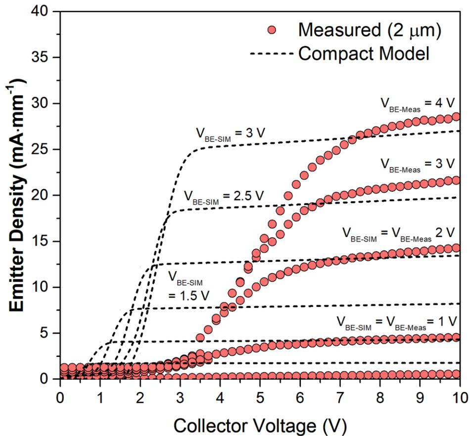
Figure 5.20: The measured results for a  $L_{EC} = 2 \mu\text{m}$  TJT with the compact model. Reducing the emitter to collector distance reduced both  $R_{EC}$  and the current lost due to recombination. As  $V_{BE}$  increases, the measured data revealed a lower transconductance than the predictions of the compact model, indicating that additional some degradation in current at higher base-emitter voltages.
