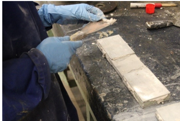
Figure 3-4: ECC coupon preparation - gluing aluminum plates
