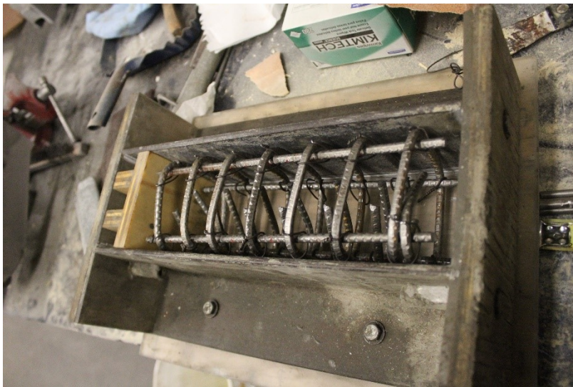
Figure 4-17: Steel cage of ECC-1.5%
