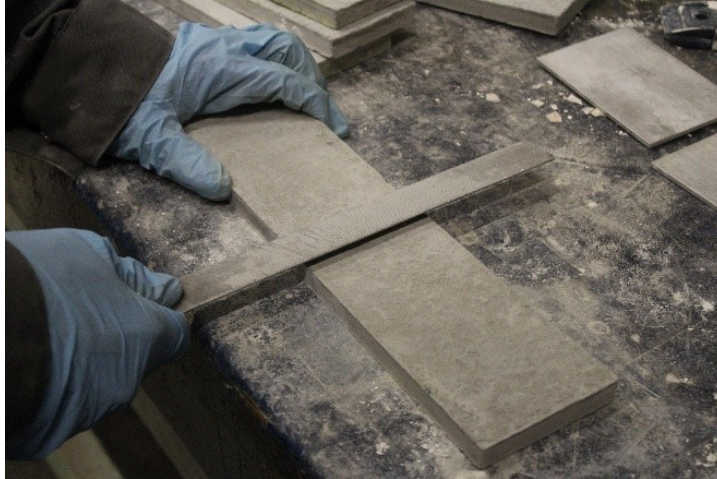
Figure 3-3: ECC coupon preparation - surface grinding
