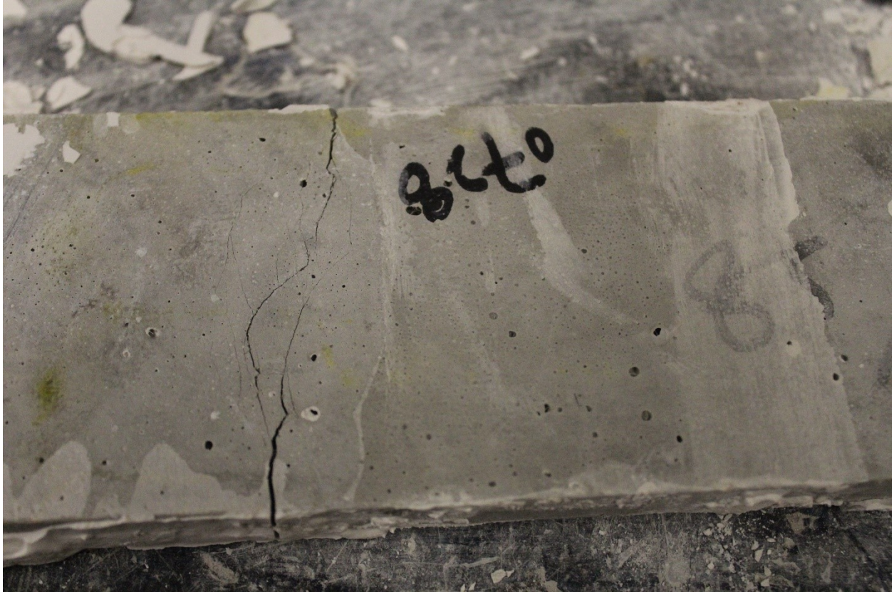
Figure 3-17: Tensile cracking on ECC03 coupon specimen
