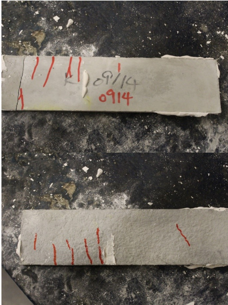
Figure 3-41: Tensile cracking of ECC09 specimen
