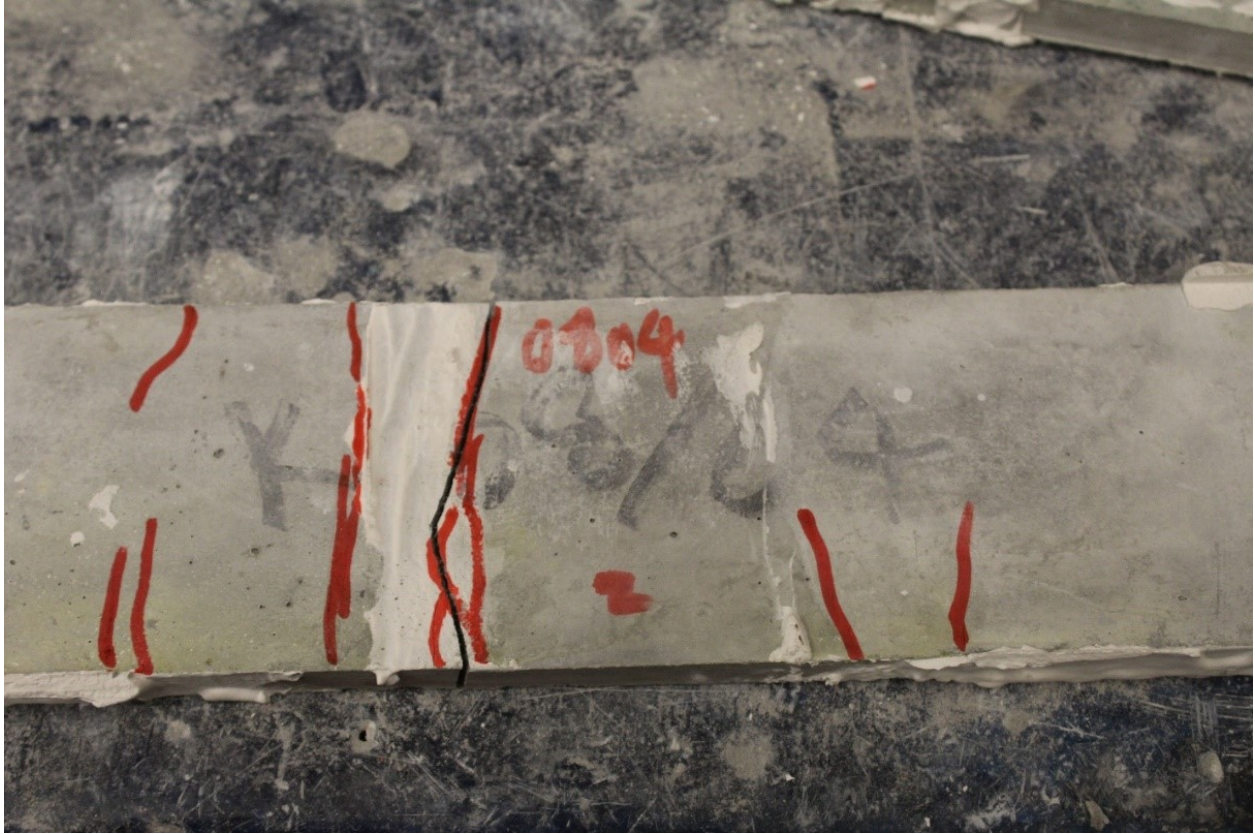
Figure 3-21: Tensile cracking on ECC04 coupon specimen
