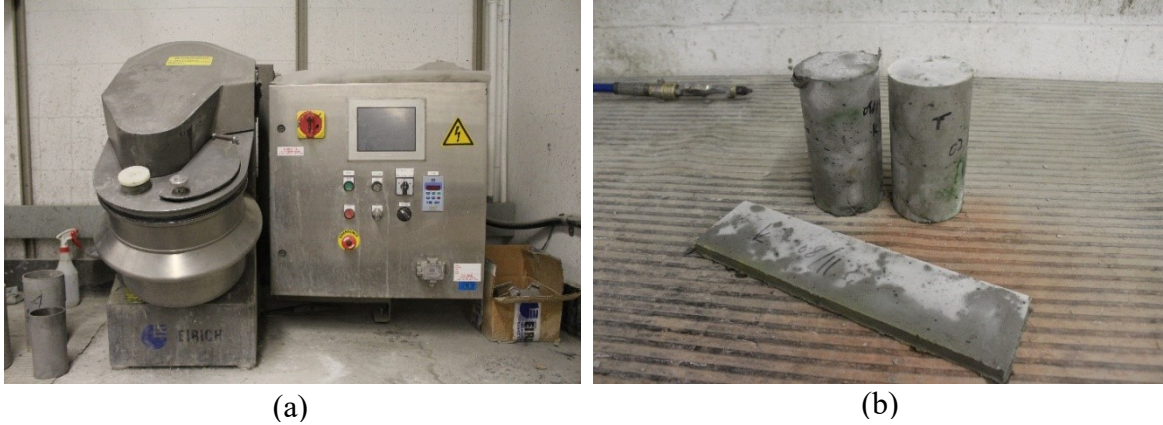
Figure 3-1: (a) ELRICH intensive mixer RV02E, (b) ECC Cylinders and Coupon specimen
