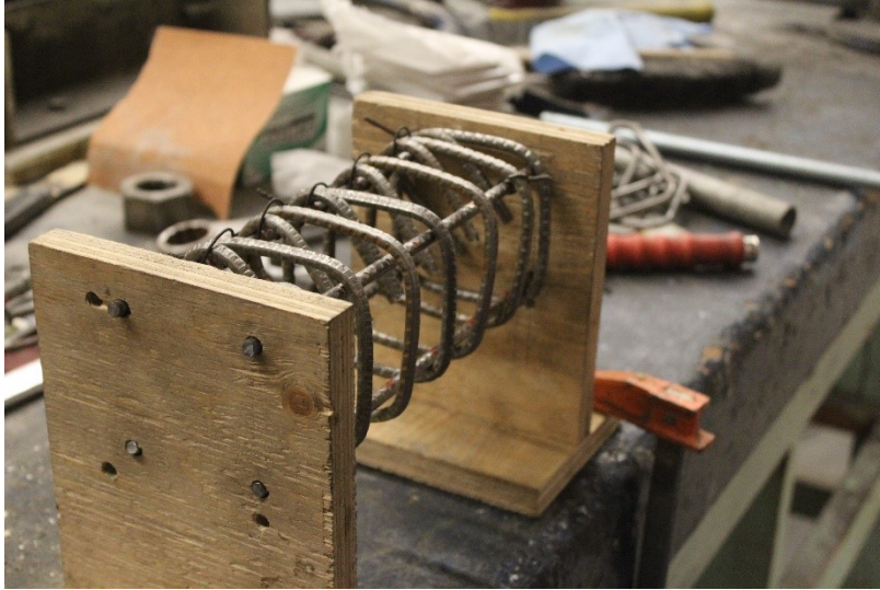
Figure 4-14: Steel cage preparation
