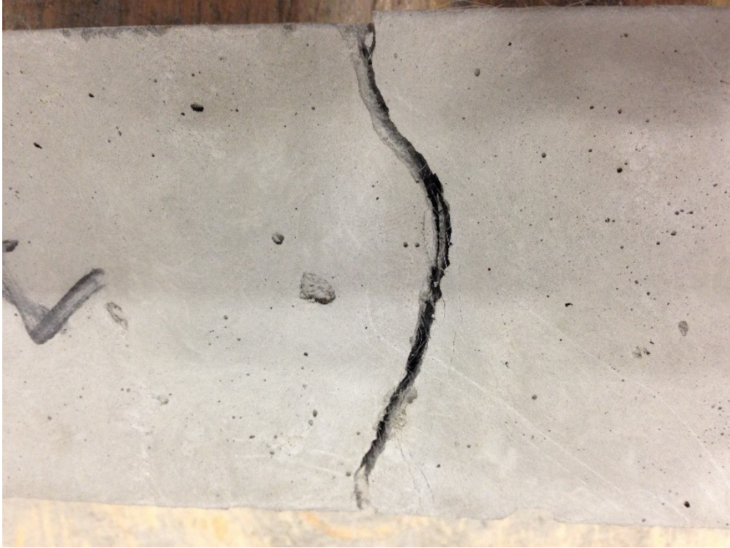
Figure 3-9: Tensile cracking on ECC01 coupon specimen
