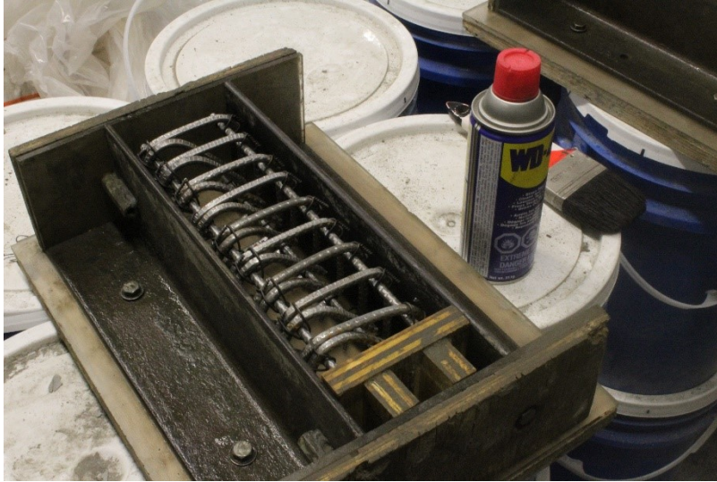
Figure 4-18: Steel cage of ECC-2%
