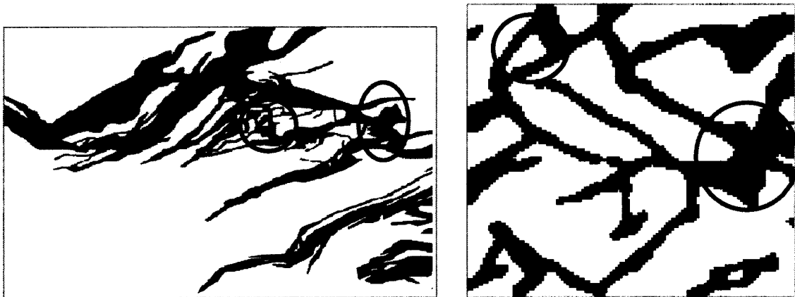
Figure 3-11: Left–Louvicourt Goldfield deposit at Val d’Or in Quebec (Robert and Poulsen, 2001), unknown scale. Right–Rotated TI with a 10:1 aspect ratio and a high cutoff. Highlights–rock pockets surrounded by veins and thickening of the veins.
