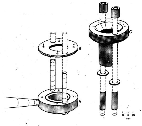
stretcher to provide resistance to the stretcher, and the locking nuts were used to increase the stretch by moving the stretcher downward. A 200 mm long, 12.5 mm diameter brass rod, tapered and threaded at one end to screw into the supportive base, was used to support the stretching apparatus.
