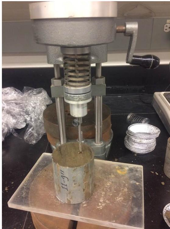
Figure A.7. Vane shear test on undisturbed sample
