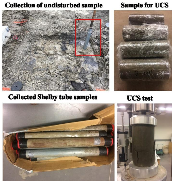
Figure A.2. Soil sample collection, sample preparation and testing
