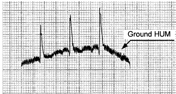
Figure 2-14: Effect of a 60 cycle ground interference on the ECG recordings [60]
