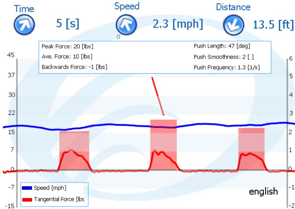
**Figure 2.10:** Computer screen display of the propulsion data (Smartwheel User's Guide 2008).
